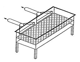
Figure 3 - Slot hood for dip tank
