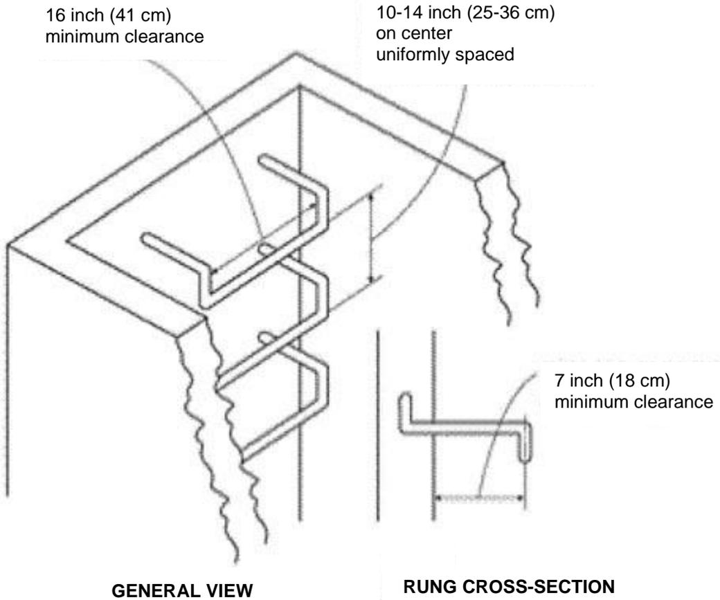
**Figure D-5 -- Fixed Ladder Clearances**
