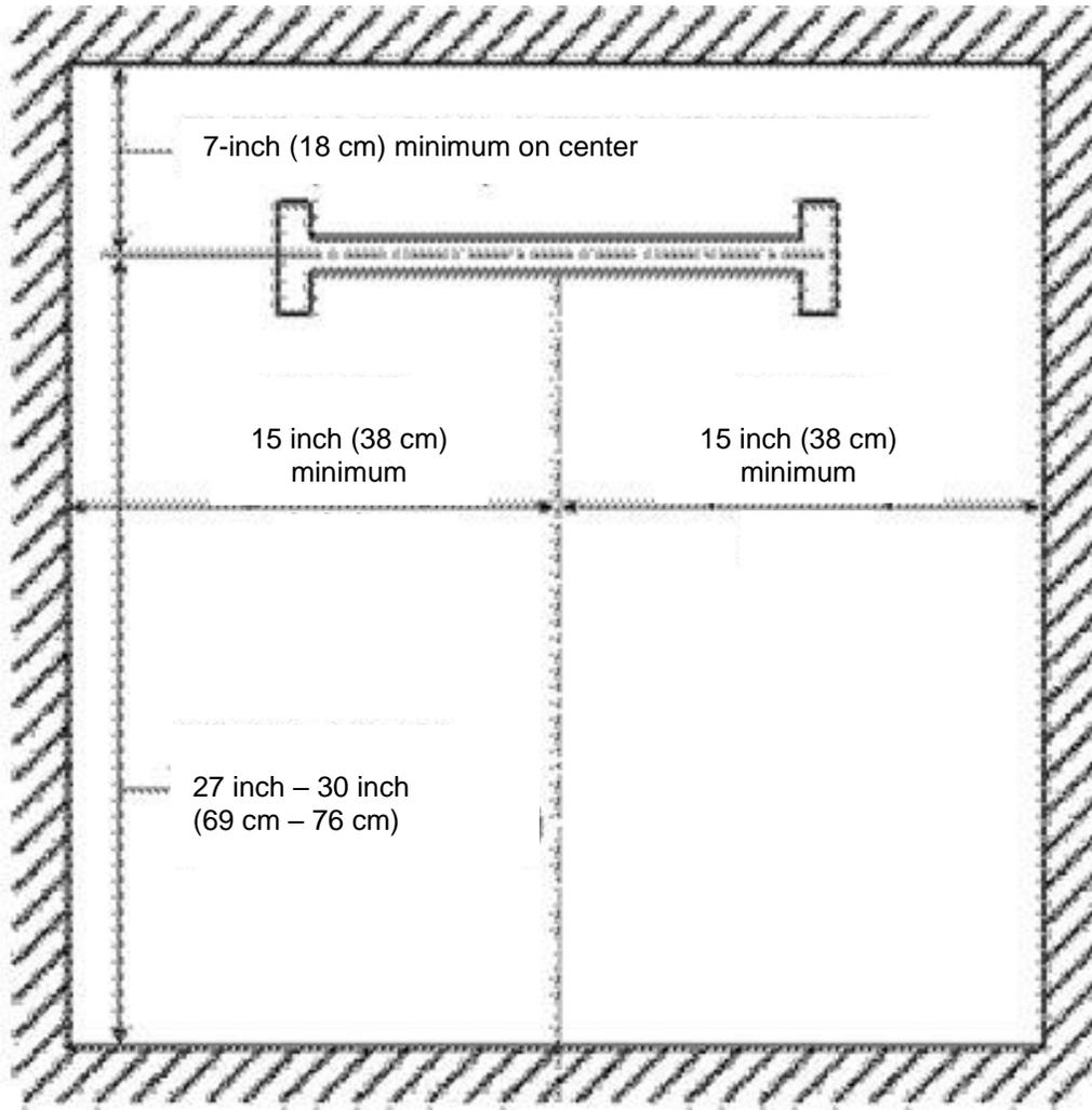
Figure D-15 -- Example of General Construction of Cages
