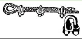
NOTE: There is only one correct method of installing wire rope clips. They should be attached to rope ends as shown in photograph above. The base of each clip should bear against the live, or long rope end, and the U-Bolt should bear against the dead or short rope end.
