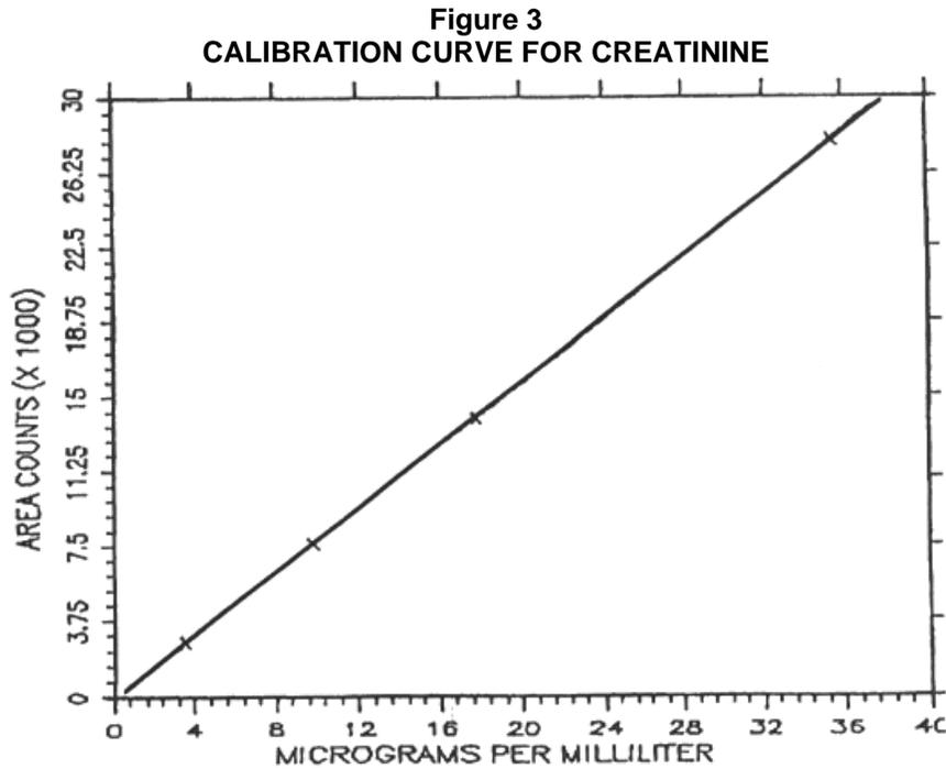
3.7.2. The concentration of creatinine in a sample is determined by finding the concentration corresponding to its detector response. (See Figure #3).
