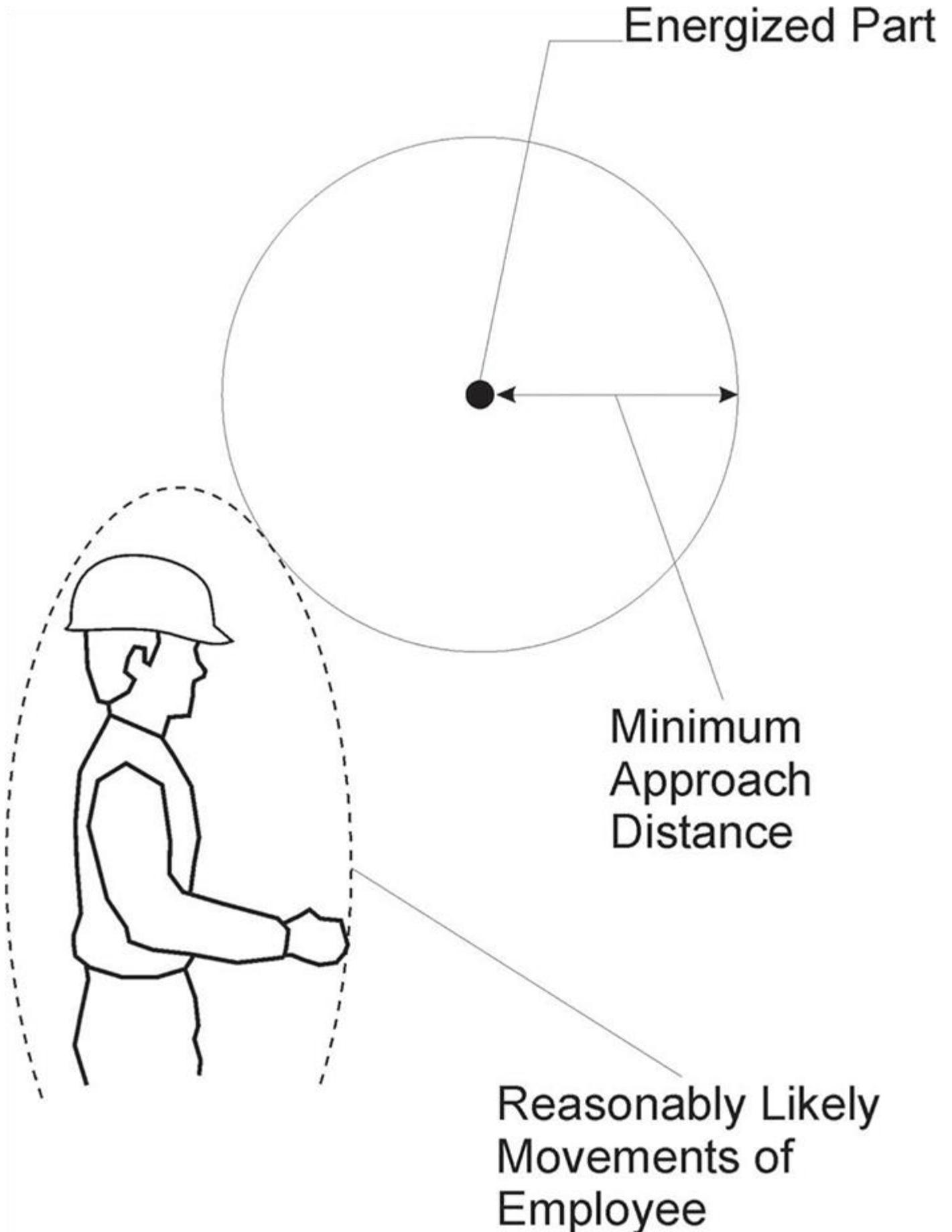
Figure 1 - Maintaining the Minimum Approach Distance
