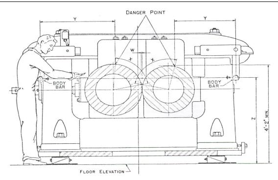
Installation of Pressure-Sensitive Body Bar
