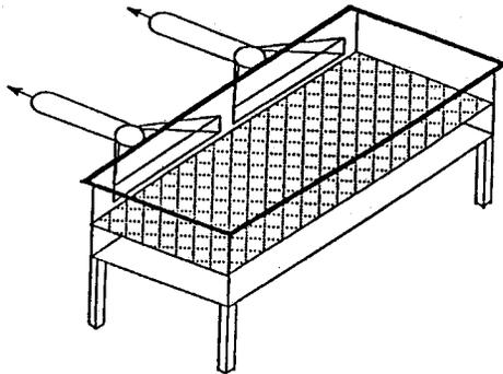
**Figure 3 – Slot hood for dip tank**
