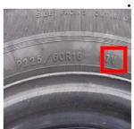
Be certain the tire speed ratings meets or exceeds the speed capability of the vehicle on which the tire is being used.
