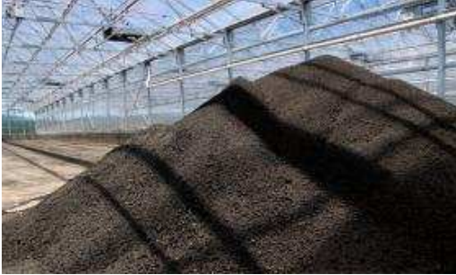
Credit City of Fayetteville Biosolids drying in a greenhouse.
