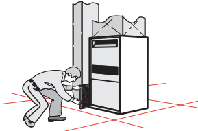
Panel filter installed in filter slot in return plenum
