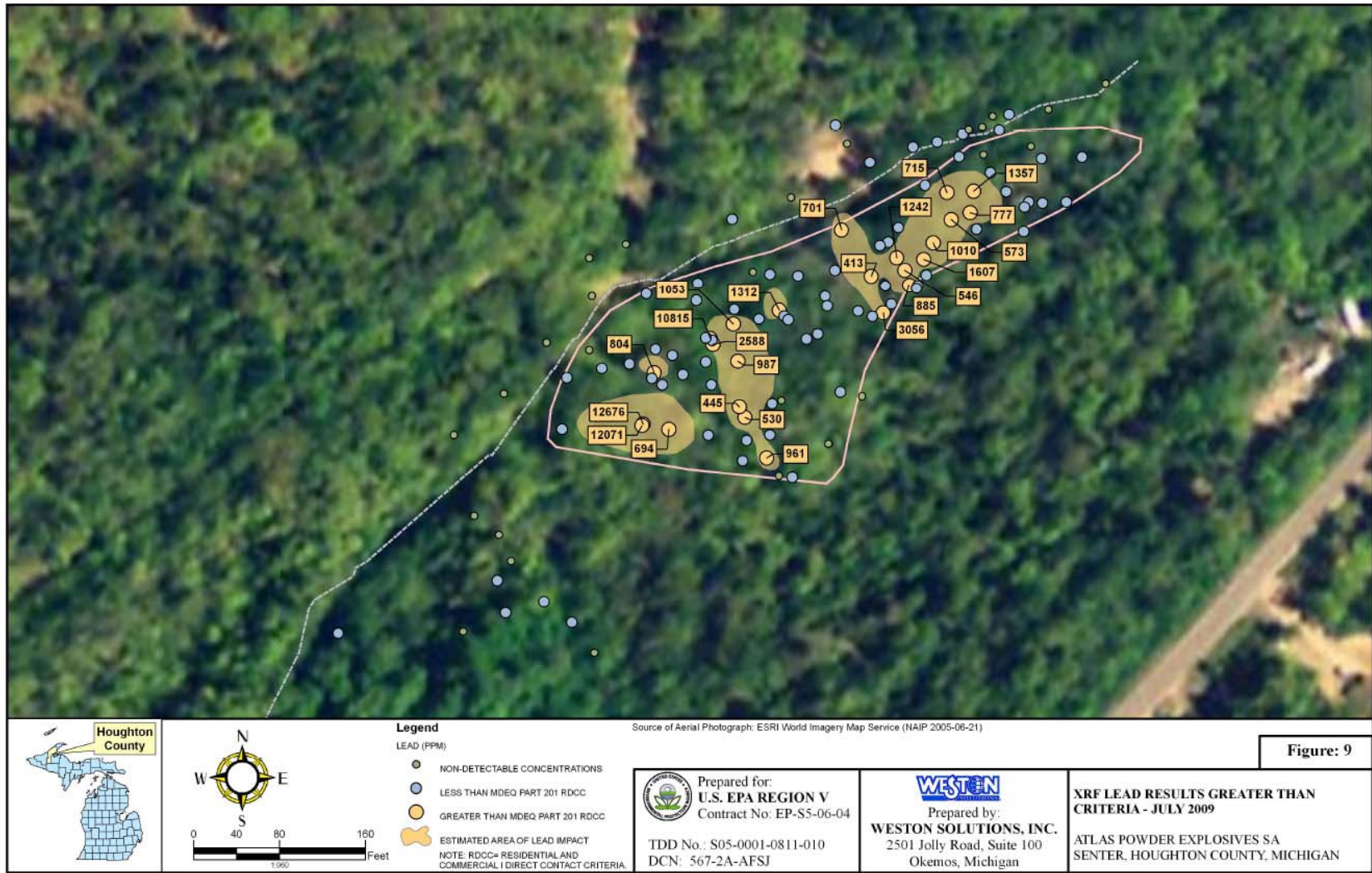
Figure 4. Soil lead concentrations detected during field work conducted in July 2009 at the Atlas Powder dump area, Senter (Houghton County), Michigan. (from Weston 2010)
