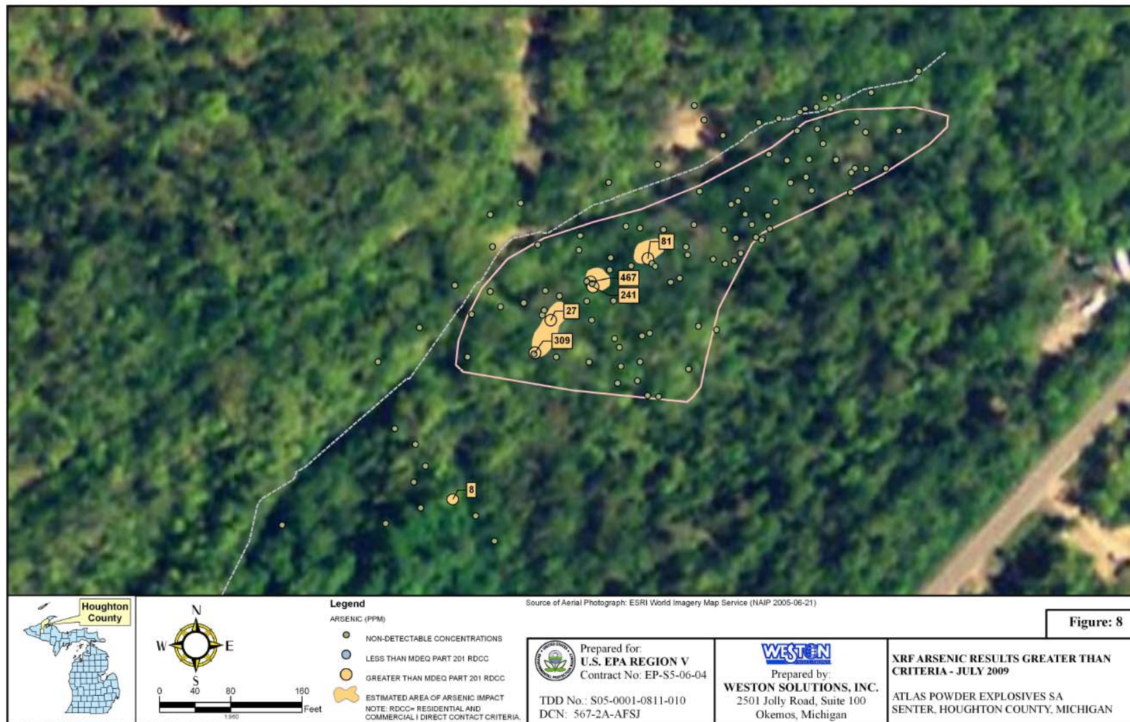
Figure 5. Soil arsenic concentrations detected during field work conducted in July 2009 at the Atlas Powder dump area, Senter (Houghton County), Michigan. (from Weston 2010)
