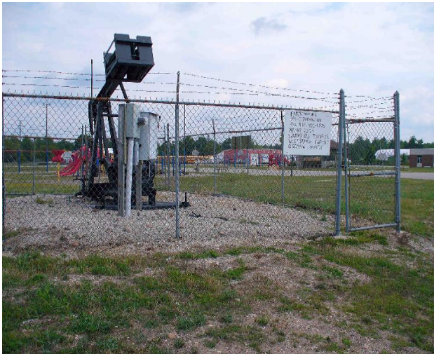
Figure 5: Pumping station for a non-sour gas well near an elementary school in West Branch, Ogemaw County, Michigan.
