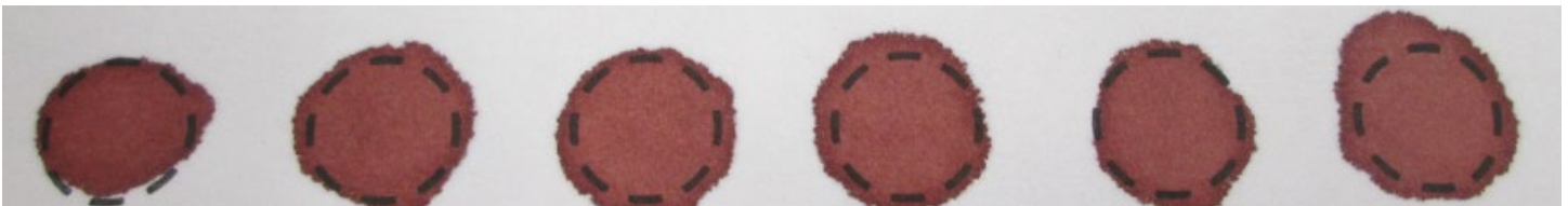
Both the front and back of the specimen card should look like the image above. Note the circles are filled and the even saturation of a single blood drop applied to each circle.
