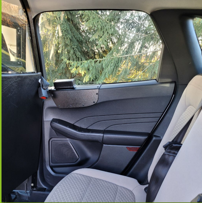
Disabled Controls and Smooth Surfaces
