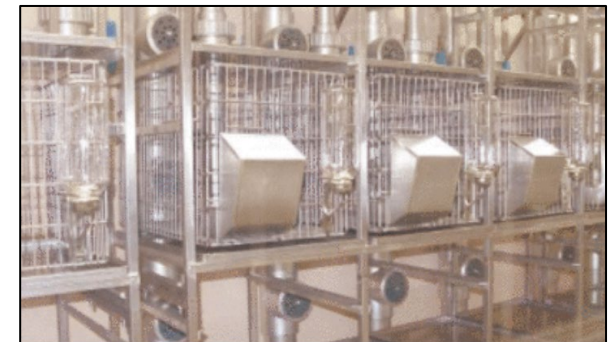
Transmission. Air from a TB ward is vented into guinea-pig cages (above) at an experimental facility in Witbank.
