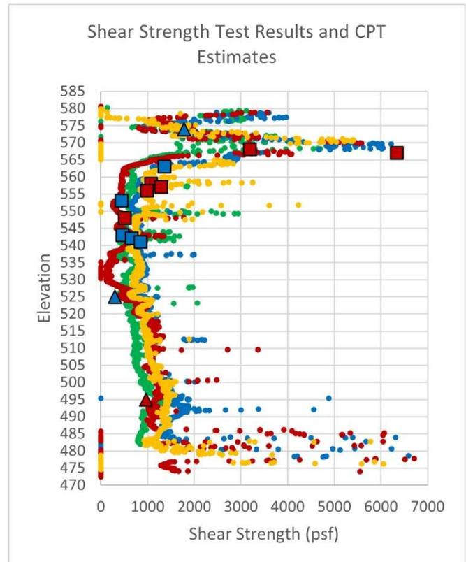
Figure 3: Shear Strength Comparison of Laboratory Tests and CPT Estimates
