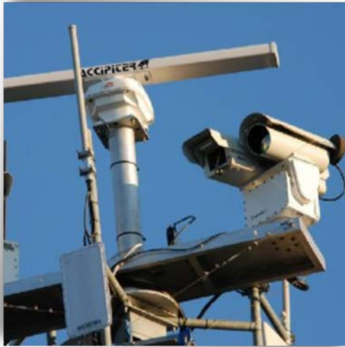
(Above) An Accipiter Radar system like those already housed at the Levin Terminal. New cameras would add visual feed of river for border & law enforcement
