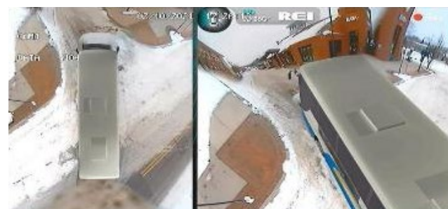
Bay Area Transportation Authority 360-degree detection system
