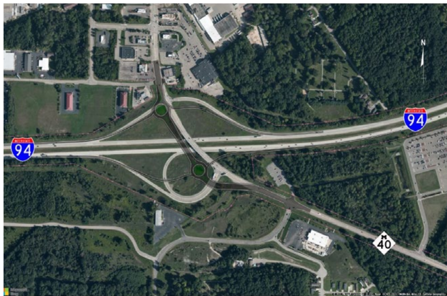
Proposed I-94/M-40 interchange with dual roundabouts (shown as shaded overlay)
