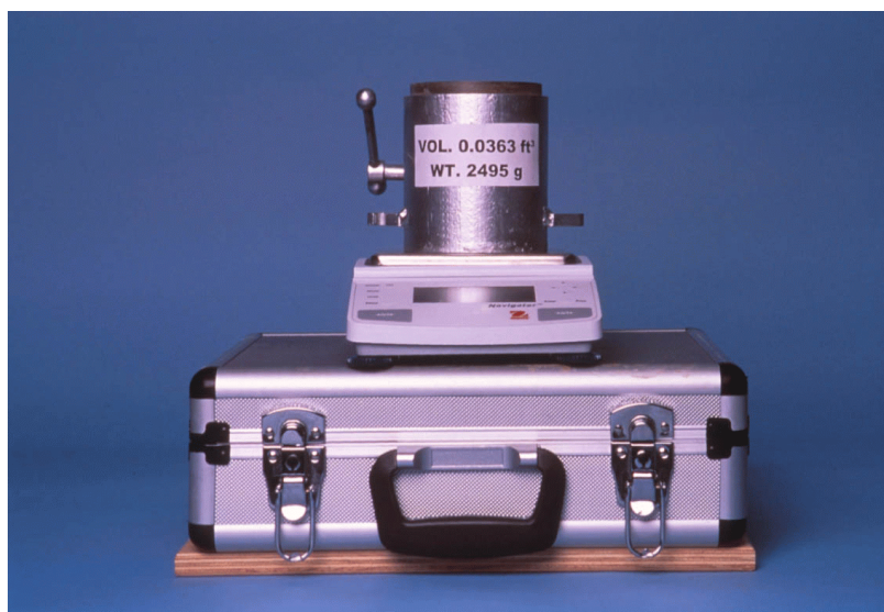
Figure 12. Weighing proctor mold and material on the scale provided in the density box
