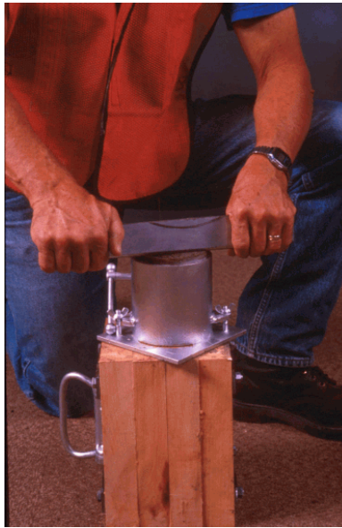
Figure 27. Mold with the material struck-off even with the top of the mold
