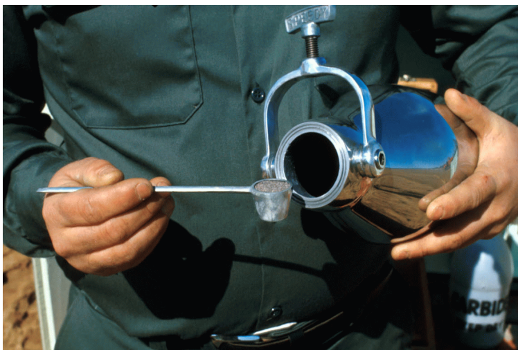
Figure 36. Place calcium carbide in body of the “Speedy”
