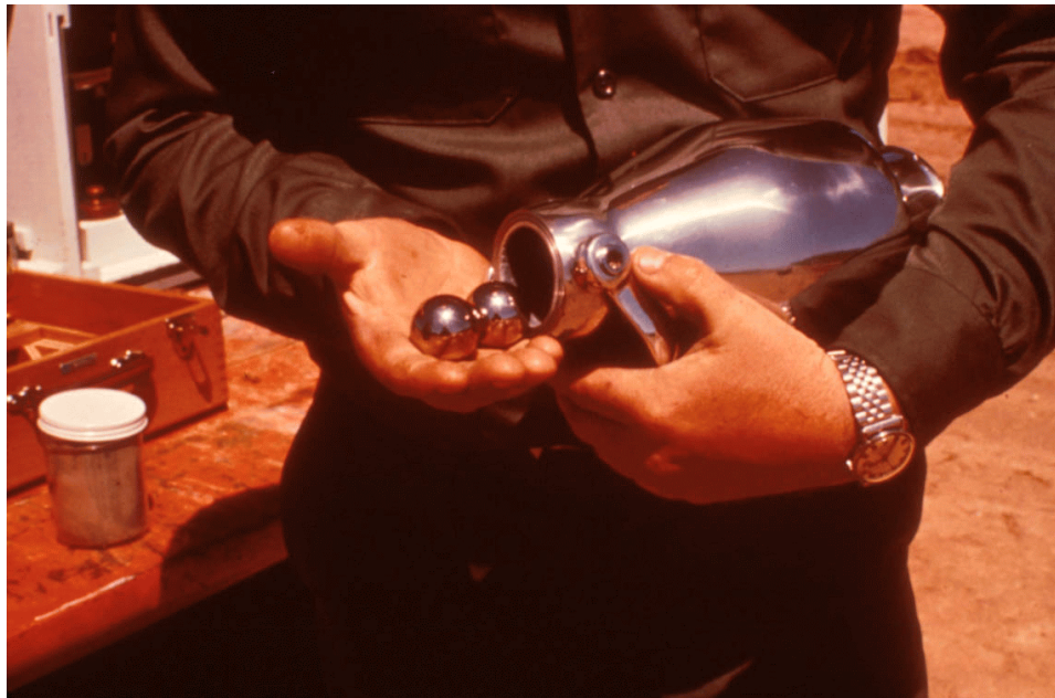
Figure 44. Place steel balls in body of “Speedy” with 3 scoops of calcium carbide
