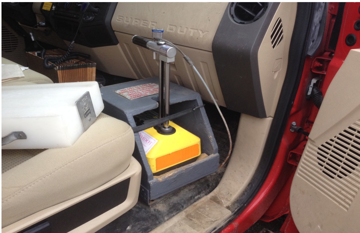
Figure 6a. Troxler nuclear gauge secured in the MDOT Type A box in a cab of a pickup truck.
