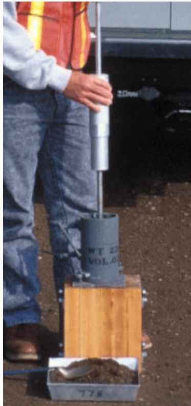
Figure 25. Recycled material being compacted in the mold
