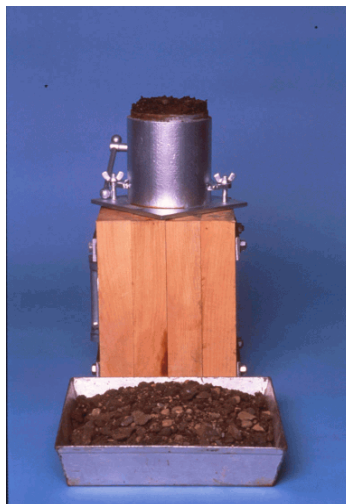
Figure 26. Mold with collar removed and recycled material \frac{1}{4} to \frac{1}{2} inch above the top of mold
