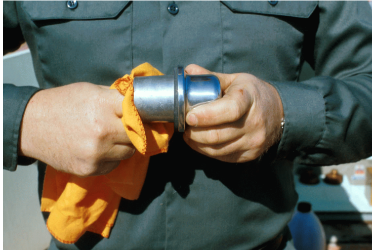
Figure 33. Proper technique for cleaning the cap of the meter
