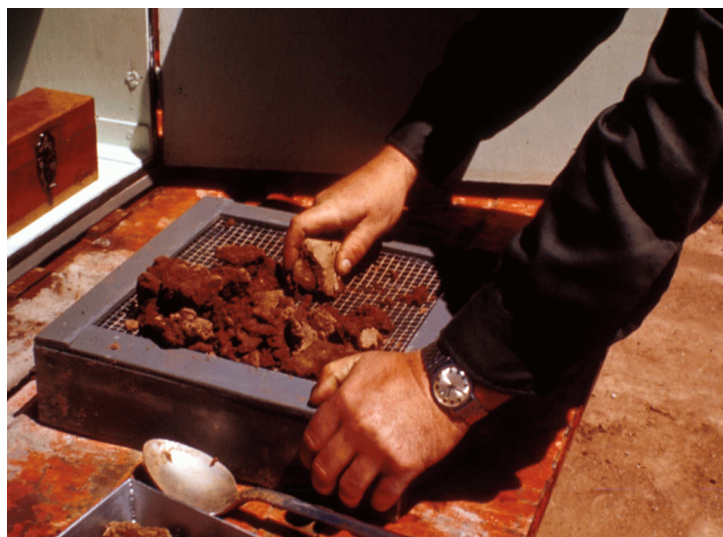
Figure 46. Using the \frac{1}{4} inch screen from the density kit, always screen cohesive soil before obtaining the moisture sample
