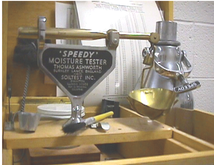
Figure 47. Weigh moisture sample
