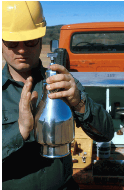
Figure 40. Hold the “Speedy” upright; tap the side of the body
