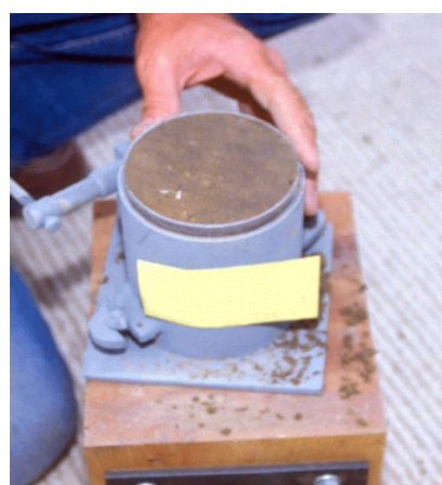
Figure 10. After removing collar, compacted soil extending \frac{1}{4} to \frac{1}{2} inch above the top of mold (top) is removed with strike-off bar (bottom)
