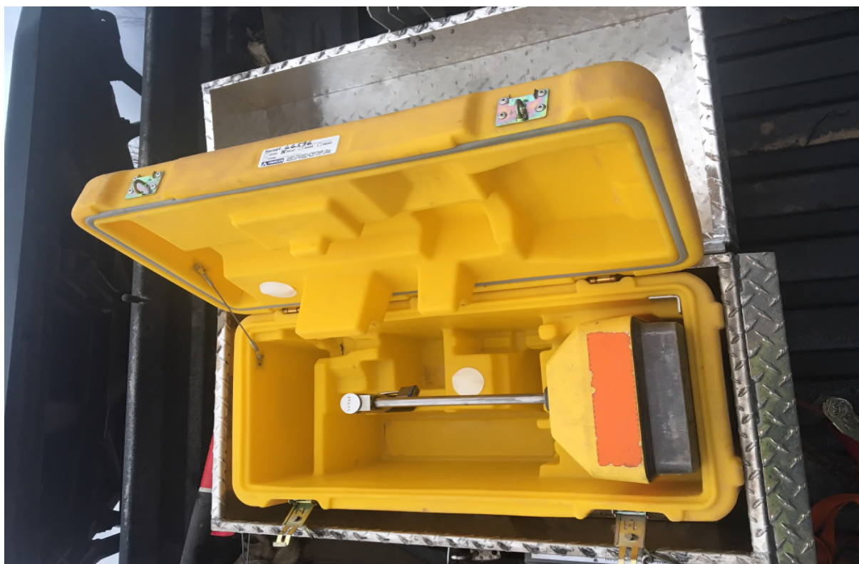
Figure 6b. Troxler nuclear gauge secured in the manufacturer's carrying case housed in the NUX Safety Containment Box.
