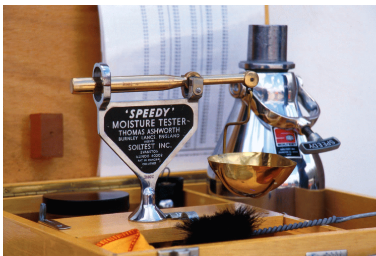
Figure 37. Weigh moisture sample
