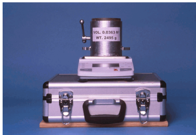
Figure 28. Weighing the mold and recycled material to the nearest gram
