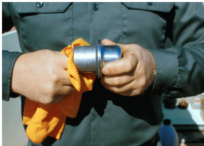
Figure 45. Cleaning the cap of the meter
