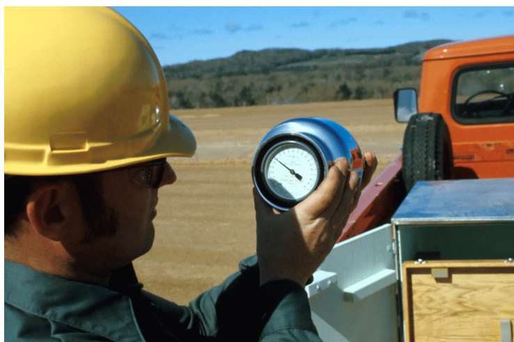
Figure 42. Read dial with “Speedy” held horizontally
