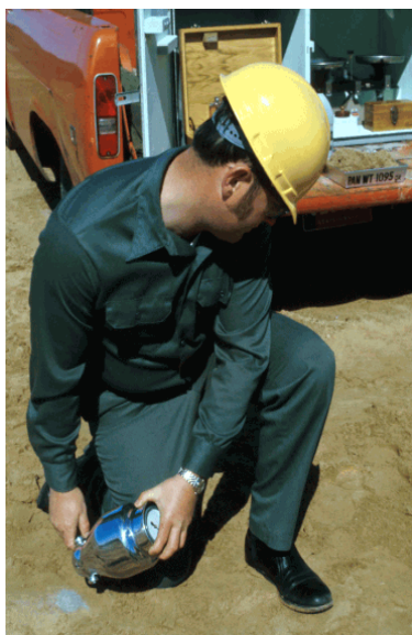
Figure 43. Hold “Speedy” downwind and away from body. Slowly release pressure and empty the “Speedy.”
