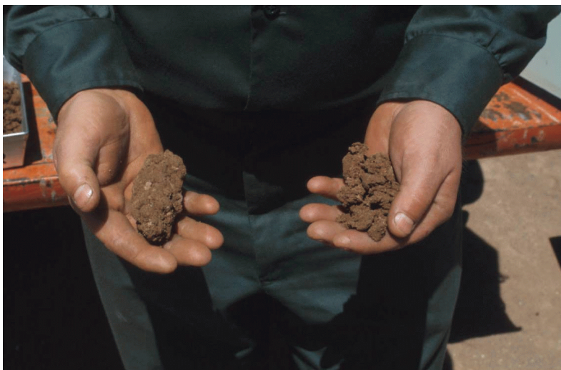
Figure 17. Appearance of soil cast approximately 4.0 percent below Optimum Moisture (left), and easily broken under minimal pressure (right)
