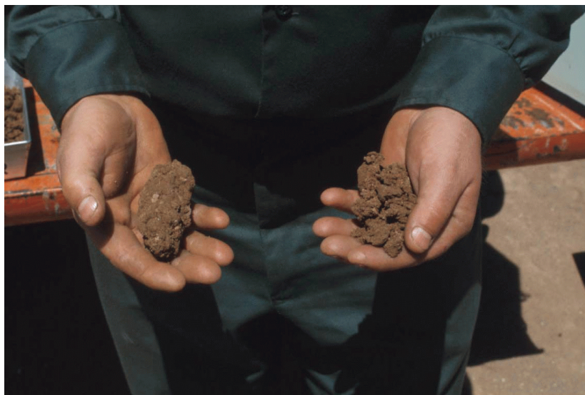
Figure 8. Appearance of the soil cast between 4.0 percent below Optimum Moisture and Optimum Moisture (left), broken up under hand pressure (right)
