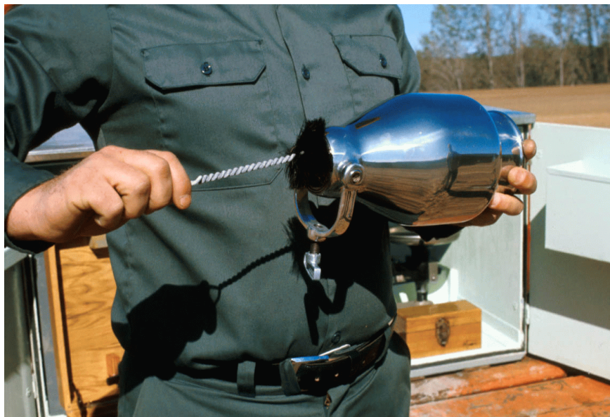
Figure 34. Proper technique for cleaning the body of the meter
