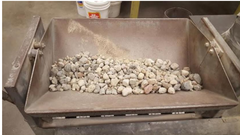
Figure 37: Splitter Filled – Top View
