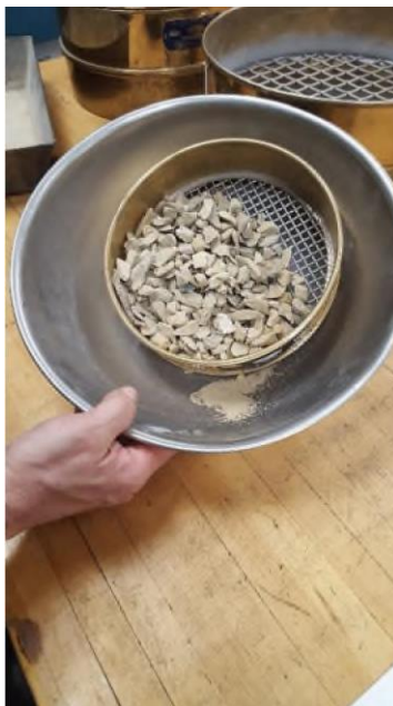
Figure 44: Sieve in bowl for 1 min of hand shaking
