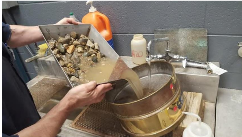
Figure 39: Pour Rinse Water into Stacked Sieves
