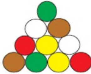
Figure 45: Marble Stacked showing poor interlocking
