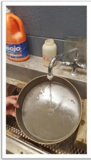
Figures 40: Rinse material to side of the sieve and back into the pan
