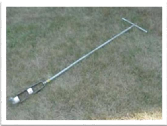
Figure 6: 5-foot T-handle bucket auger made from thick walled galvanized iron pipe with blades welded on either a 3 or 4 inch outside diameter foot long thin walled pipe
