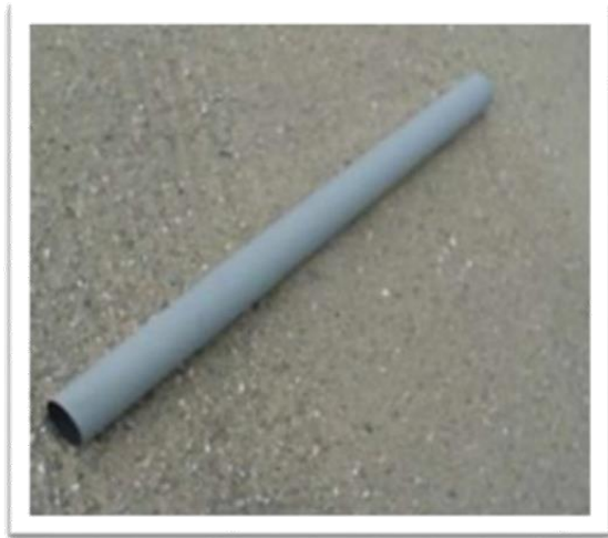
Figure 5: A sample thief made from 1½ to 2 inch diameter by approximately 30 inches long thin wall electrical conduit to sample fine aggregates (sand) only
