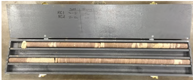
Figure 2: Wood Core Box with Wood Inserts
