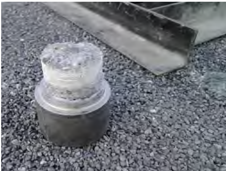
Figure 5.05.09 Thin Overlay Tensile Rupture Test Sample
