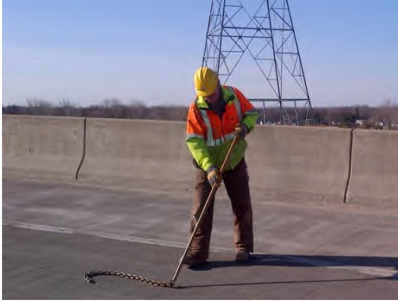
Figure 5.05.08 Sounding Shallow Overlay Using Chain-Drag Method
