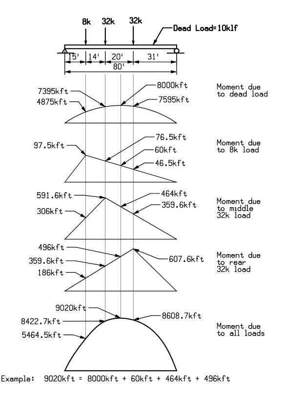
FIGURE 4.2 Example of Superposition
