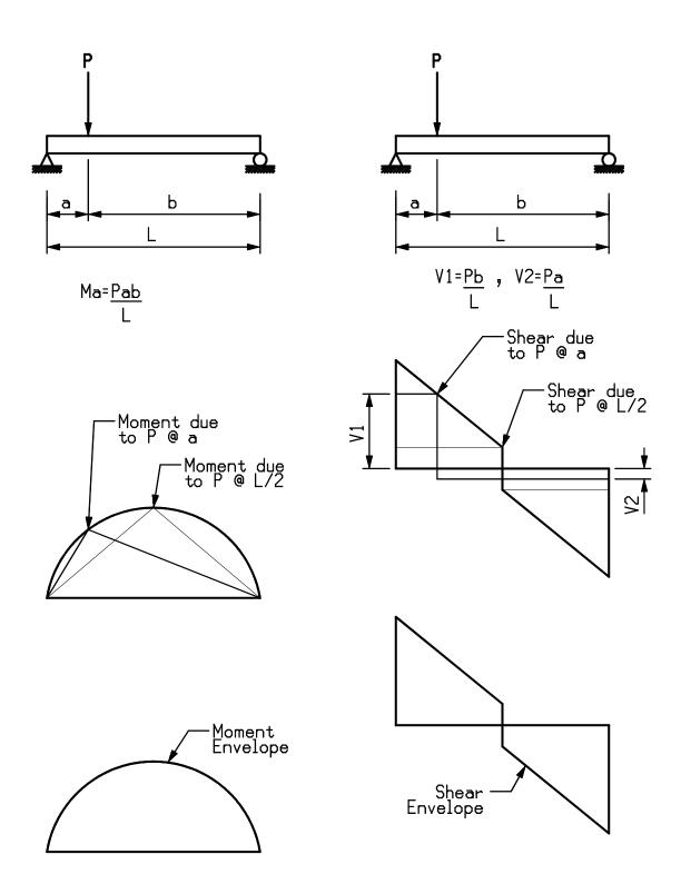
FIGURE 4.4 Example of Moment and Shear Envelopes
