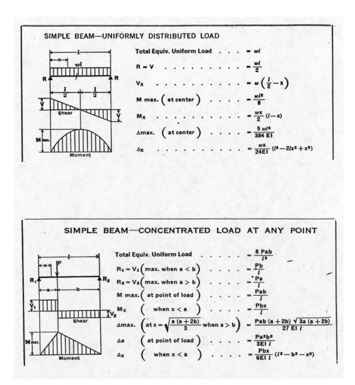
FIGURE 4.1 Common Beam Diagrams
