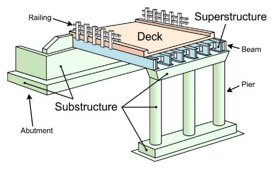
Figure 6: Diagram of basic elements of a bridge
