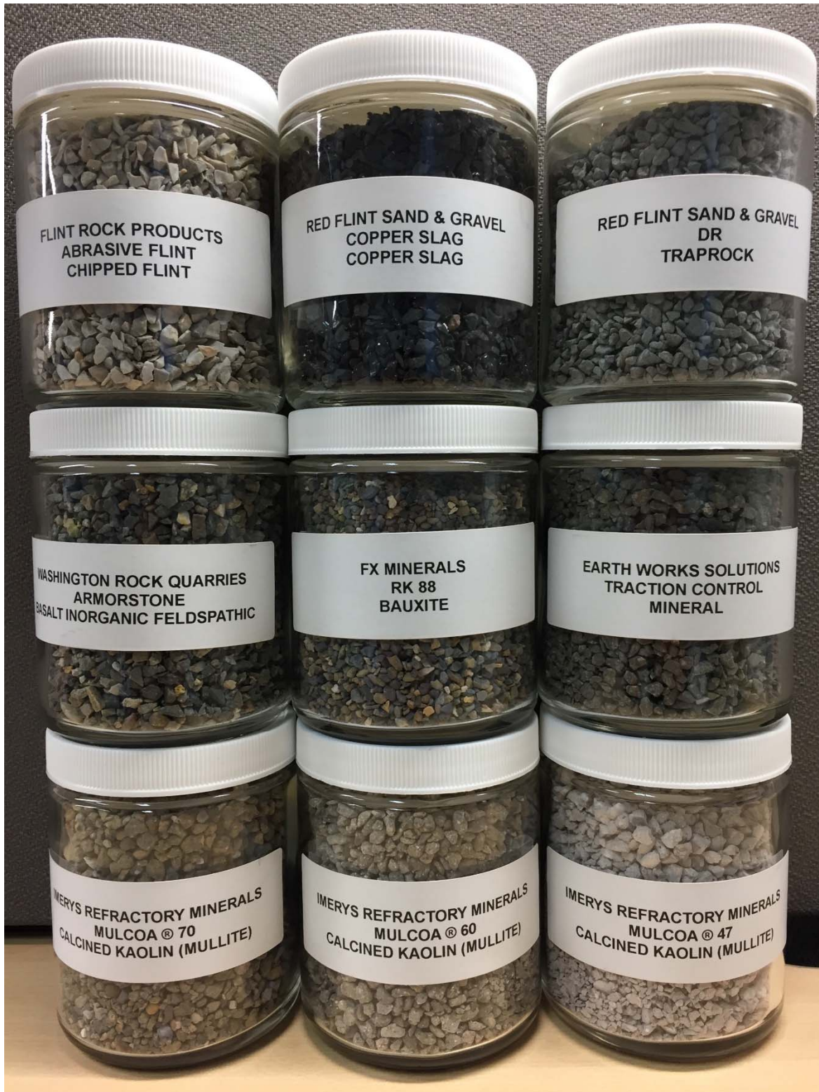
Figure 4 Angular aggregate used for thin epoxy overlays to increase skid resistance.
