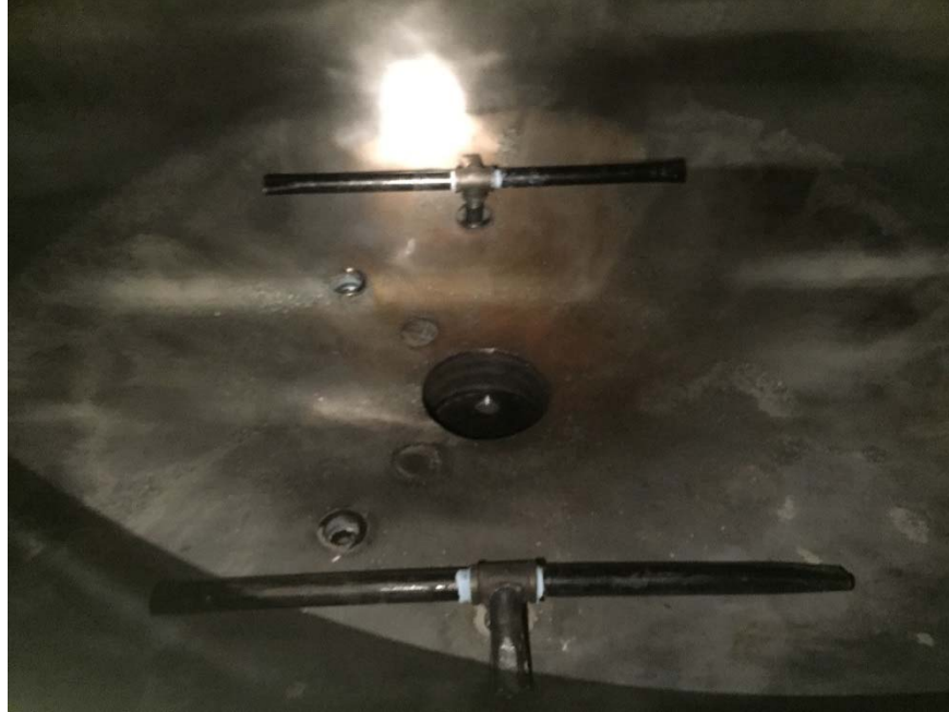
Figure 25 - Interior view of the bottom of the blast pot showing air manifold used to push aggregate towards middle/center dispensing lines.
