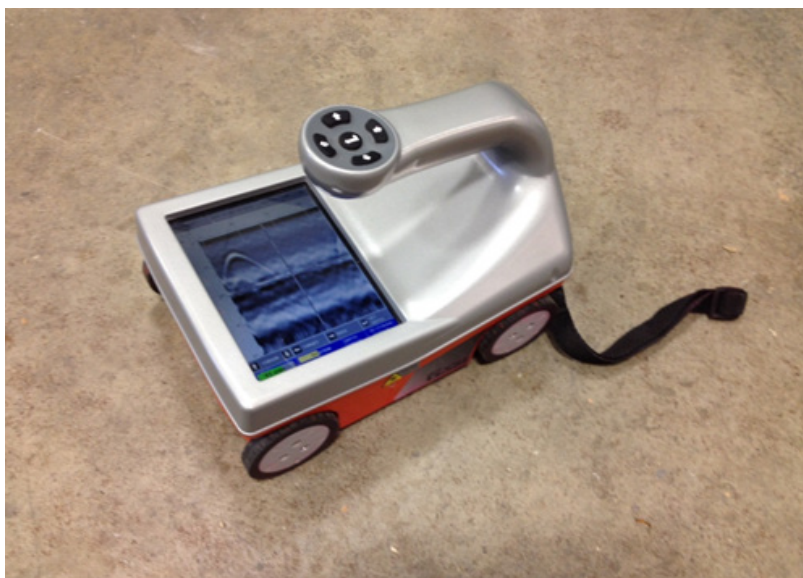
Figure 15. GPR used for locating bar reinforcement.
