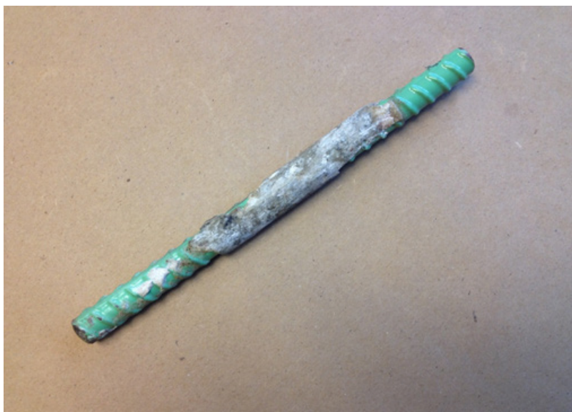
Figure 9. Anchor depicting adhesive bond failure.
