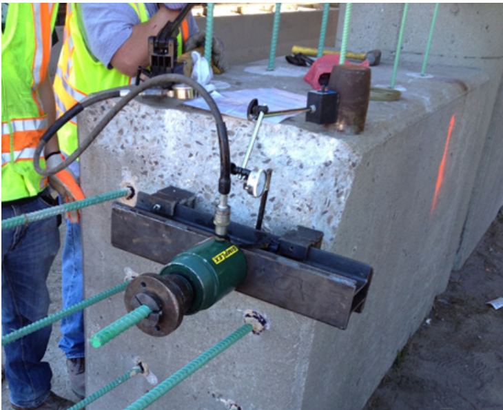
Figure 24. Proof testing in the field on a horizontal anchor.
