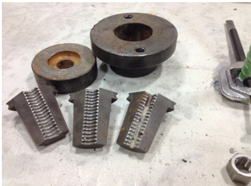
Figure 19. Set of jaws for testing rebar.
