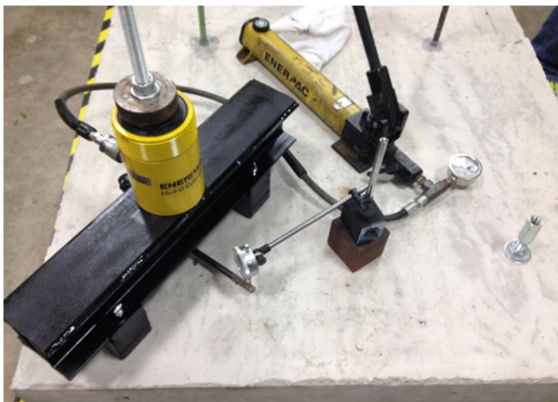
Figure 25. Test Setup for Mechanical Anchor.
