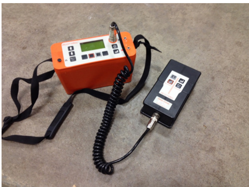
Figure 14. Pachometer used for locating bar reinforcement.
