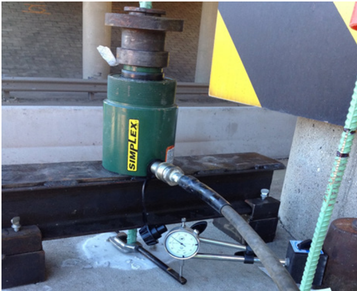
Figure 23. Proof testing in the field on a vertical anchor.
