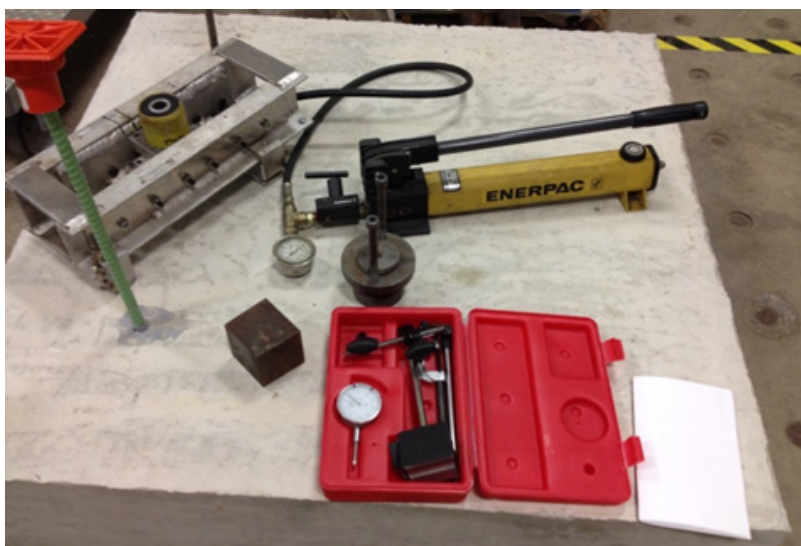
Figure 16. Unconfined tension testing device with complete testing kit.
