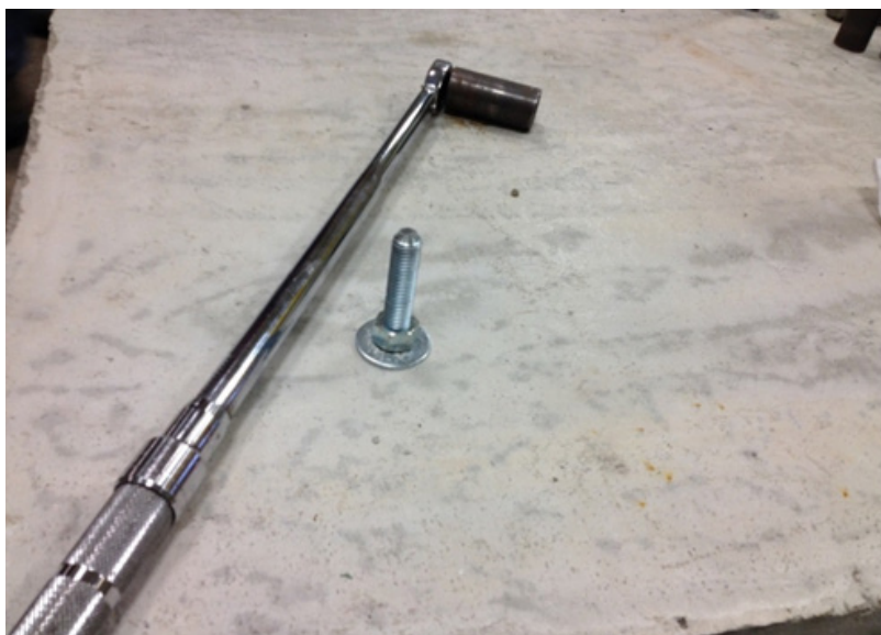
Figure 26. Tension anchor with a torque wrench.
