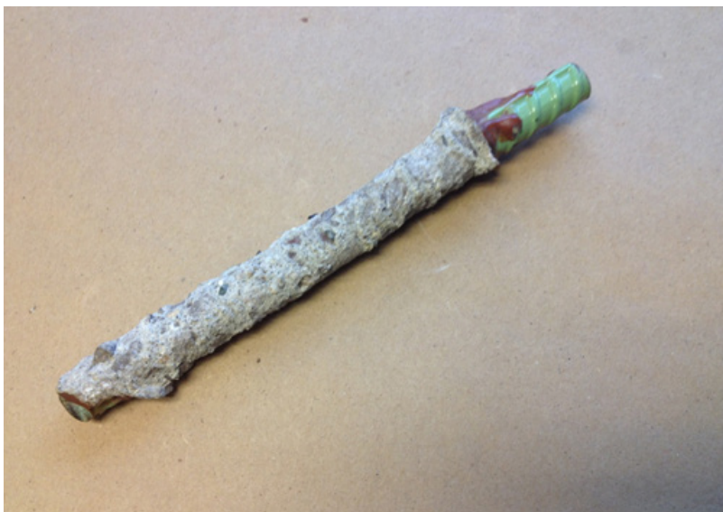
Figure 10. Anchor depicting concrete conical failure (excess concrete removed).
