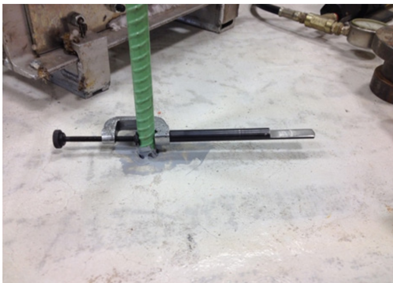
Figure 17. Clamp for measuring displacement.
