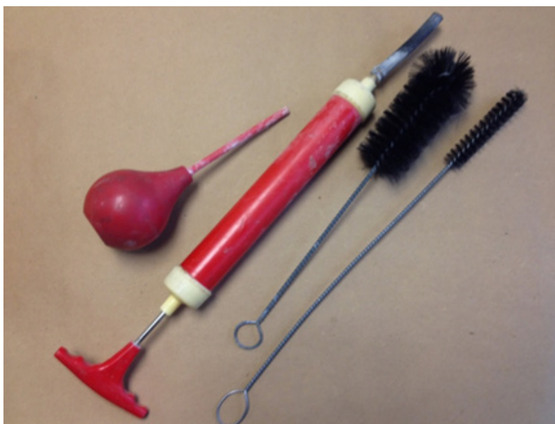
Figure 13. Brushes and air used for cleaning holes.
