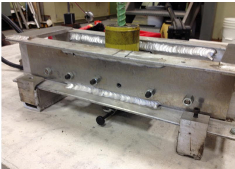
Figure 18. Load Frame for testing rebar.
