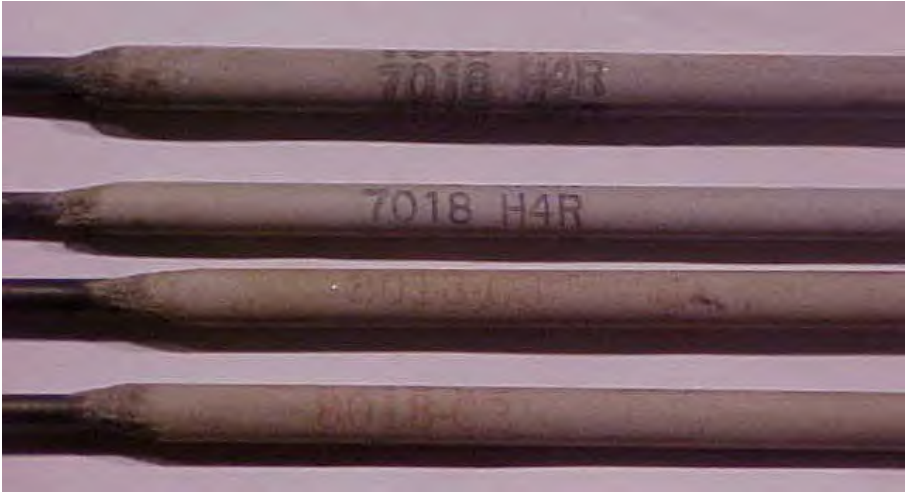
Figure 8. E7018 SMAW 1/8-inch (common size) electrodes.
