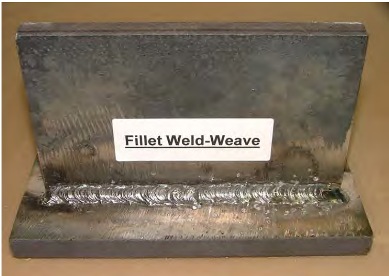
Figure 20. Fillet weld using weave bead.
