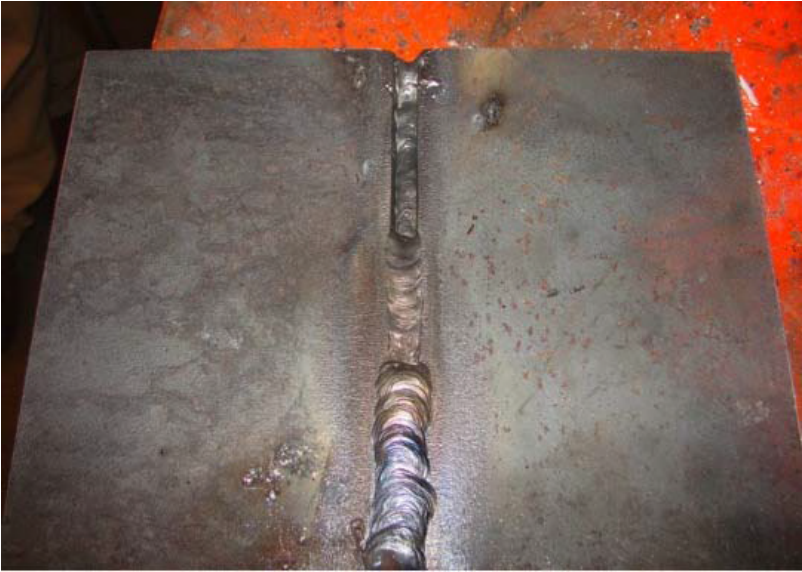
Figure 23. Groove weld showing progression of passes.
