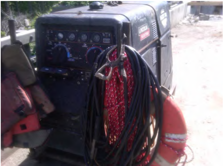
Figure 5. SMAW electric arc welding machine.
