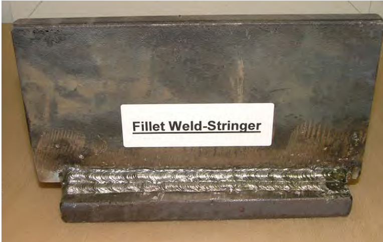
Figure 19. Fillet weld using stringer beads.
