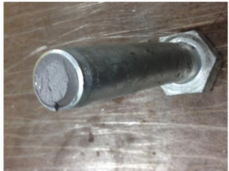
(a) Torsional Failure
