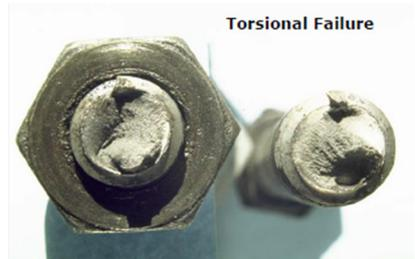
Figure 17: Failure modes to look for after rotational capacity test.
