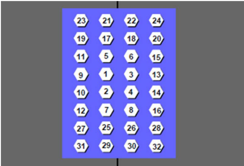
Figure 19: Typical installation pattern for high strength bolts.
