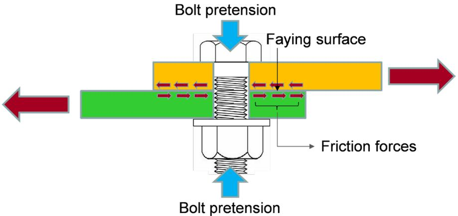
Figure 4: Load transmission in a slip critical-type connection (bolt pretension prevents slip into bearing for service loads).
