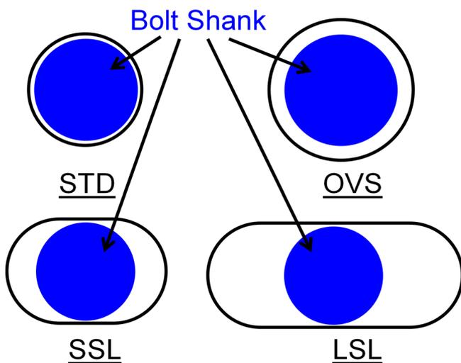
Figure 8: Bolt hole types.
