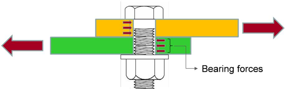
Figure 3: Load transmission in a bearing-type connection.
