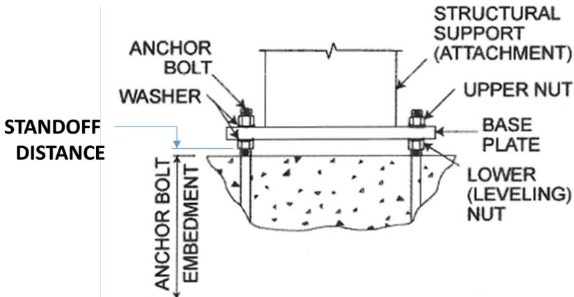
Figure 23: Typical double-nut AB connection.
