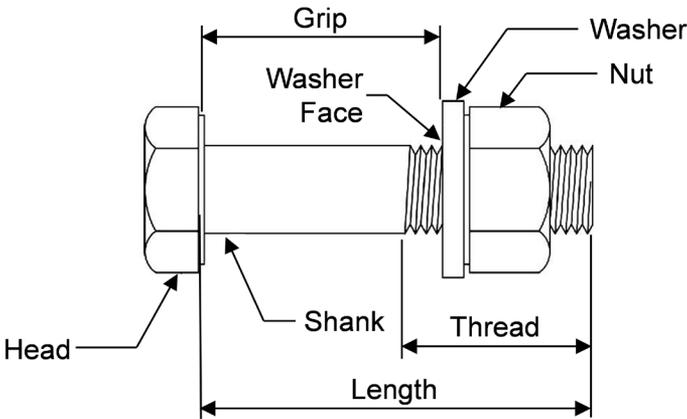
Figure 2: HSB assembly components.
