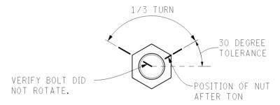
Figure 11: Example TON pre-tensioning match marking procedures.
