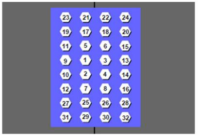
Figure 19: Typical installation pattern for high strength bolts.
