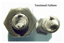
Figure 17: Failure modes to look for after rotational capacity test.
