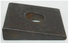
Figure 6: Flat circular washers. Figure 7: Beveled washers. For pre-tensioned joints, ASTM F3125 Grade A325 bolts require a washer under the element (head or nut) being turned to tighten the bolt. For pre-tensioned joints with specified base metal yield strength less than 40ksi, ASTM F3125 Grade A490 and F2280 bolts require a washer under both the head and nut to prevent base metal yielding.
