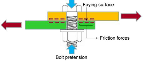
Figure 4: Load transmission in a slip critical-type connection (bolt pretension prevents slip into bearing for service loads).
