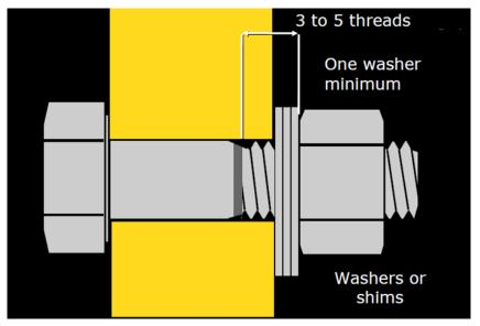
Figure 15: Bolt configuration for rotational capacity test.
