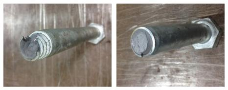
(a) Torsional Failure(b) Tension FailureFigure 18: Bolt failure in torsion versus tension.
