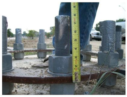
Figure 26: Damaged anchor bolt threads.
