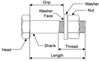
Figure 2: HSB assembly components.
