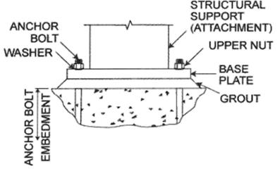
Figure 22: Typical single-nut AB connection (not permitted by MDOT).
