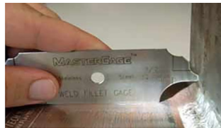
Fillet Weld Gauge (verifying weld size)
