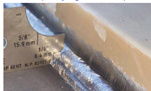
Fillet Weld Gauge (verifying weld is not concave)
