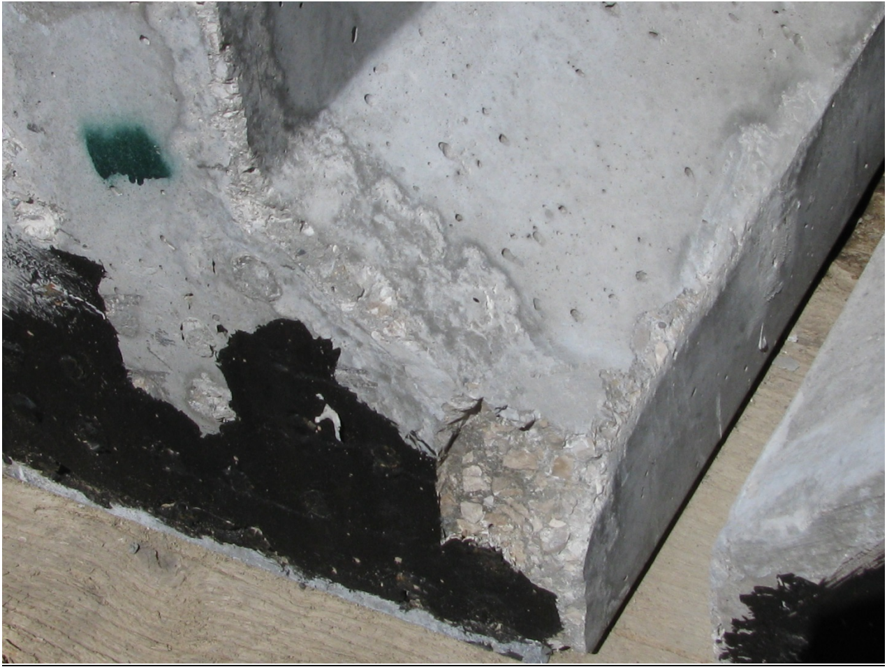
Figure 5. Broken corner at end of PCI beam.
