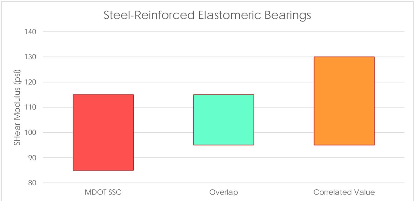
Figure 1. Chart depicting steel-reinforced elastomer shear modulus overlap between as-designed bearing (MDOT SSC) and material provided based on hardness (Shore A 50 durometer) testing (correlated value).
