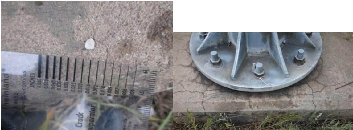
Figure 8.4.5: Truss or cantilever structure foundation, minor cracking measured with a crack comparator (left), significant cracking (right)
