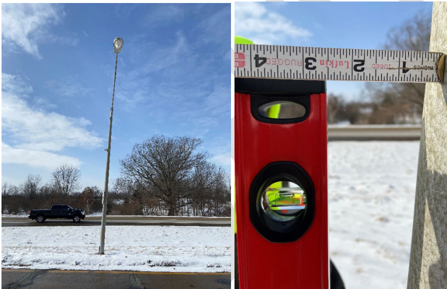
Figure 8.11.20: Non-frangible pole structure vertical support column (upright), visual identification of out of plumb pole (left), measurement of pole plumbness (right)
