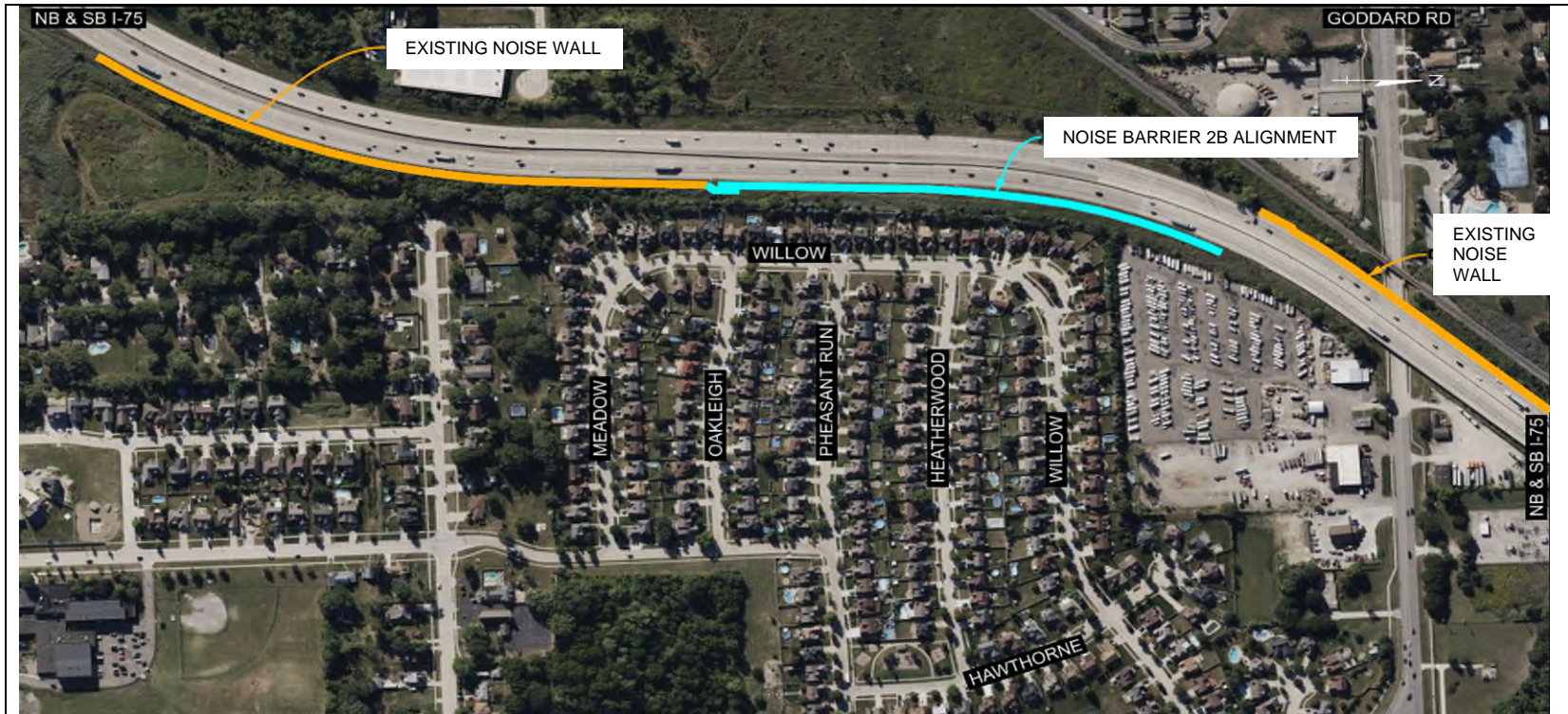
Figure 2: Noise Barrier 2B Alignment
