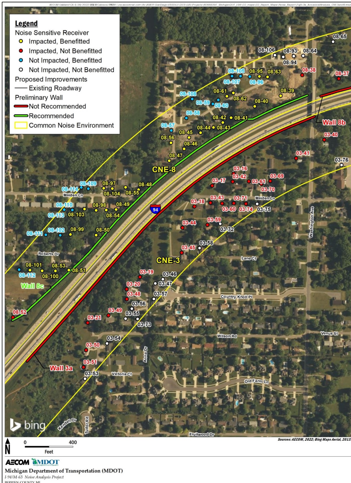
Figure 5-3A Acoustical Analysis for CNE-3, and CNE-8 (Detail Sheet 1 of 2)
