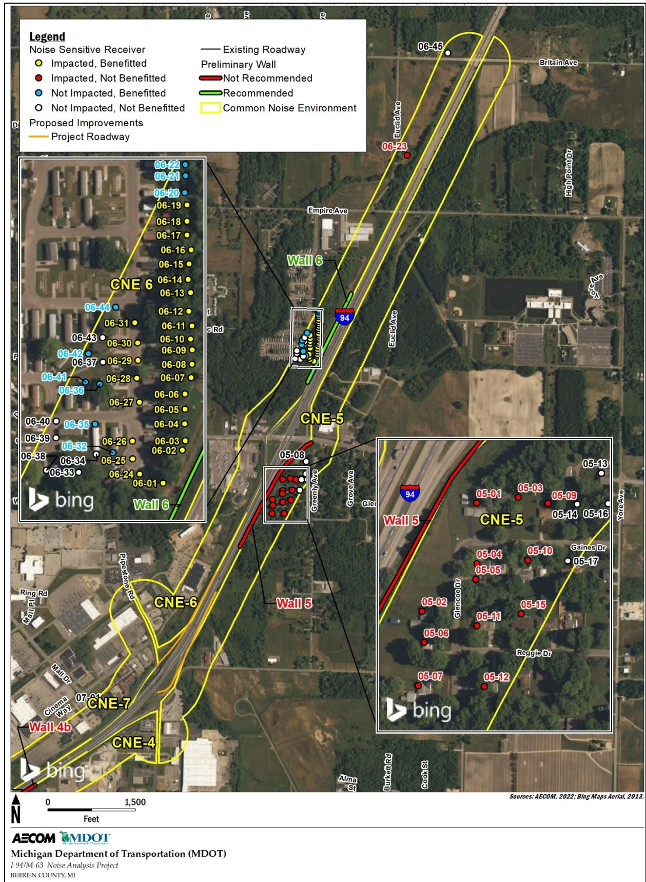
Figure 5-5 Acoustical Analysis for CNE-5 and CNE-6
