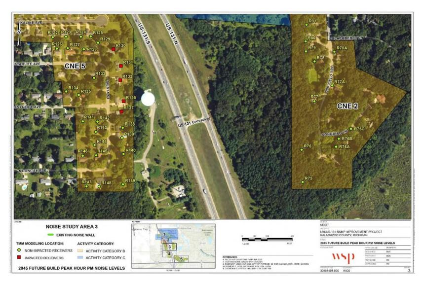
Figure 5C – Peak-Hour PM 2045 Build Noise Level Estimates With Existing Noise Walls
