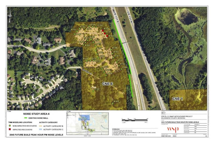
Figure 5D – Peak-Hour PM 2045 Build Noise Level Estimates With Existing Noise Walls
