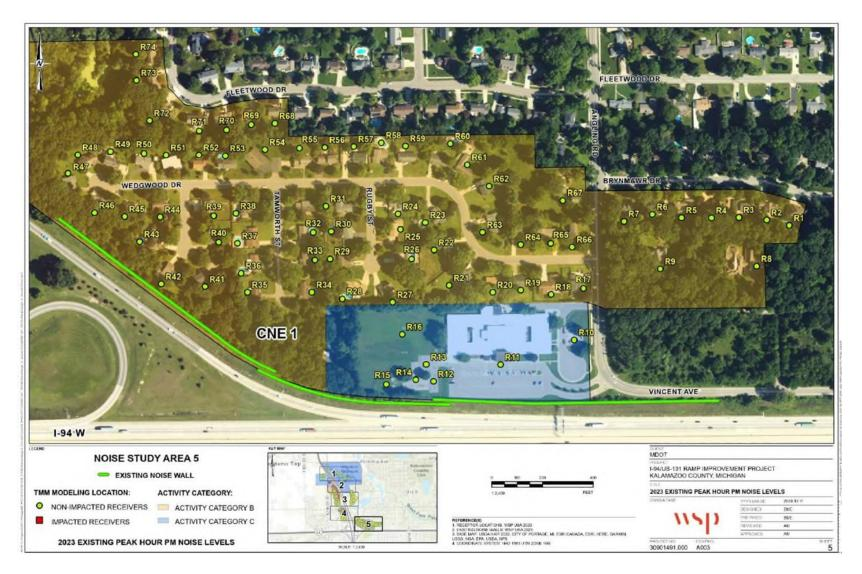
Figure 4F – Peak-Hour PM 2023 Existing Noise Level Estimates With Existing Noise Walls
