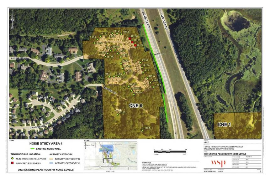
Figure 4E – Peak-Hour PM 2023 Existing Noise Level Estimates With Existing Noise Walls
