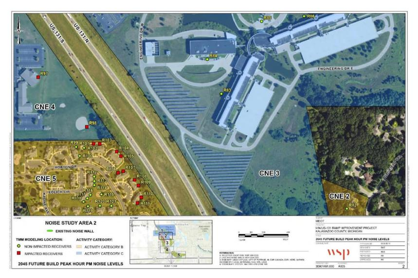
Figure 5B – Peak-Hour PM 2045 Build Noise Level Estimates With Existing Noise Walls
