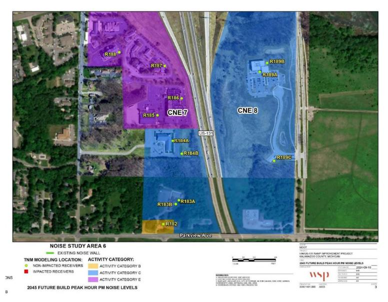
Figure 5F – Peak-Hour PM 2045 Build Noise Level Estimates With Existing Noise Walls
