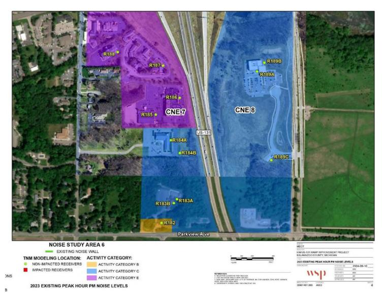
Figure 4G – Peak-Hour PM 2023 Existing Noise Level Estimates With Existing Noise Walls
