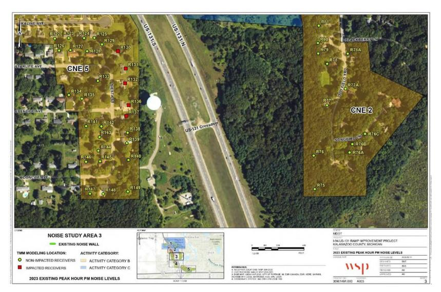
Figure 4D – Peak-Hour PM 2023 Existing Noise Level Estimates With Existing Noise Walls
