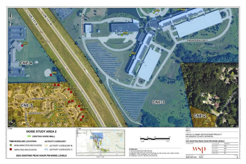
Figure 4C – Peak-Hour PM 2023 Existing Noise Level Estimates With Existing Noise Walls
