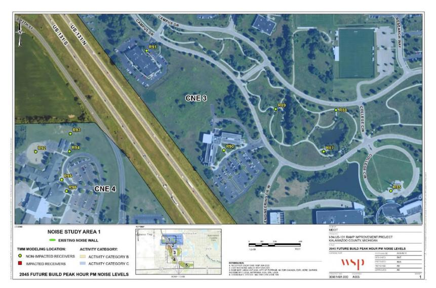
Figure 5A – Peak-Hour PM 2045 Build Noise Level Estimates With Existing Noise Walls
