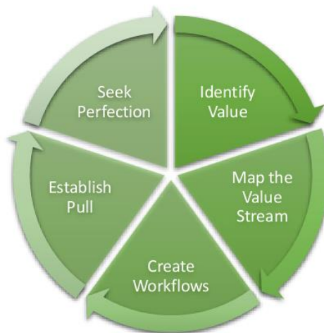
Figure 31. The five principles of a lean process.
