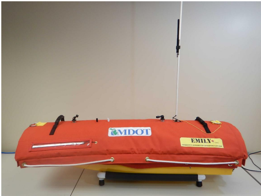
Figure 6: Sonar EMILY with float and antenna installed
