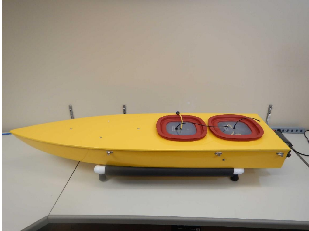
Figure 3: Sonar EMILY without Floatation Device
