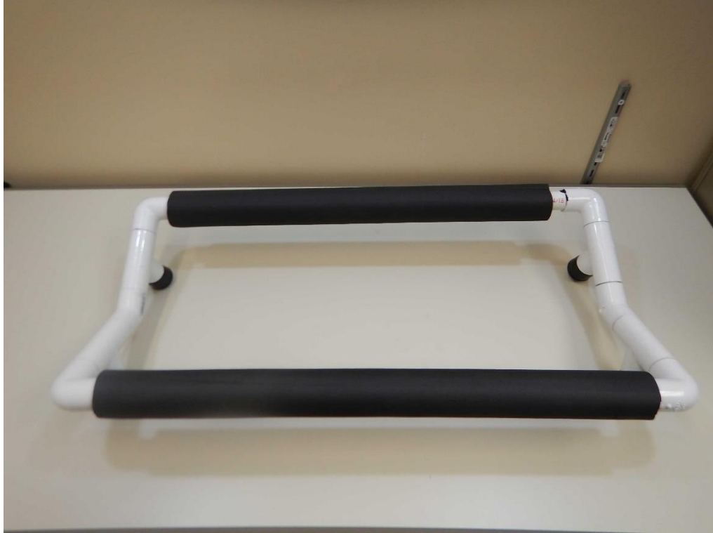
Figure 1: Travel Stand Boat Resting Skids
