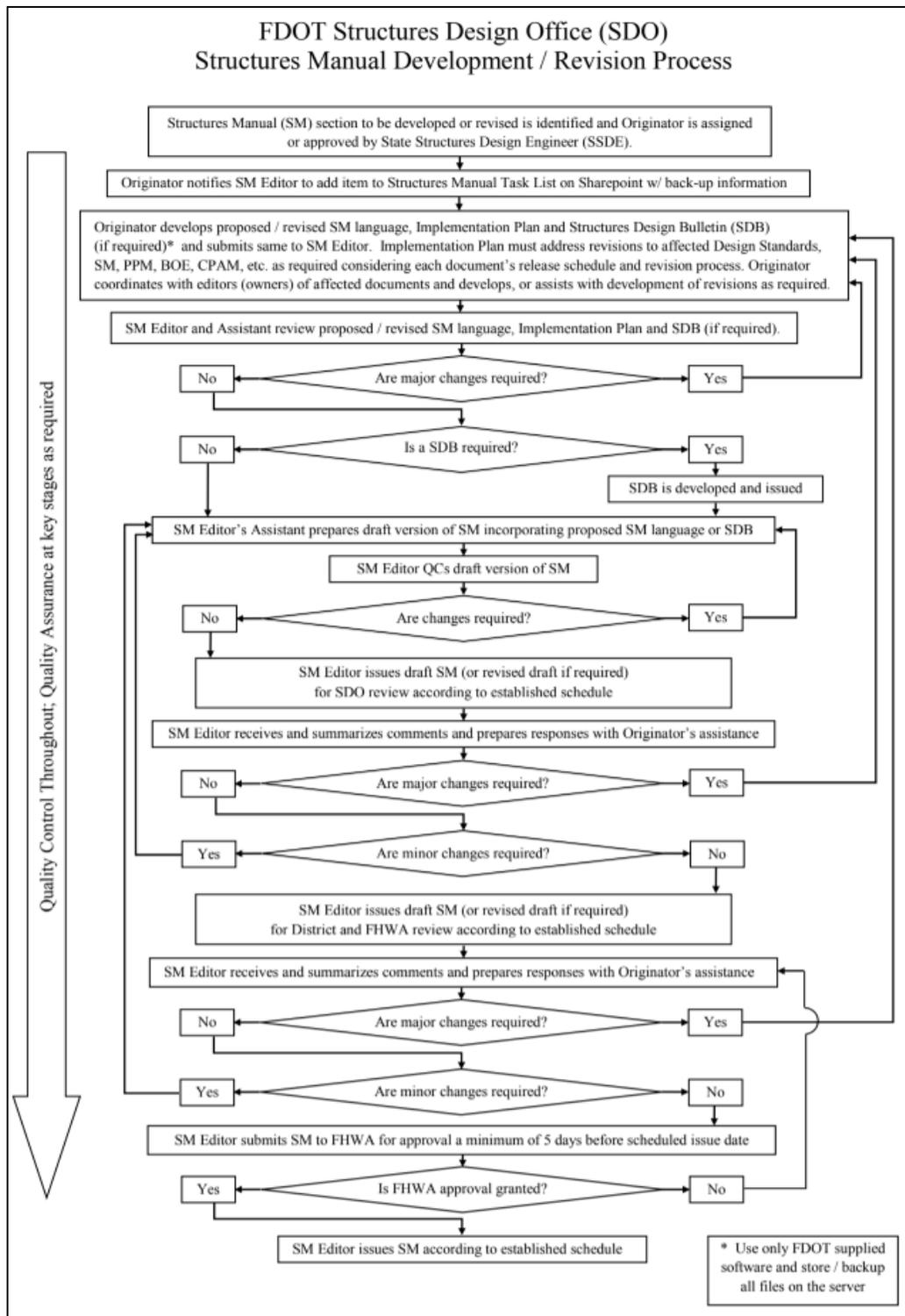
**Figure 3-19. The FDOT Structures Manual Development/Revision Process flowchart**
