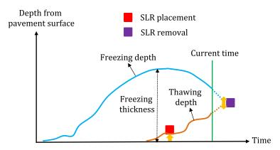
Figure 5.4 SLR decision-making based on the theory proposed by (Baïz et al. 2008)
