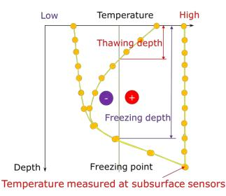
Figure 3.3 Calculation of freezing and thawing depths based on subsurface temperature measurements
