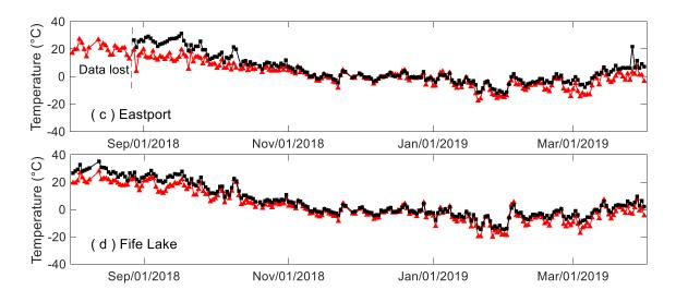
Figure 5.7 Measured air and pavement surface temperatures for Year Cycle 2018-2019
