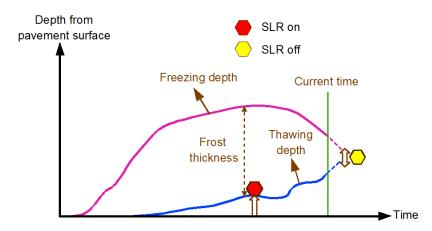
Figure 6.1 SLR decisions with freezing/thawing depth predictions (Baïz et al. 2008)
