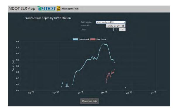
Figure 6.7 Measured variation of freezing/thawing depth
