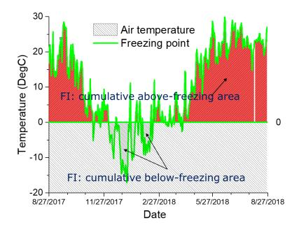
Figure 3.5 Calculation of freezing and thaw indices
