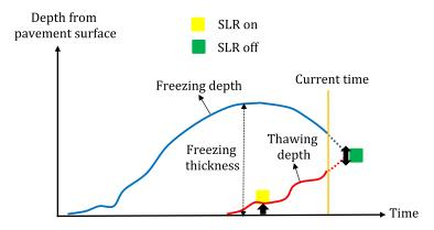
Figure 2.2 SLR decisions based on freezing/thawing depth predictions (modified after (Baïz et al. 2008))
