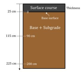
Figure 5.3 Schematic of a test road pavement cross section
