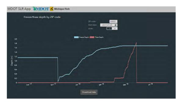
Figure 6.6 Predicted variation of freezing/thawing depth
