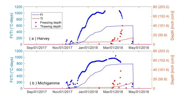
Figure 3.6 FI/TI calculated with the pavement surface temperature: (a) Harvey and (b) Michigamme
