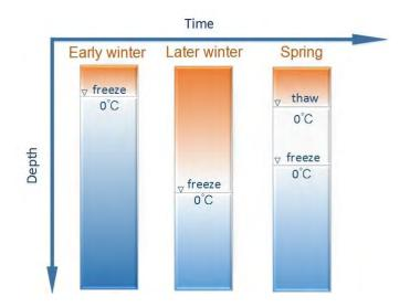
Figure 6.9 Variation of freezing and thawing depth with time
