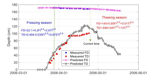
Figure 5.1 Measured vs predicted data for FD and TD [data is from (Baïz et al. 2008)]. Note that predicted TD and FD trends are obtained using the thawing season fitting constants.
