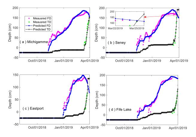
Figure 5.11 Predictions of FD and TD with the measured data for Year Cycle 2018-2019. Circled data Fig. 8 are excluded
