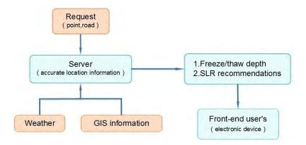
Figure 6.8 The calculation framework of the web-based tool
