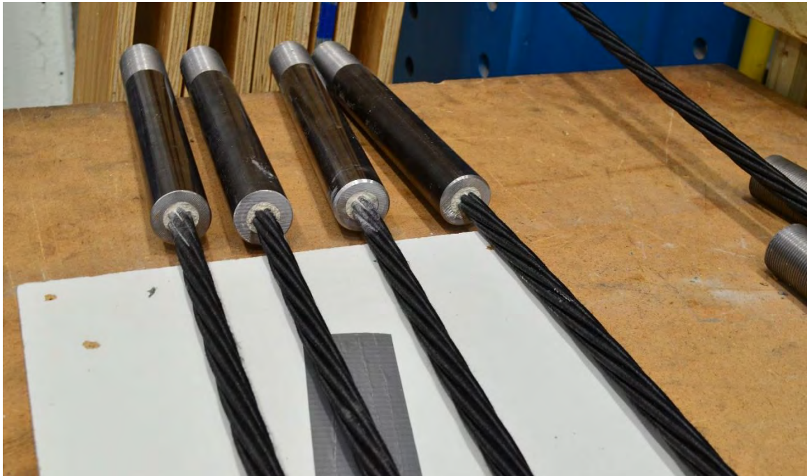
Figure 2.4-5 CFCC specimens with sleeve anchorage device after curing
