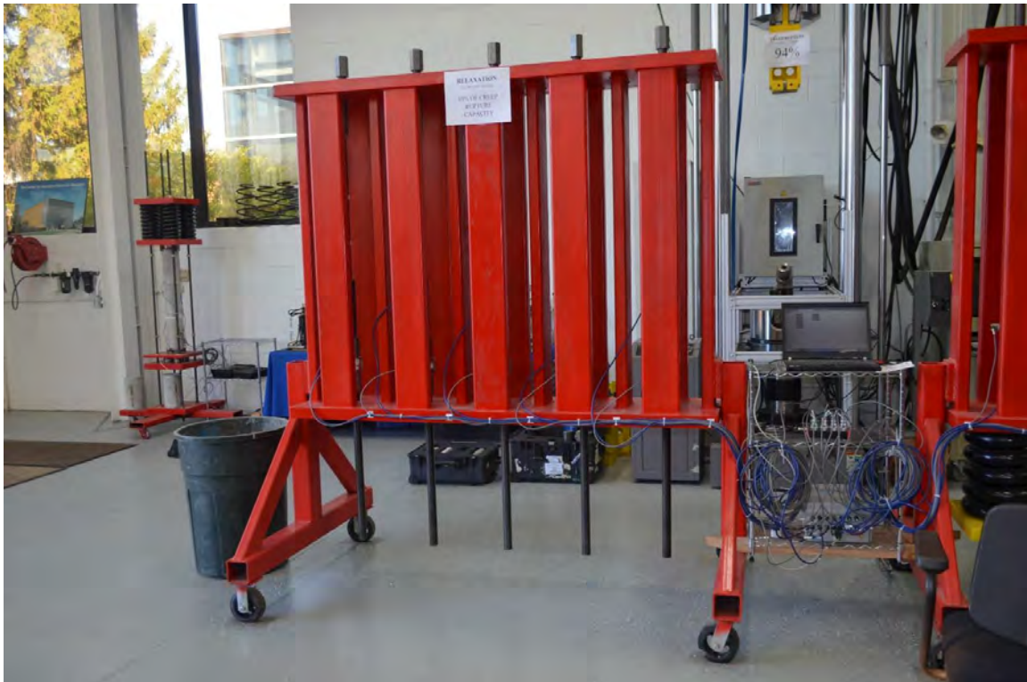
Figure 3.3-1 Relaxation test setup
