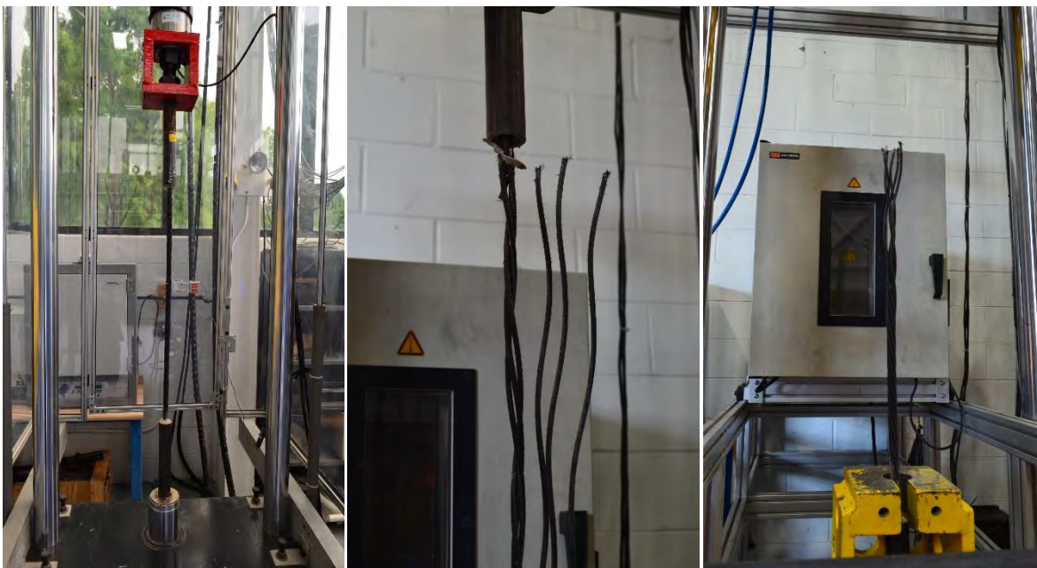
Figure 4.2-14 Uniaxial testing of CFCC specimens in Phase III
