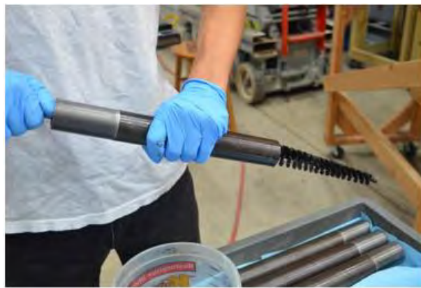
(c) Cleaning the socket
