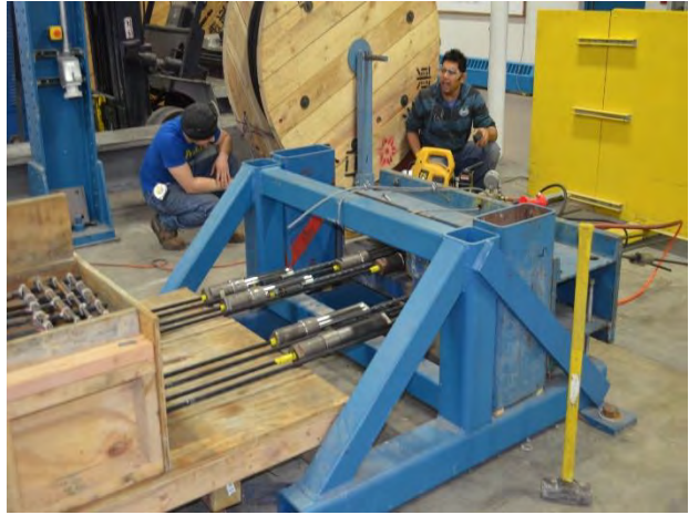
Figure 4.3-7 Applying prestressing force using a hydraulic pump
