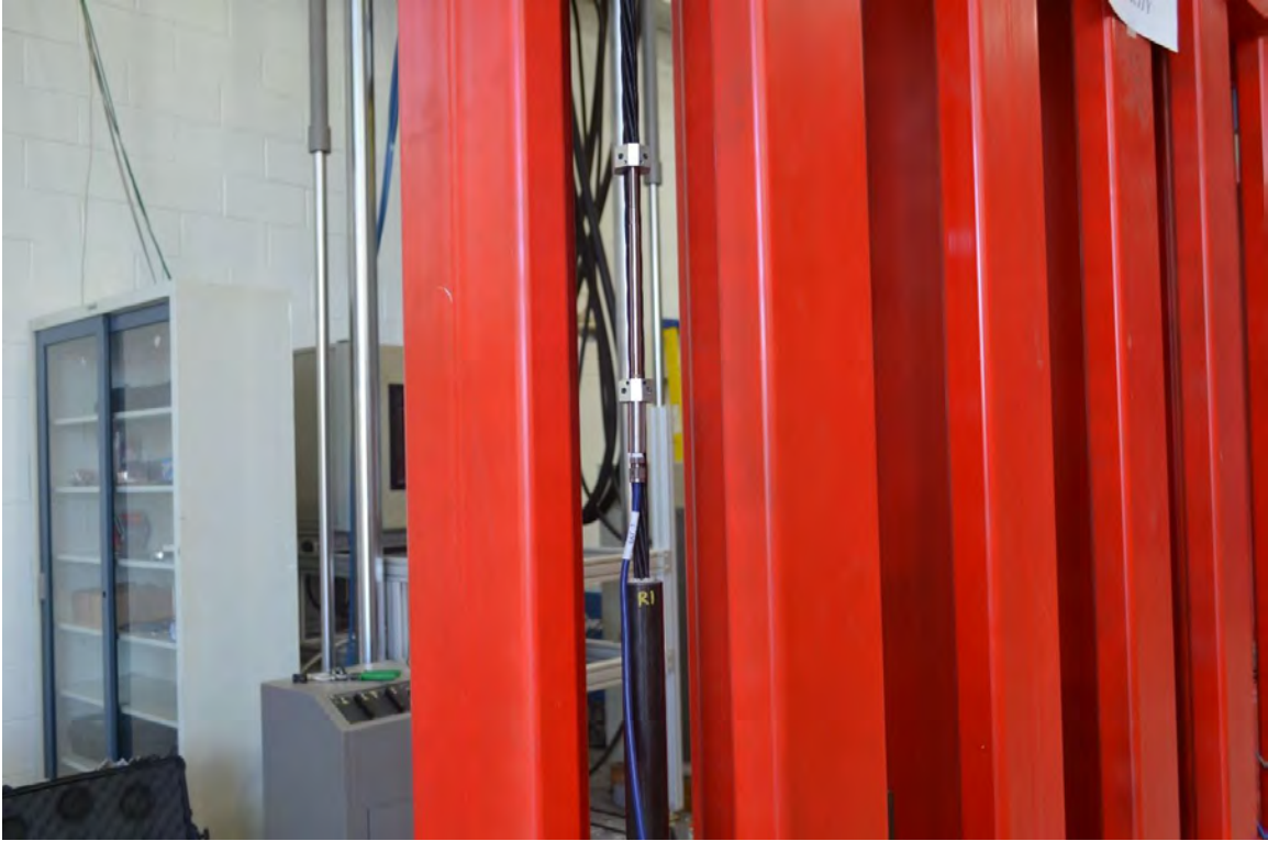
Figure 3.3-4 Strand-meters to evaluate the strain in CFCC relaxation specimens
