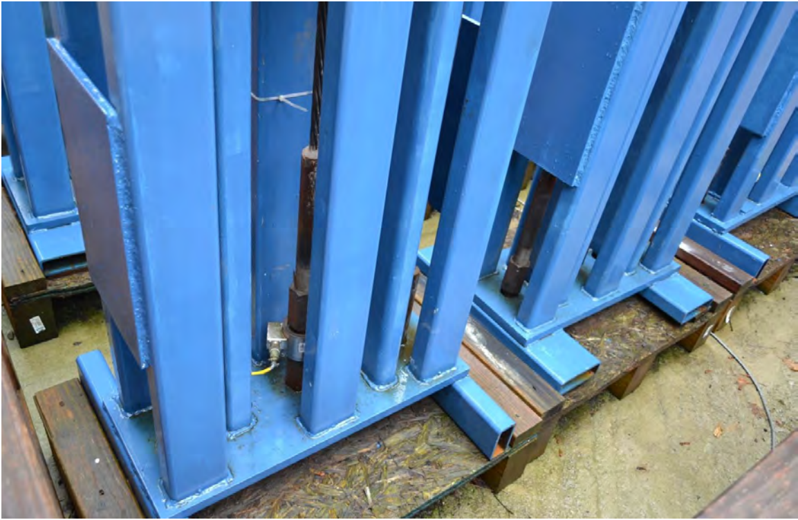
Figure 3.4-4 Monitoring the level of prestressing force through inline load cells attached to the CFCC specimens
