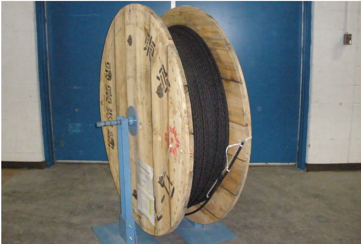
Figure 2.2-1 Spool of CFCC strands with a diameter of 0.6 in. (15.2 mm)
