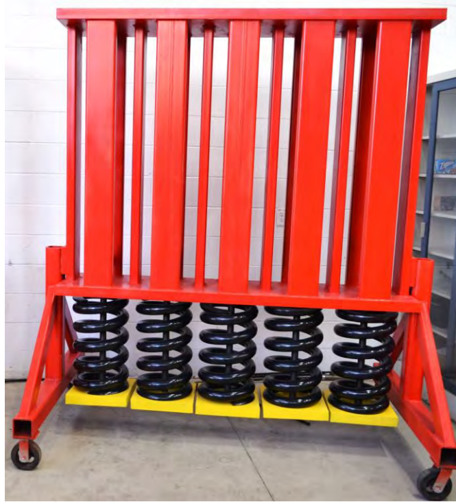
Figure 3.2-1 Test setup for evaluating creep rupture strength of CFRP with high strength steel springs to maintain the load level
