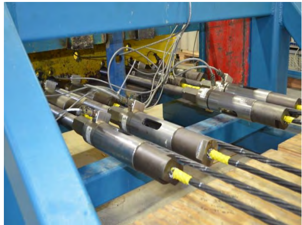
Figure 4.3-5 Passing prestressing CFCC strands through the reinforcement cages and connecting load cells and end couplers
