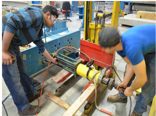
Figure 4.3-6 Attaching steel anchorage and applying prestressing force with a hydraulic jack
