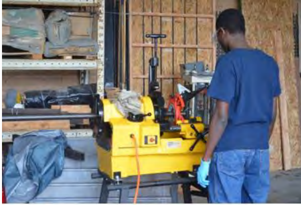
(a) Threading and cutting steel socket
