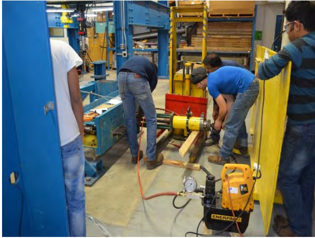
Figure 4.3-7 Applying prestressing force using a hydraulic pump
