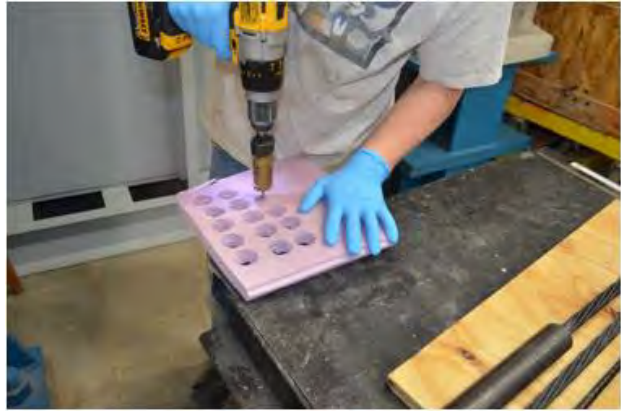
(b) Preparing end caps from Styrofoam
