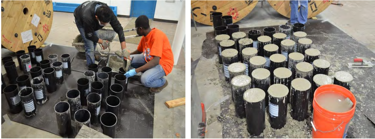
Figure 4.3-10 Preparing concrete cylinders for uni-axial compressive strength test
