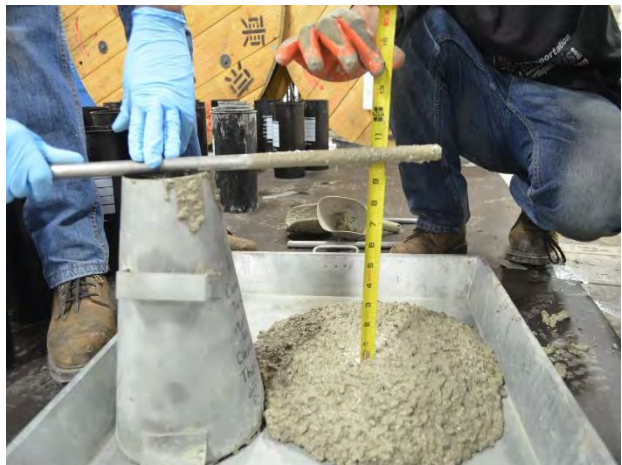
Figure 4.3-9 Slump test measuring 10 in. (254 mm)
