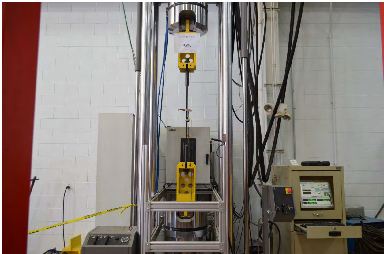
Figure 3.2-7 Creep rupture test setup for stress levels higher than 90 % of the CFCC average tensile strength
