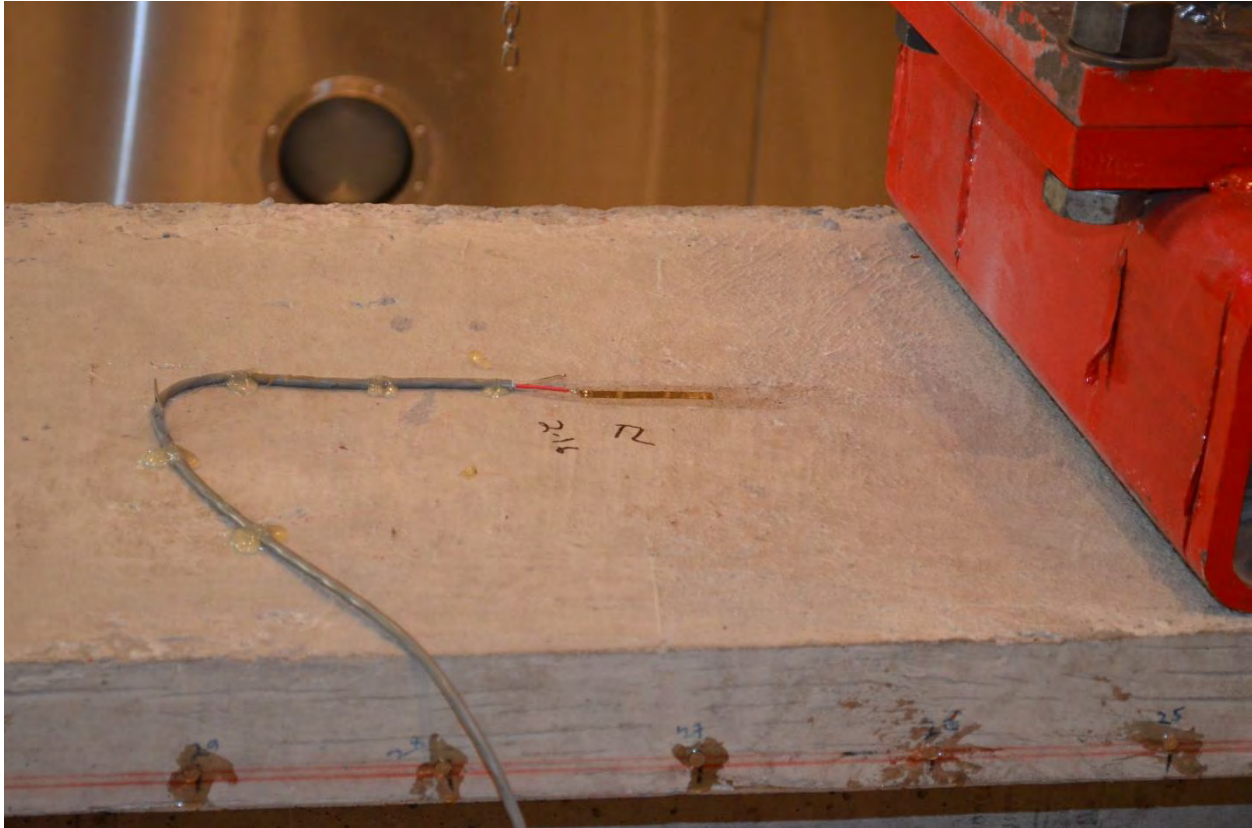
Figure 4.3-17 Strain gages on the top surface of the decked bulb T beam
