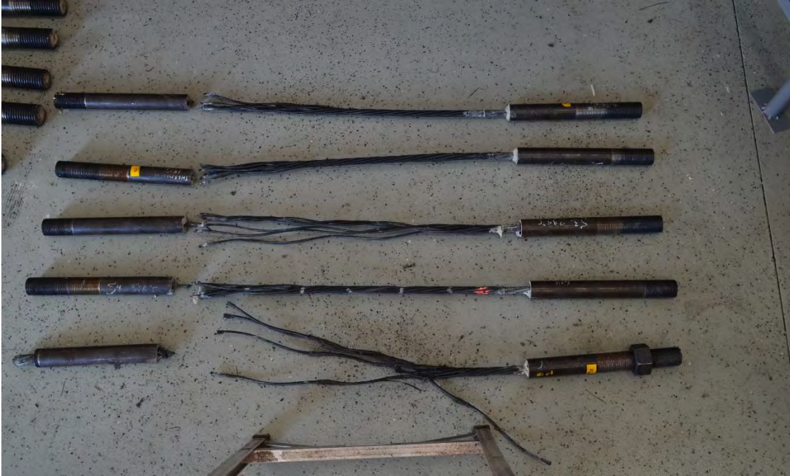
Figure 4.2-15 Failure of CFCC specimens in Phase III
