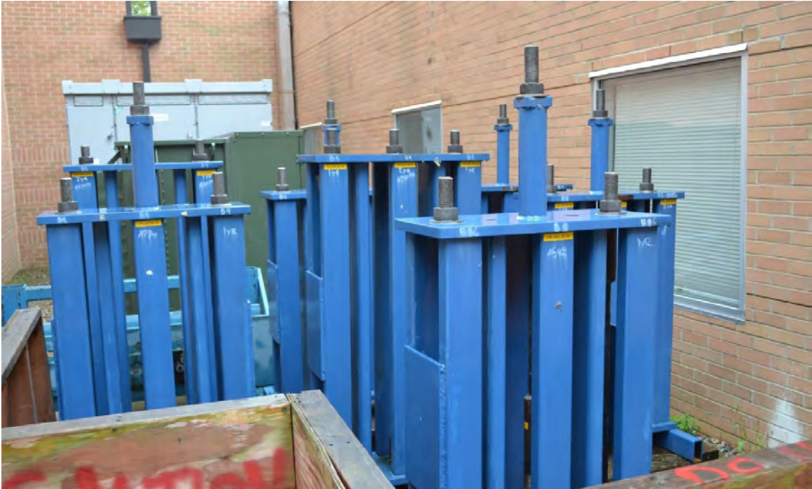
Figure 3.4-5 CFCC specimens stored outdoors after three years of continuous monitoring
