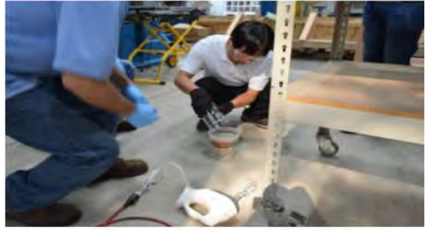
(b) Adding water and mixing HEM
