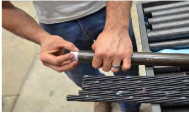
(a) Capping the ends of the steel sockets
