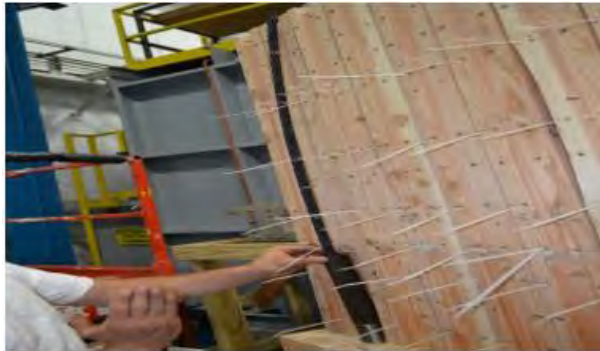
(b) Placing specimen in wooden stand
