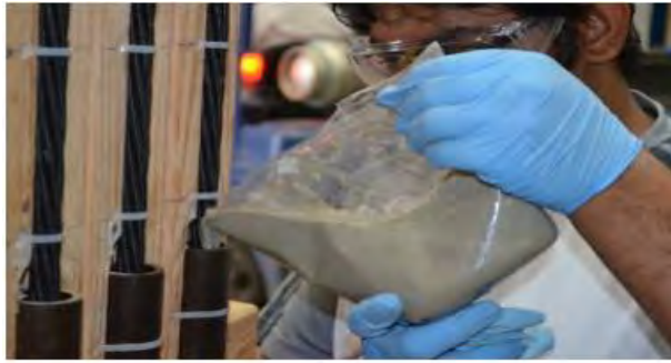
(c) Pouring HEM to the socket
