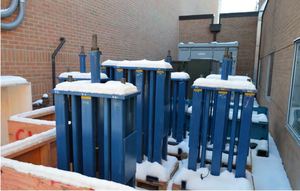
Figure 3.4-3 Long-term monitoring of prestressed CFCC specimens stored outdoors and exposed to Michigan weather
