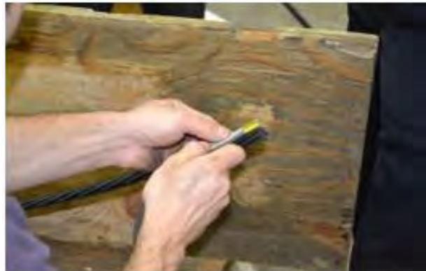
(b) Wrapping steel mesh around CFCC
