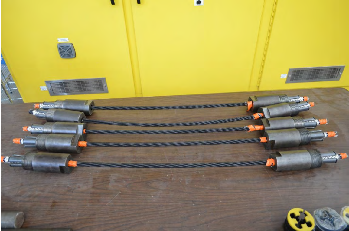
Figure 2.3-4 Test specimens prepared using composite buffer layer and wedge anchorage
