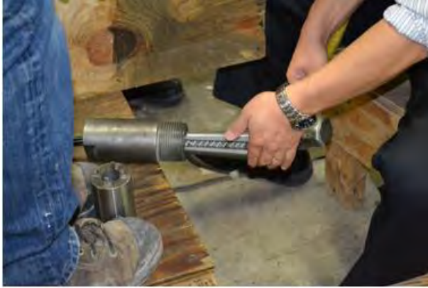
(a) Sliding steel wedges into barrel
