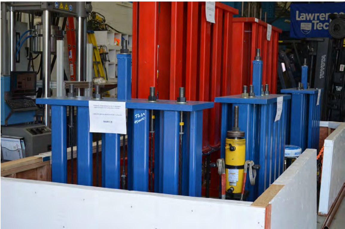
Figure 3.4-2 Long-term monitoring of CFCC specimens in a controlled laboratory environment
