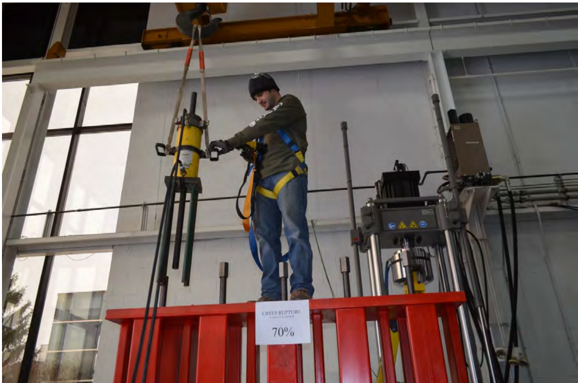
Figure 3.2-2 Stressing creep rupture specimens to 70 % of the average tensile strength of CFCC
