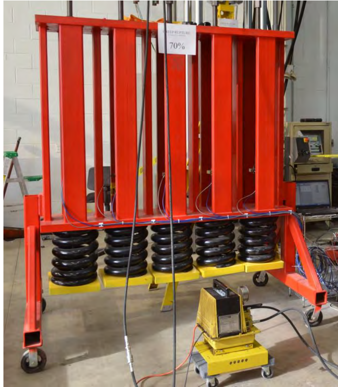
Figure 3.2-3 Creep rupture specimens after stressing showing the compressed steel springs
