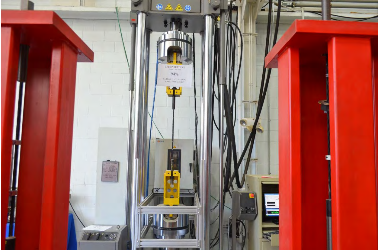
Figure 3.2-8 Creep-rupture test setup for stress level of 94 % of average CFCC tensile strength
