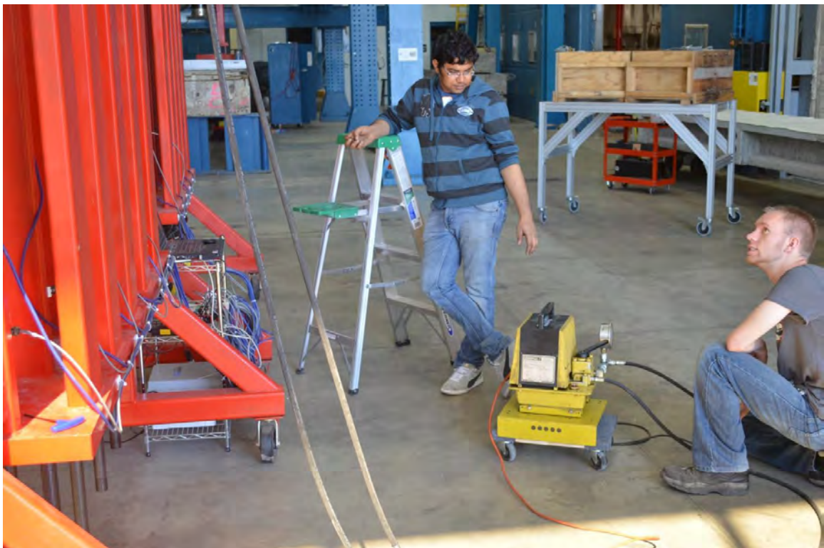
Figure 3.3-3 Stressing relaxation specimens to an initial load level of 47.5 kip (211 kN)
