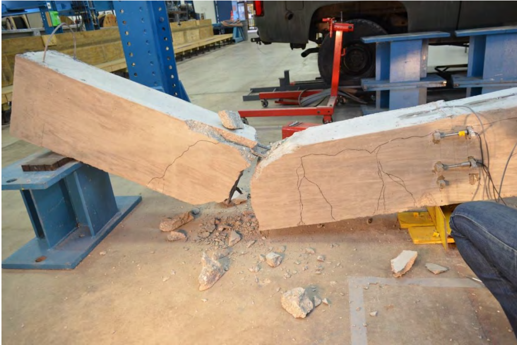
Figure 7.3-25 Crushing of concrete followed by rupture of CFCC strands in BC-0.6
