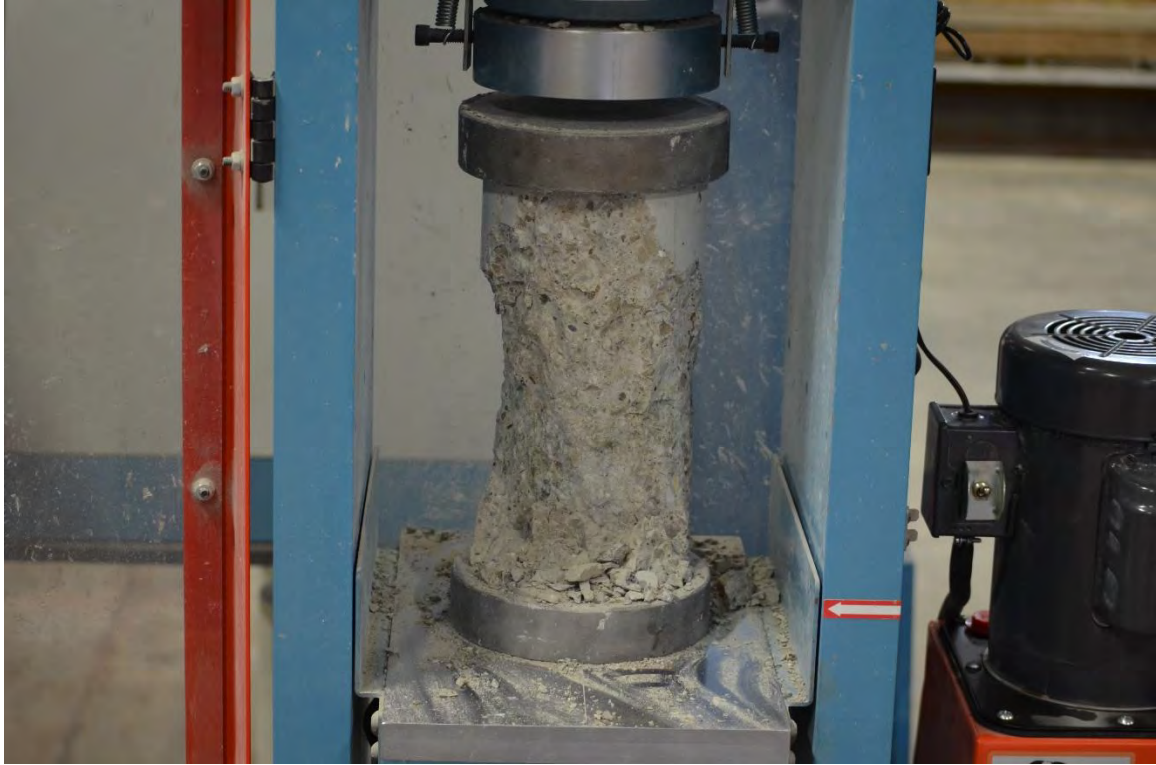
Figure 5.2-13 Testing and failure of control cylinders
