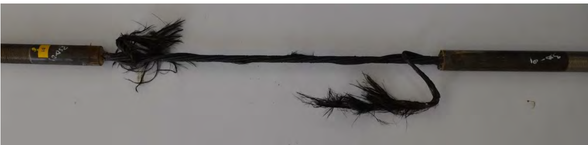
Figure 6.2-11 Failure of CFCC specimen at 662 °F (350 °C)
