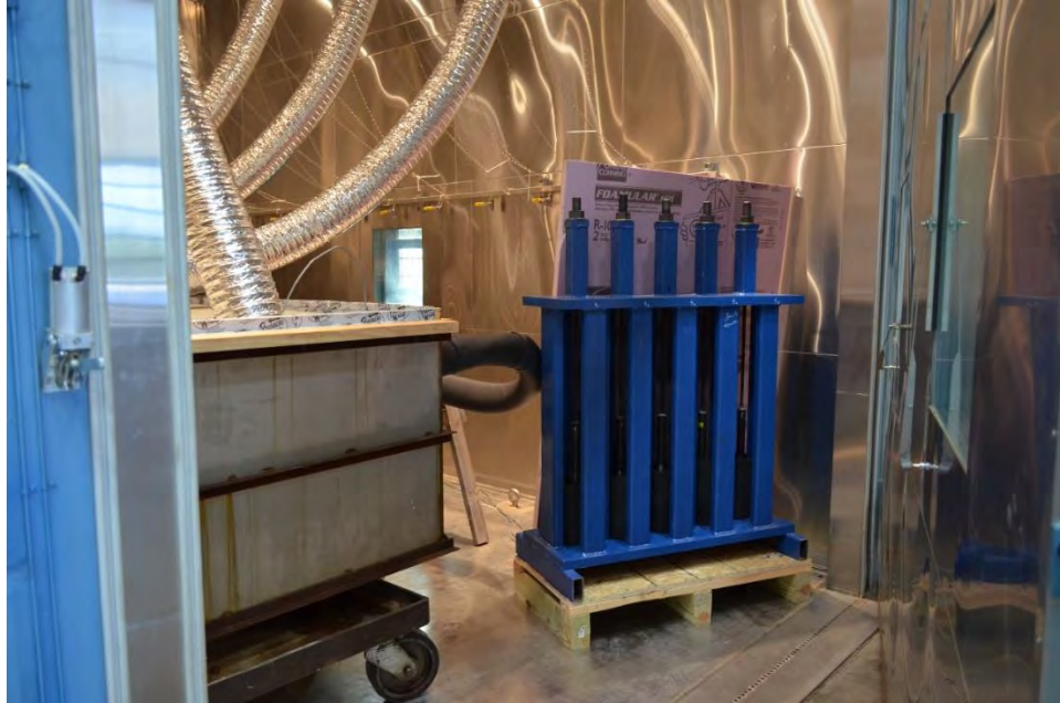
Figure 5.3-3 CFCC specimens in the Environmental Chamber along with the beams
