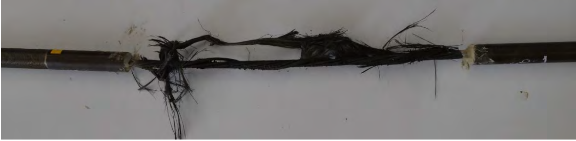
Figure 6.2-7 Failure of CFCC specimen at 482 °F (250 °C)
