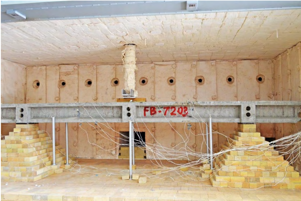
Figure 6.3-16 Beam C72-14-1 before fire
