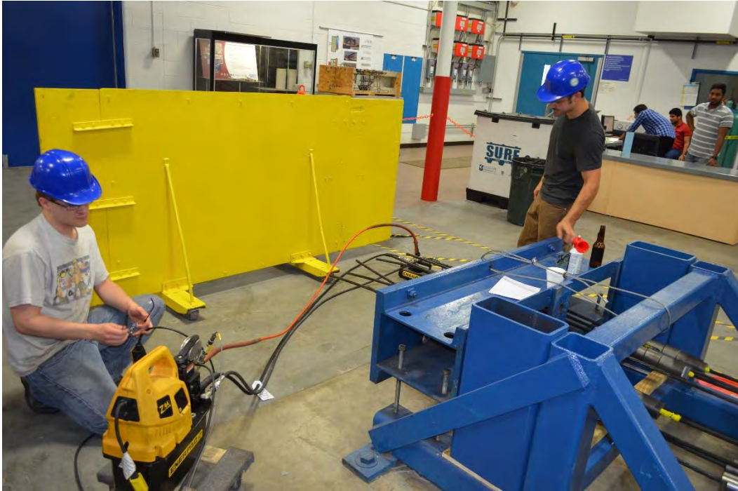
Figure 7.4-9 Prestressing CFCC strands from the live end
