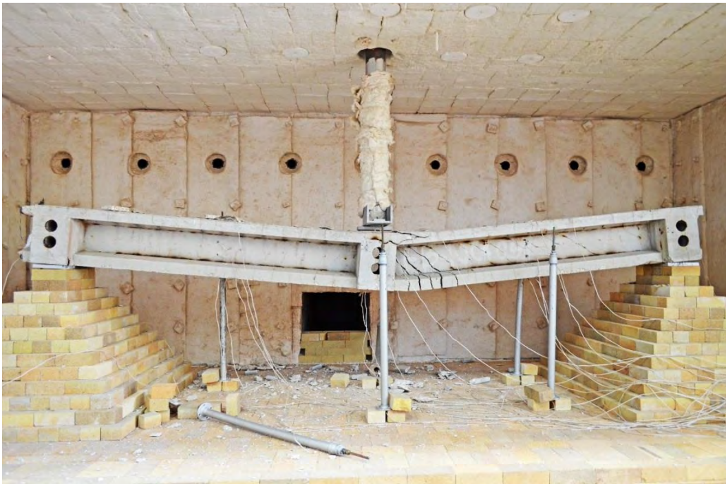
Figure 6.3-37 Beam C100-20-3 after fire
