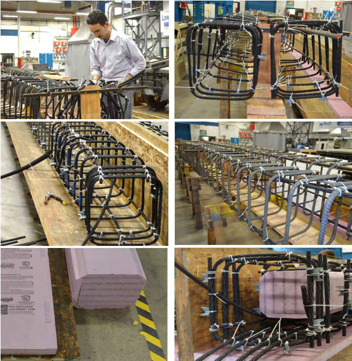
Figure 7.4-7 Preparing and instrumenting the reinforcement cages
