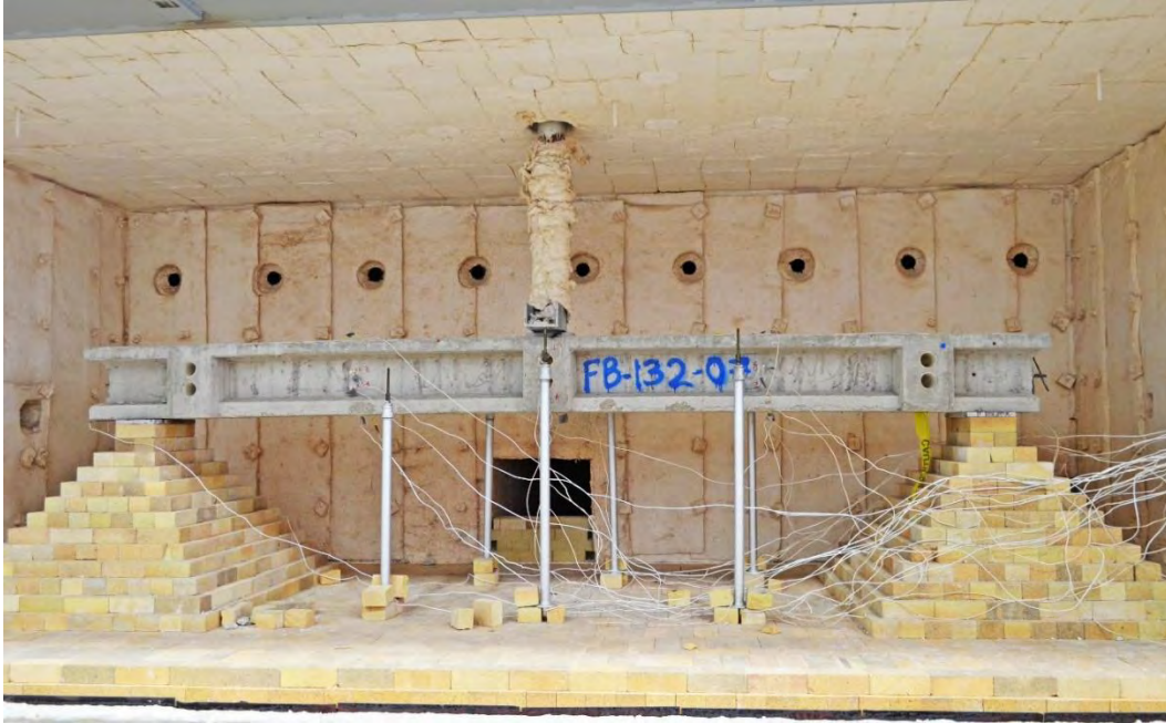
Figure 6.3-54 Beam C132-25-1 before fire
