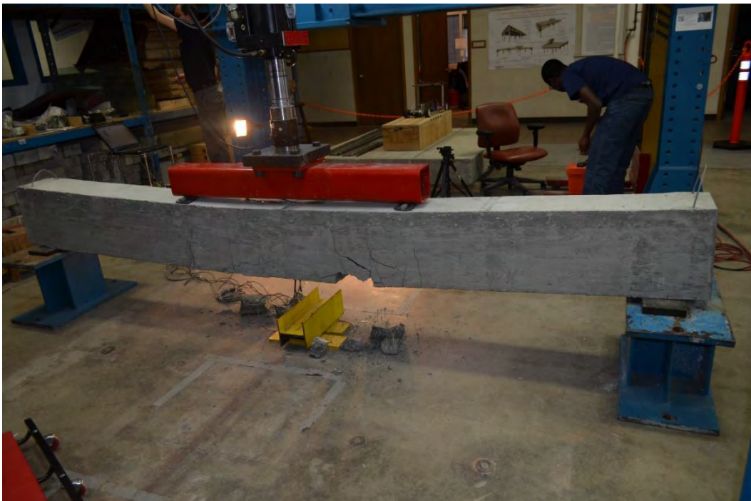
Figure 7.3-36 Failure of B4-0.6
