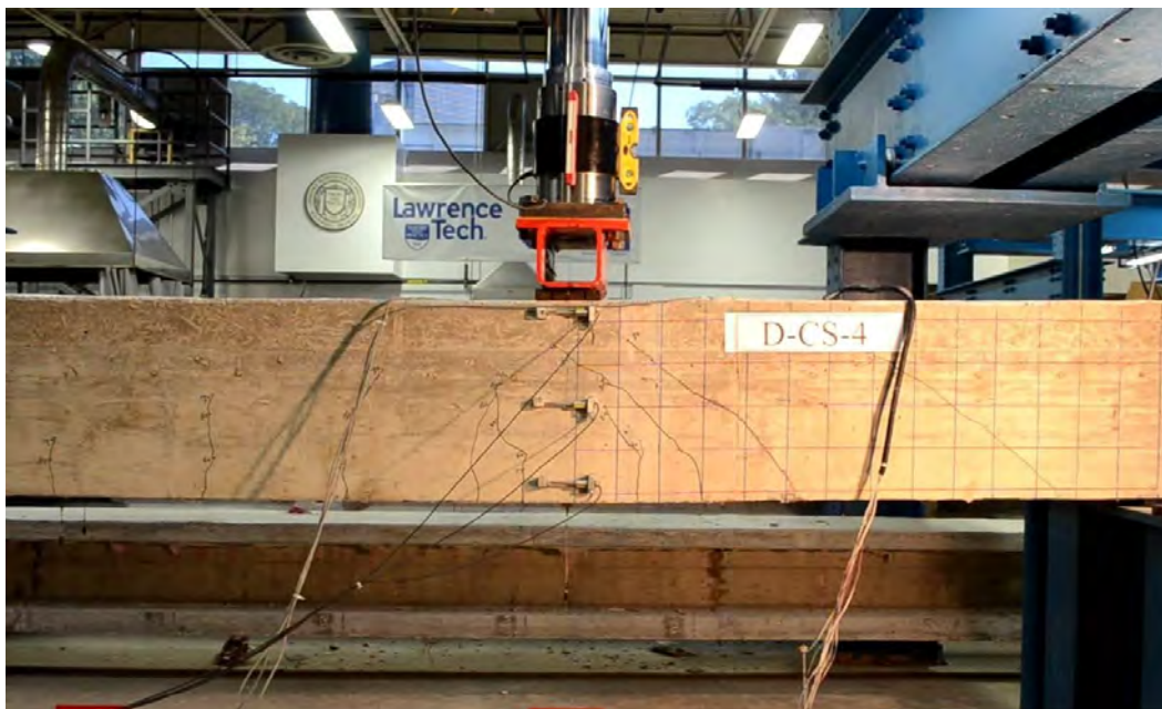
Figure 7.4-30 Crack pattern of beam C-4
