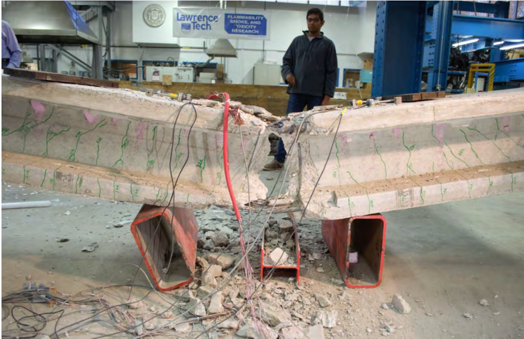
Figure 8.2-54 Failure of Beam I-2
