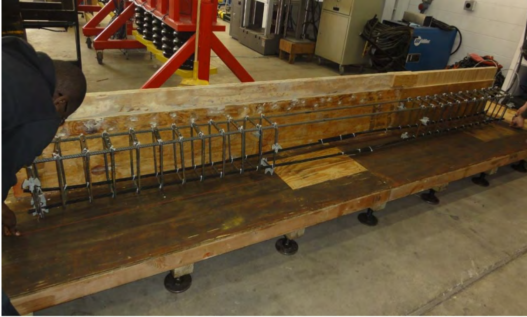
Figure 7.3-4 Completed reinforcement cage showing the location of the splice and stirrups
