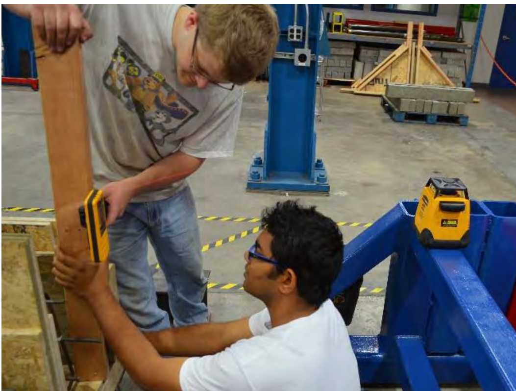
Figure 8.2-7 Leveling the platform using a laser level
