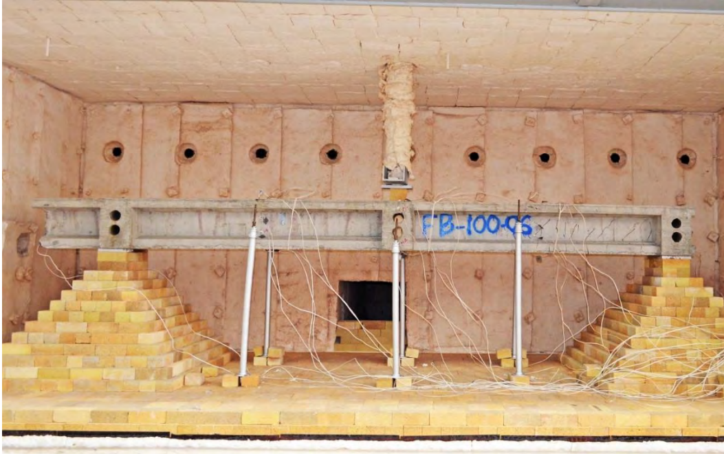
Figure 6.3-42 Beam C100-20-4 before fire
