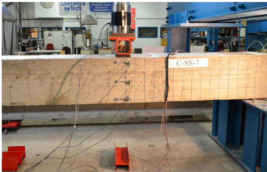
Figure 7.4-42 Crack pattern of beam S-7
