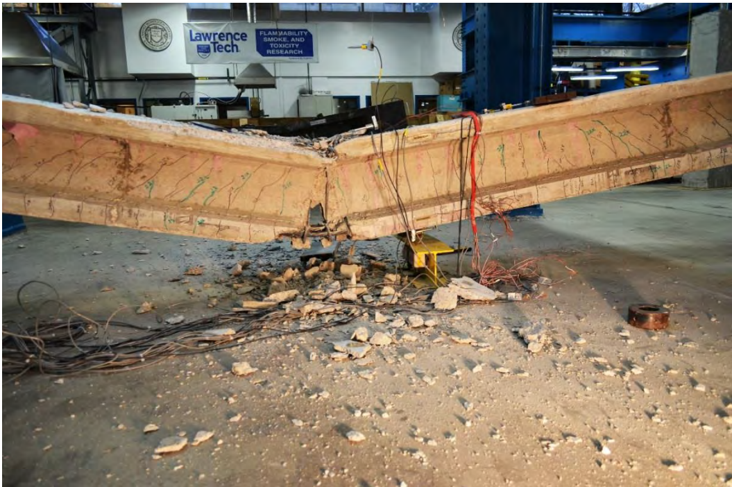
Figure 8.2-49 Failure of Beam I-1
