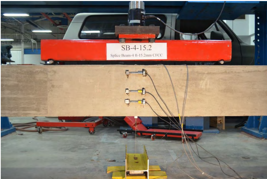
Figure 7.3-35 Setup and testing of B4-0.6
