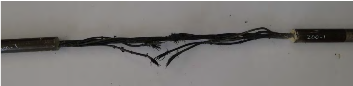
Figure 6.2-5 Failure of CFCC specimen at 392 °F (200 °C)
