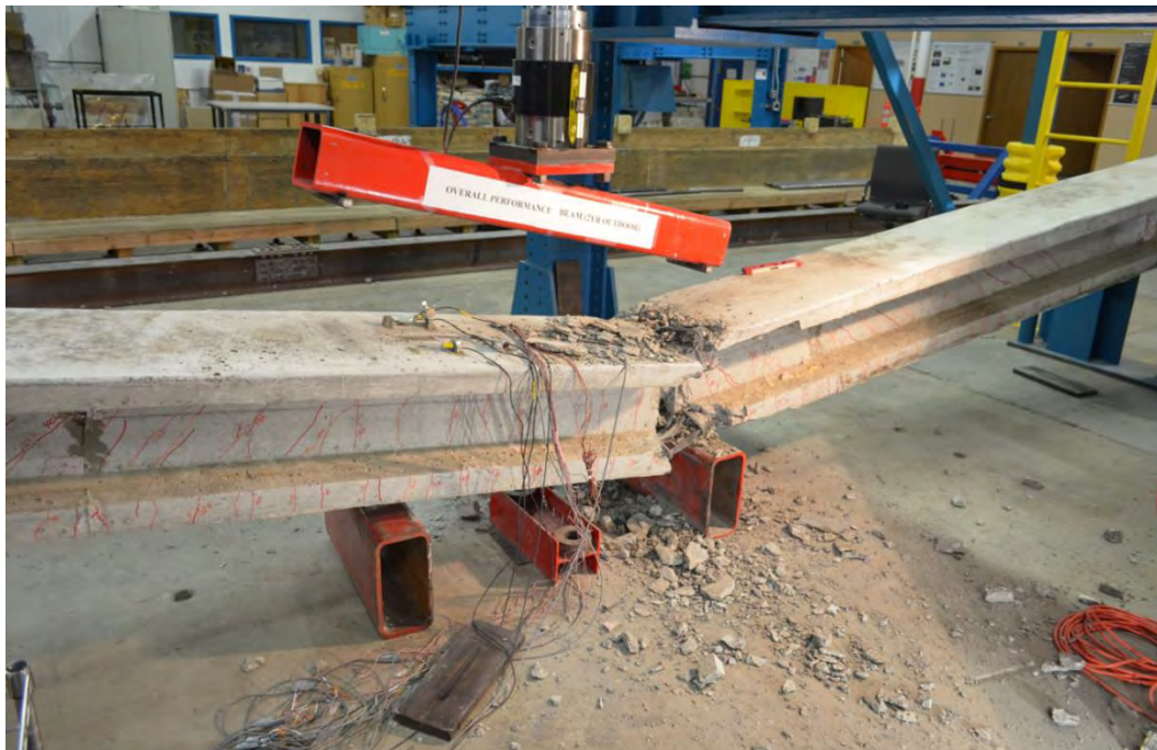
Figure 8.2-57 Failure of Beam O-2
