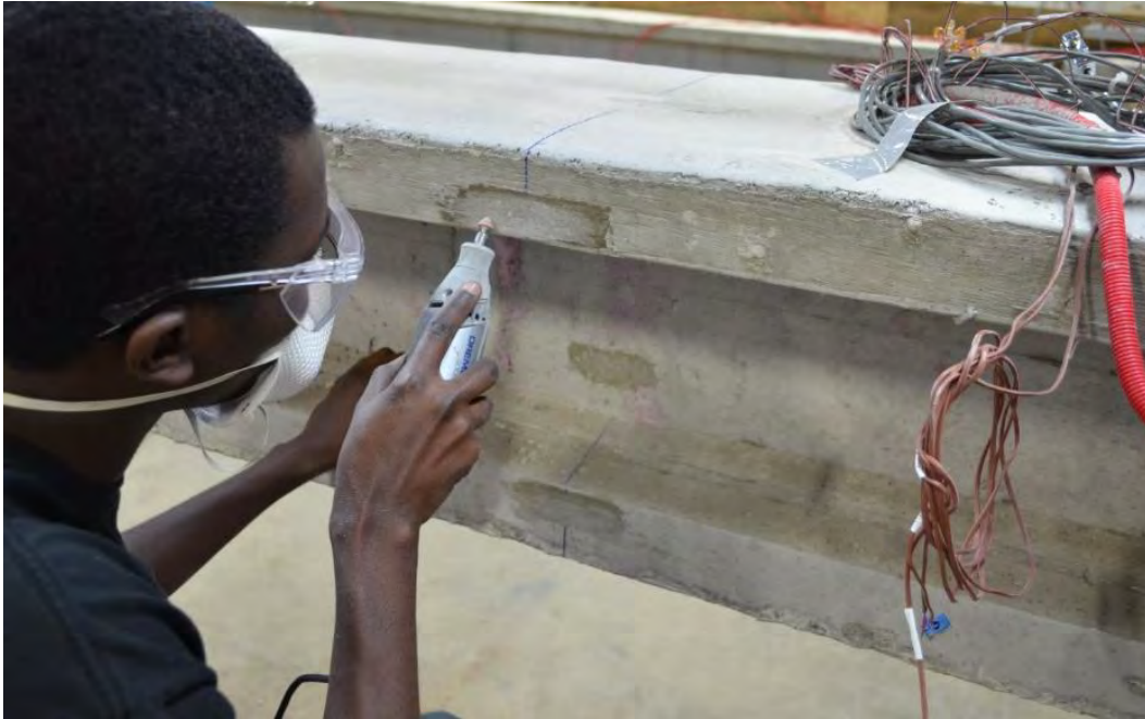
Figure 8.2-18 Smoothing the surface before installing strain gages
