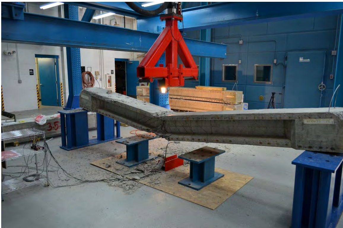
Figure 5.2-33 Failure of Beam H1
