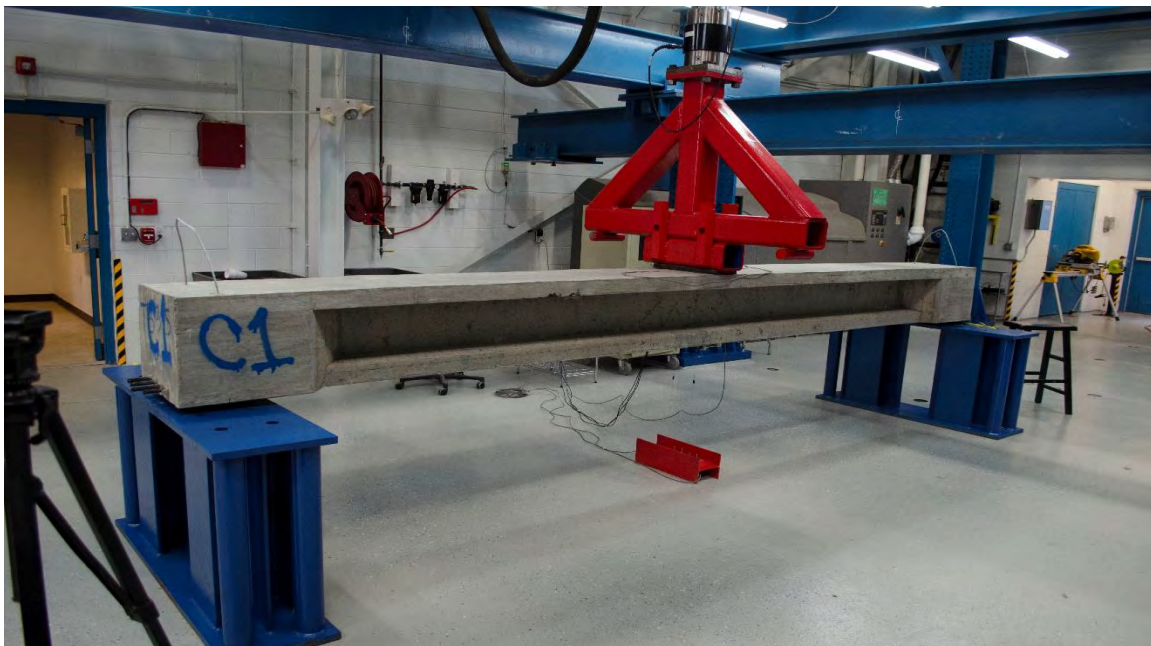
Figure 5.2-15 Flexural test setup for control beam C1
