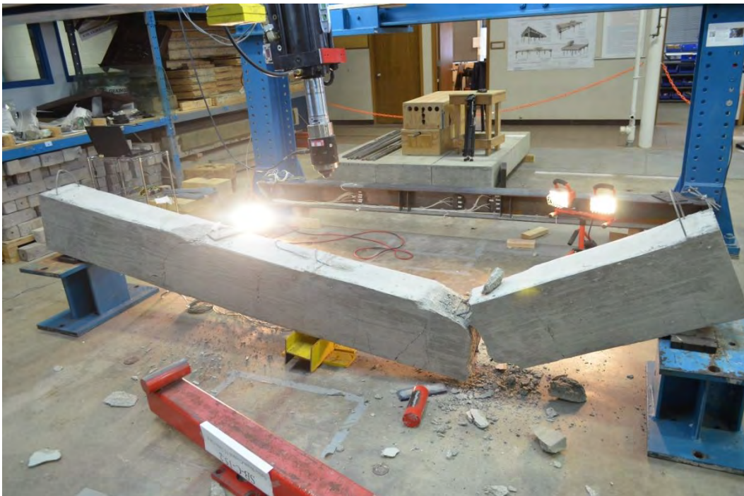
Figure 7.3-24 Failure of BC-0.6
