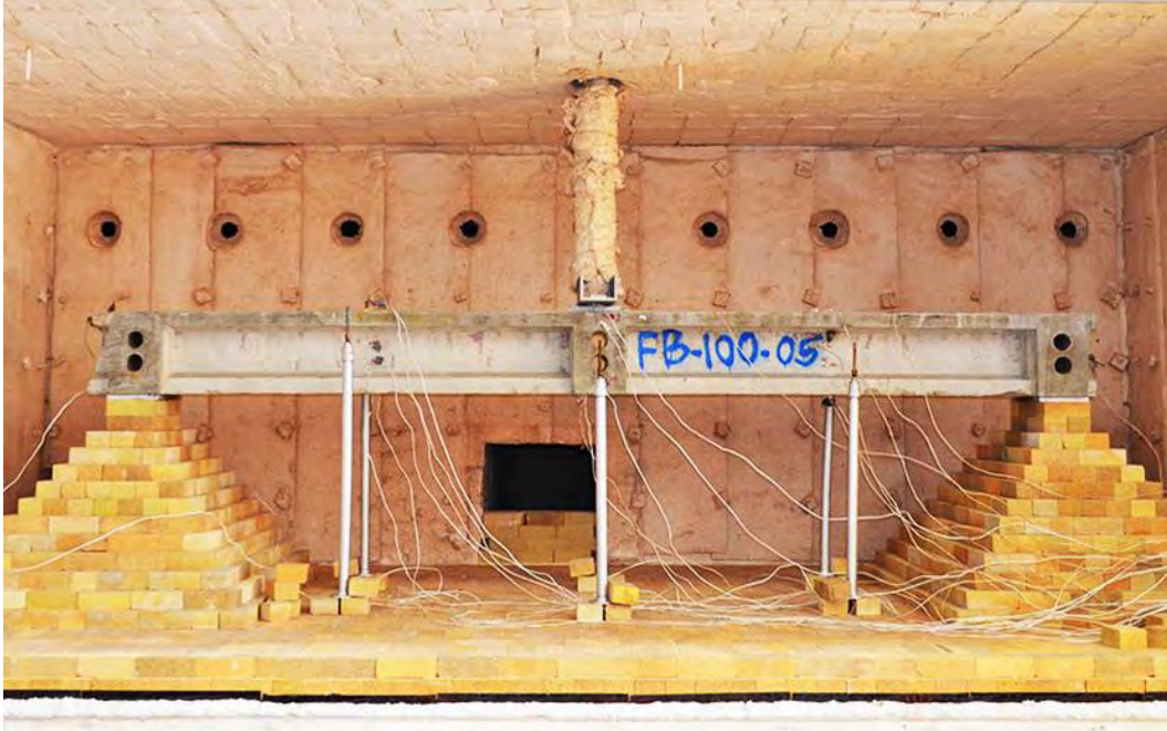
Figure 6.3-36 Beam C100-20-3 before fire
