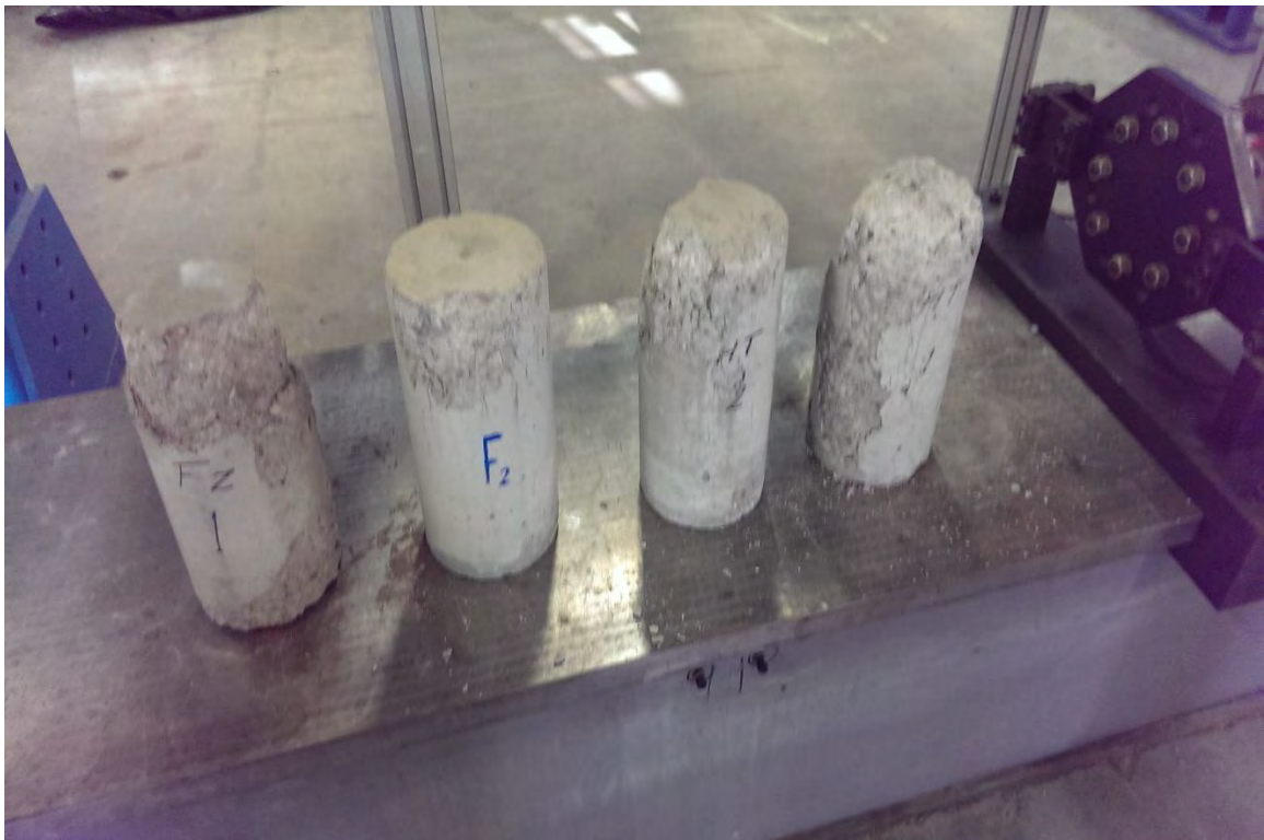
Figure 5.2-12 Testing and failure of concrete cylinders after exposure to freeze-thaw cycles
