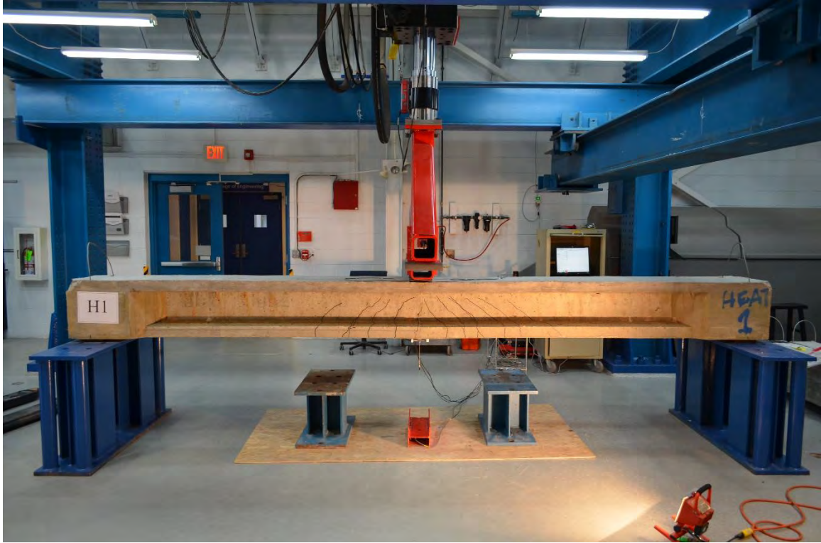
Figure 5.2-32 Test setup for Beam H1 after exposure to freeze-thaw cycles
