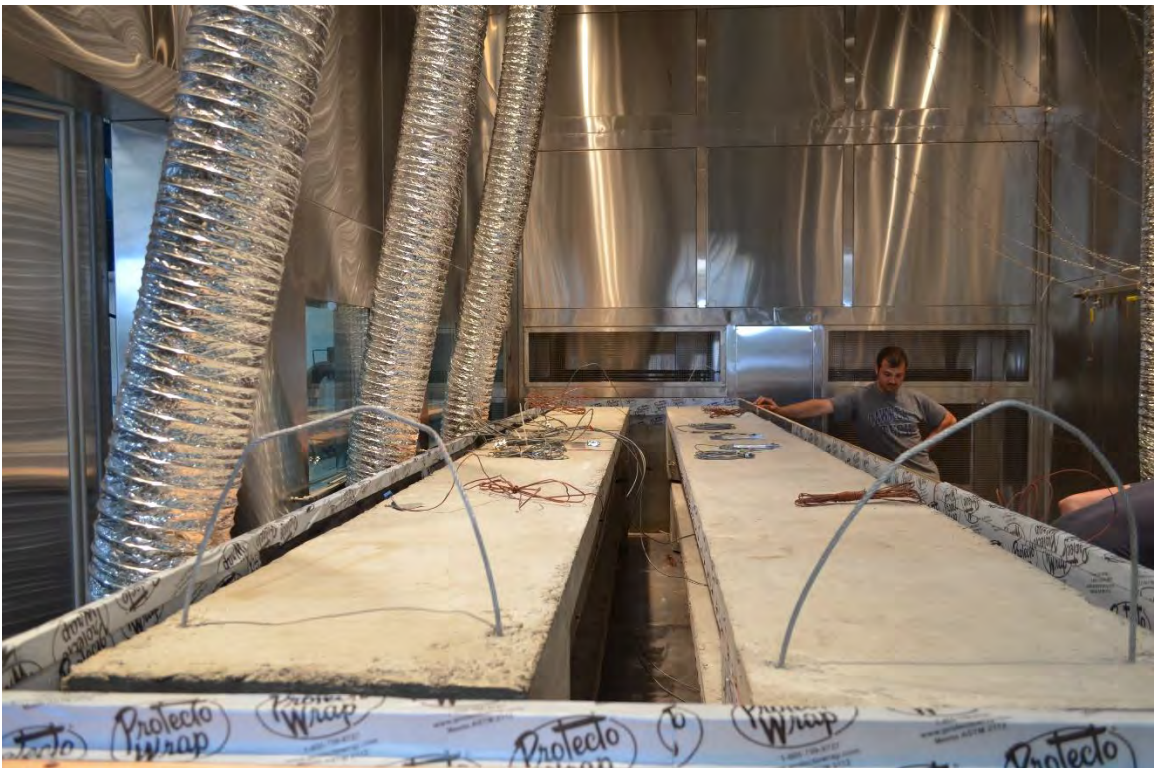
Figure 5.2-3 Decked bulb T beam placed in the tank for freeze-thaw testing
