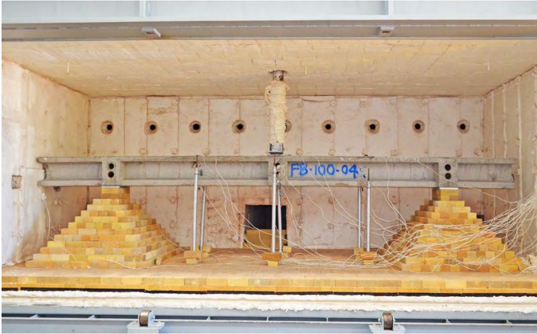
Figure 6.3-30 Beam C100-20-2 before fire
