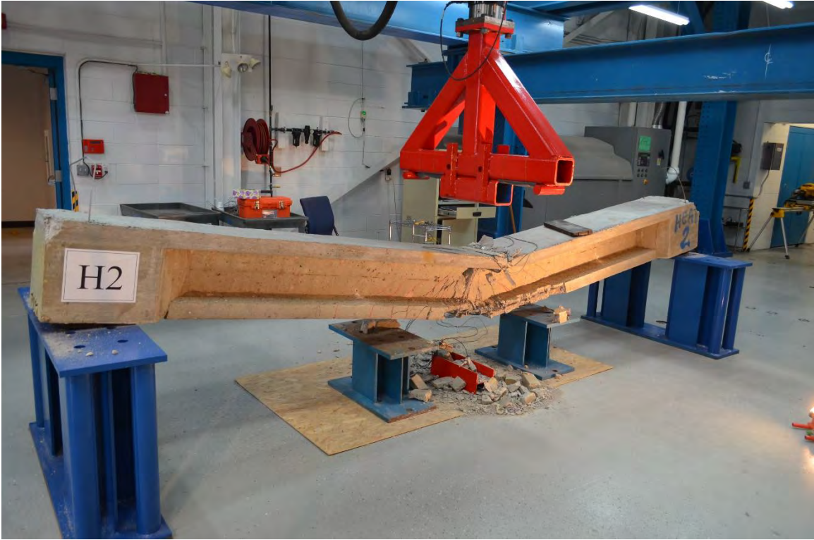
Figure 5.2-37 Failure of Beam H2
