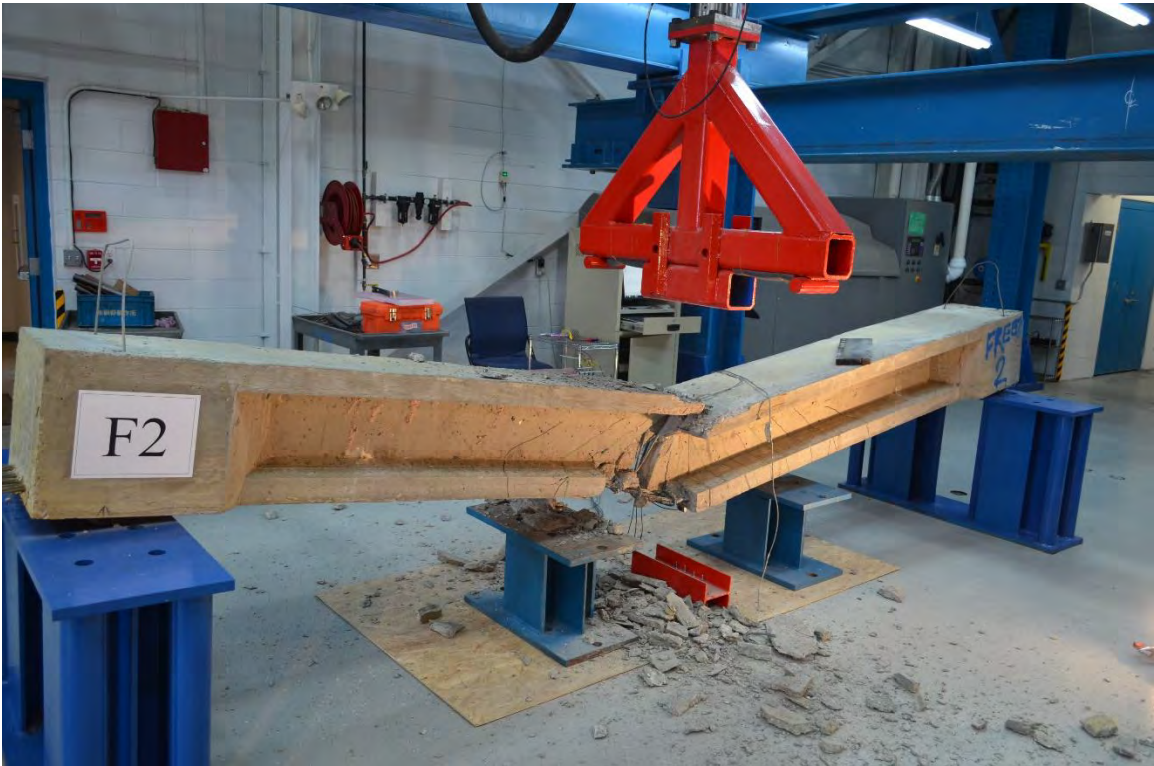
Figure 5.2-29 Failure of Beam F2
