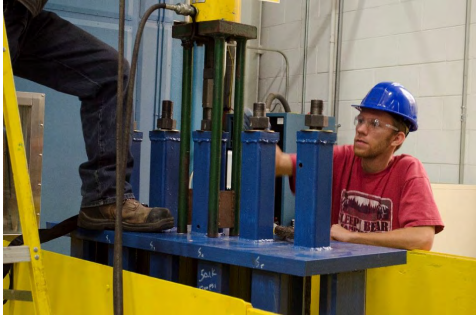
Figure 5.3-7 Releasing CFCC strands after freeze-thaw exposure
