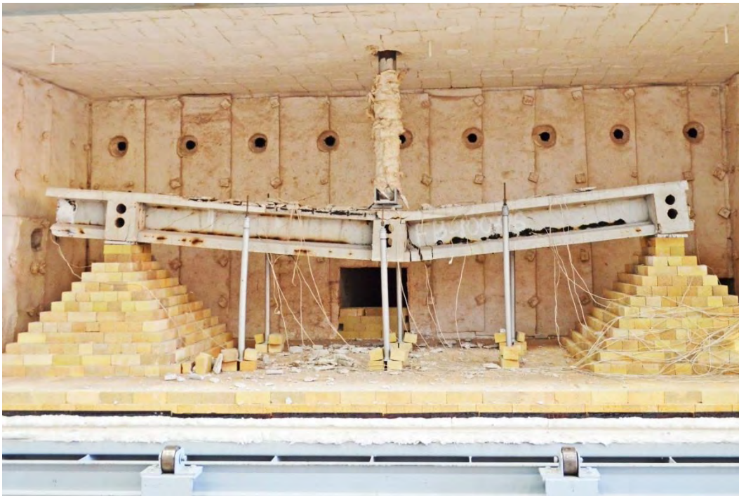
Figure 6.3-43 Beam C100-20-4 after fire
