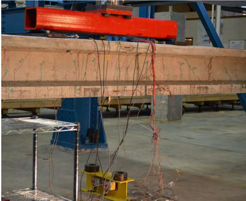
Figure 8.2-20 Instrumentation of decked bulb T beams at mid-span
