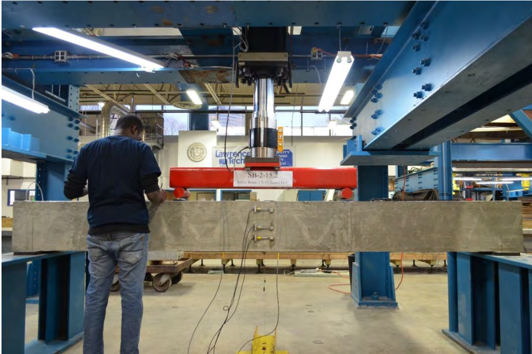
Figure 7.3-29 Setup and testing of B2-0.6
