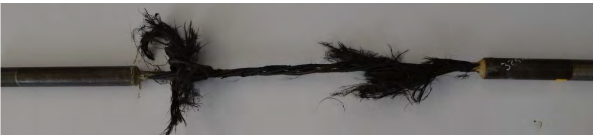
Figure 6.2-10 Failure of CFCC specimen at 617 °F (325 °C)
