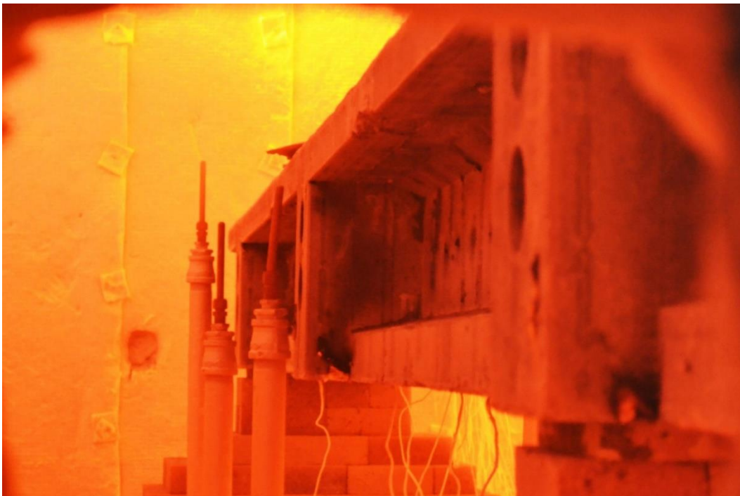
Figure 6.3-49 Beam C100-20-5 during fire
