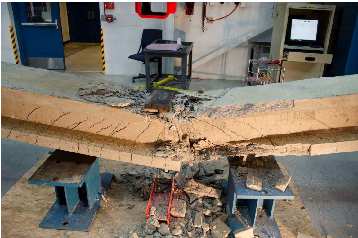
Figure 5.2-25 Failure of Beam F1
