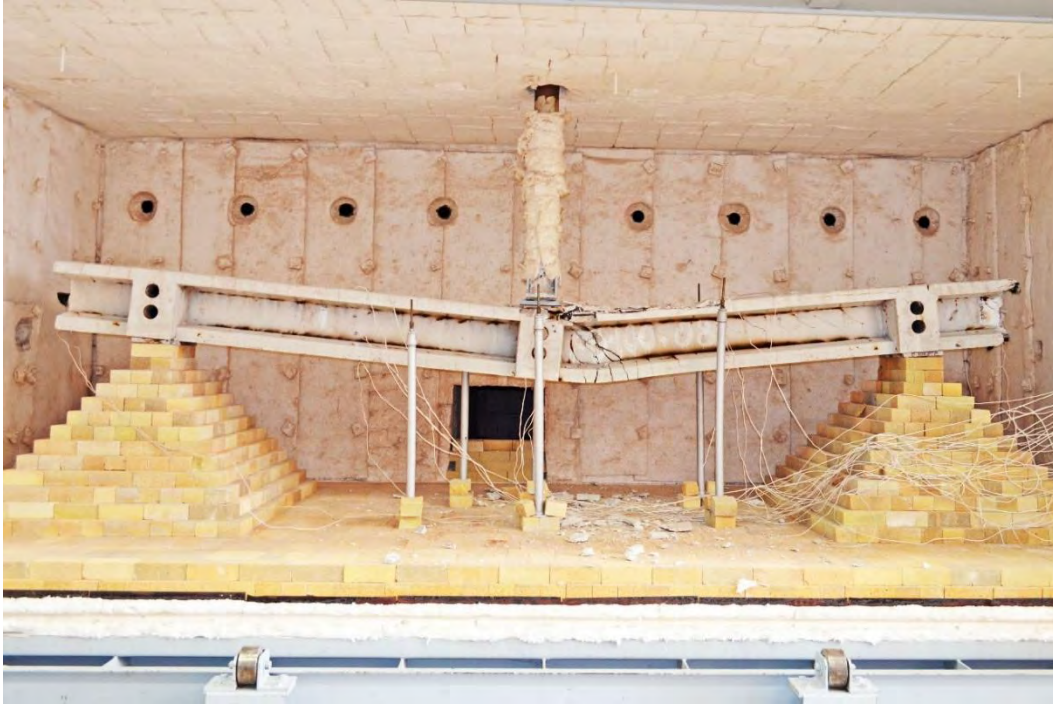
Figure 6.3-50 Beam C100-20-5 after fire
