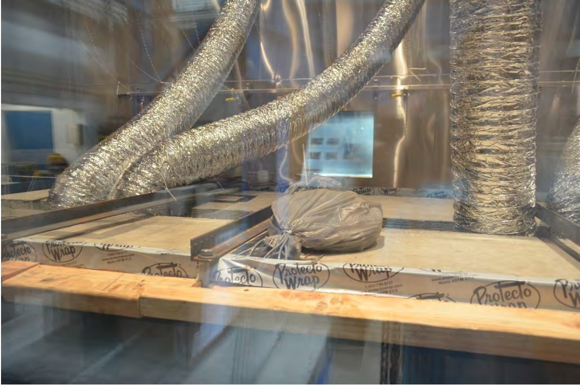
Figure 5.2-6 Decked bulb T beams during freezing and thawing cycles
