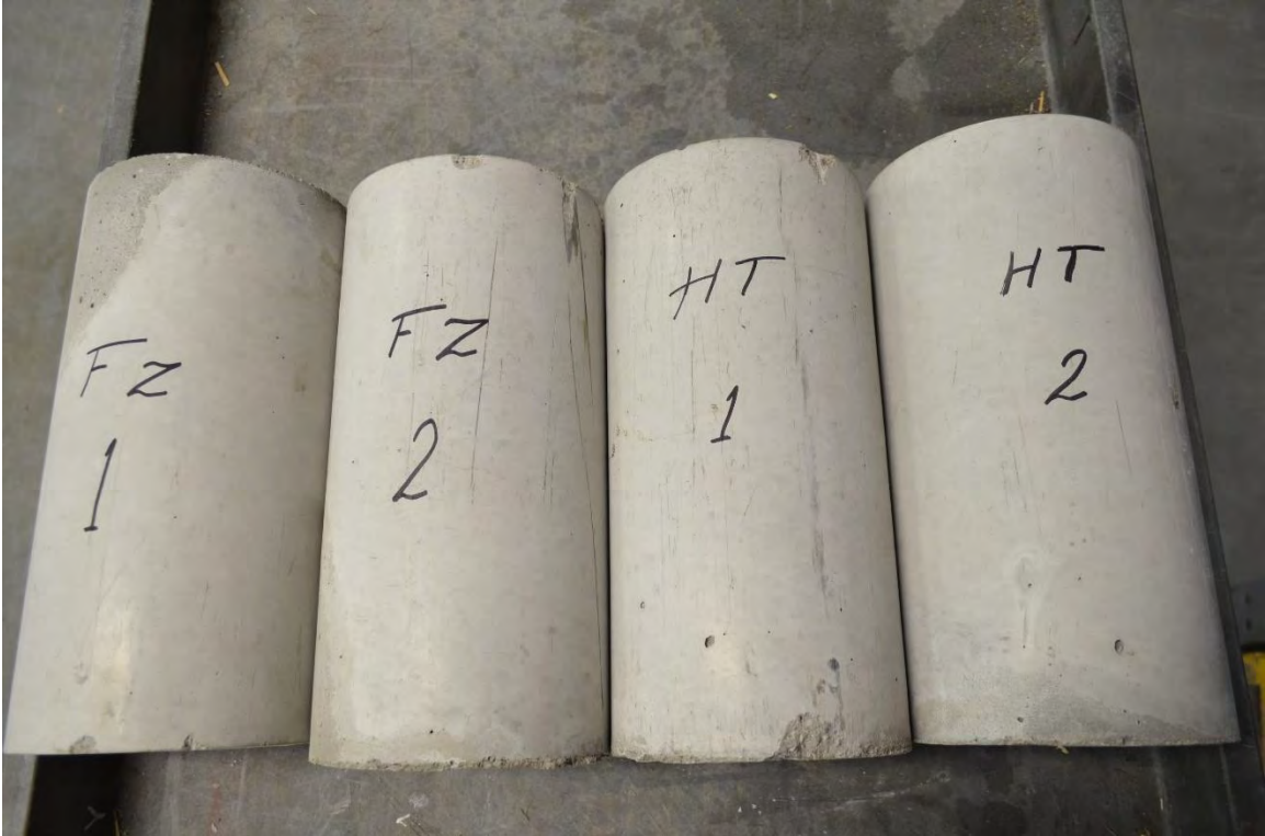
Figure 5.2-4 Concrete cylinders from the same batch as the beams placed with the beams and exposed to freeze-thaw cycles. Other cylinders are stored at Lab. conditions
