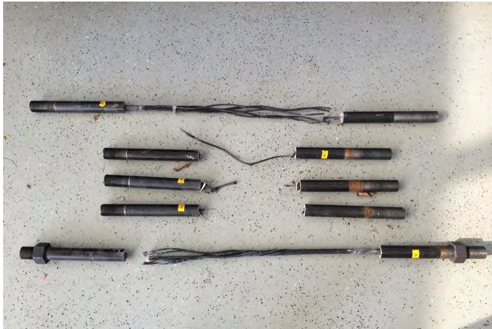
Figure 5.3-10 Failure of CFCC strands under uni-axial load test setup
