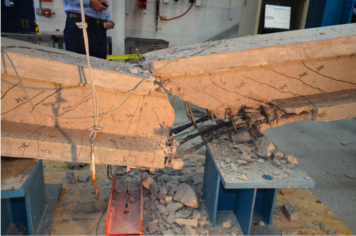
Figure 5.2-18 Close-up view showing the rupture of CFCC strands in Beam C1
