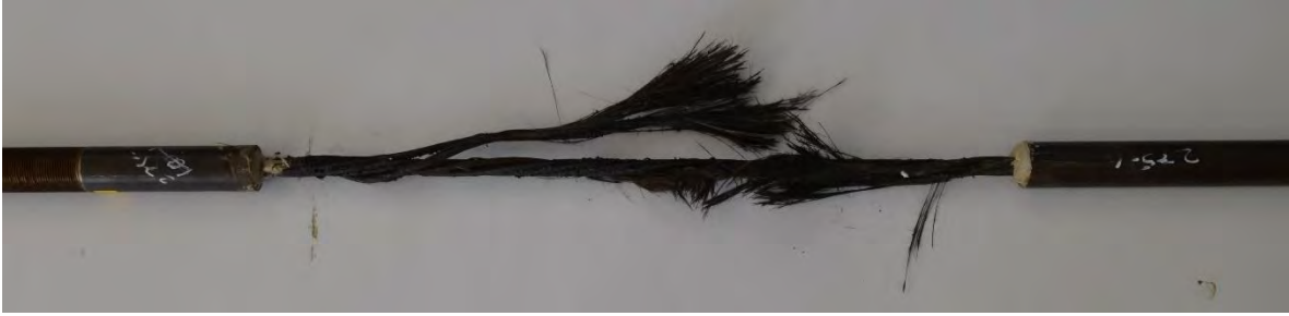
Figure 6.2-8 Failure of CFCC specimen at 527 °F (275 °C)
