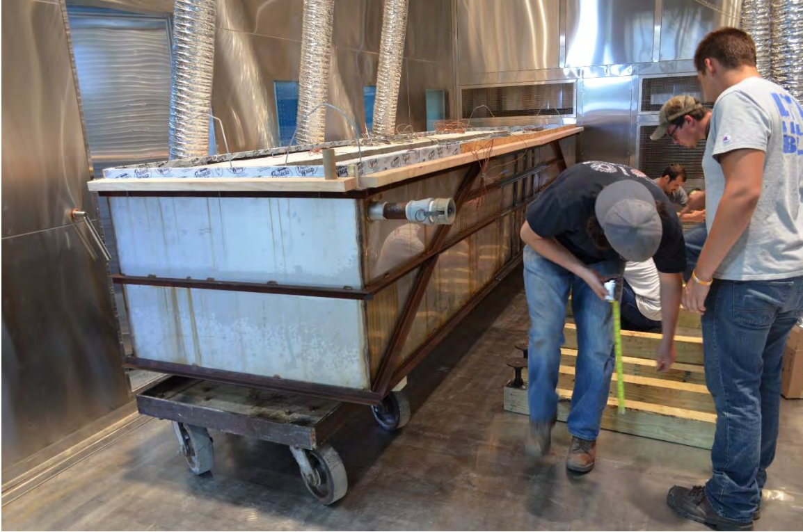
Figure 5.2-2 Building a steel tank for the freeze-thaw test of bulb T beams
