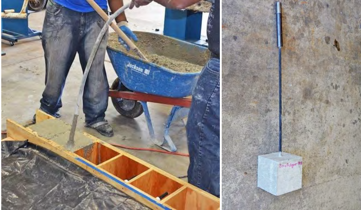
Figure 7.2-4 Pouring concrete and completed pull-out specimen after removal of formwork
