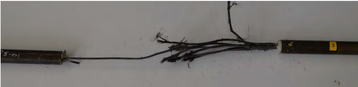
Figure 6.2-4 Failure of CFCC specimen at 347 °F (175 °C)
