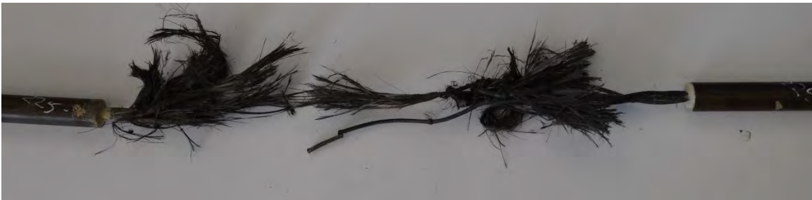
Figure 6.2-6 Failure of CFCC specimen at 437 °F (225 °C)
