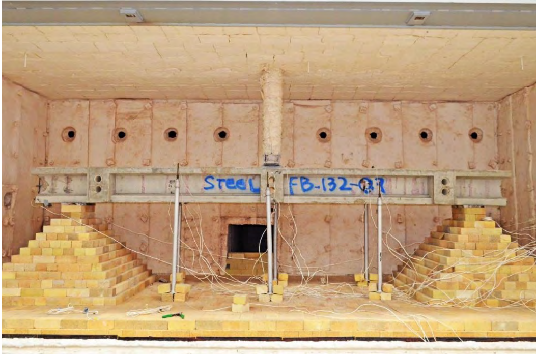
Figure 6.3-9 Beam S132-25-1 before fire
