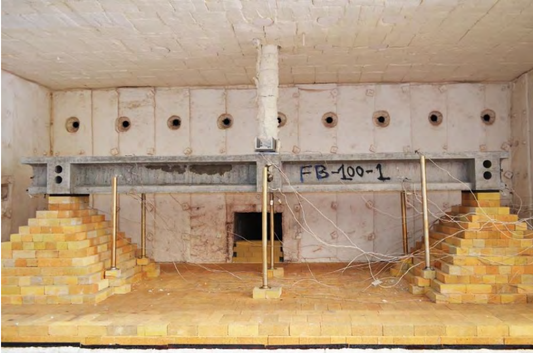
Figure 6.3-24 Beam C100-20-1 before fire
