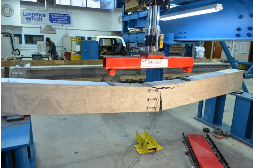
Figure 7.3-13 Failure of B1-0.5
