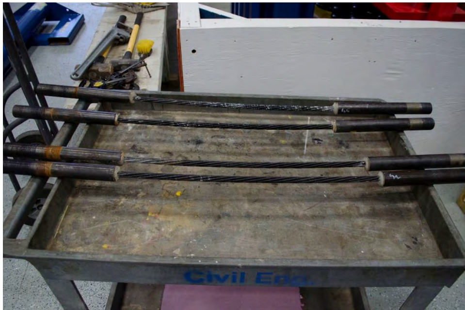
Figure 5.3-8 Preparing CFCC strands for uniaxial tensile test to evaluate residual capacity
