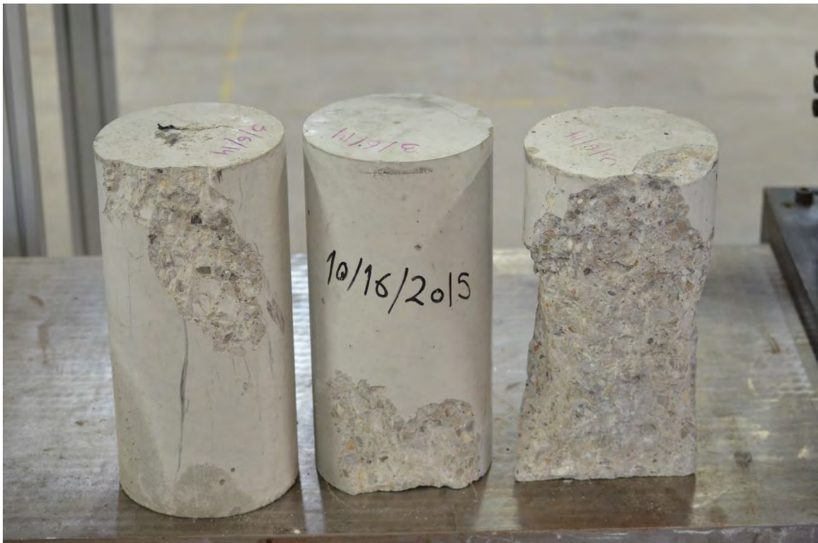
Figure 5.2-14 Typical failure mode of control cylinders not exposed to freeze-thaw cycles
