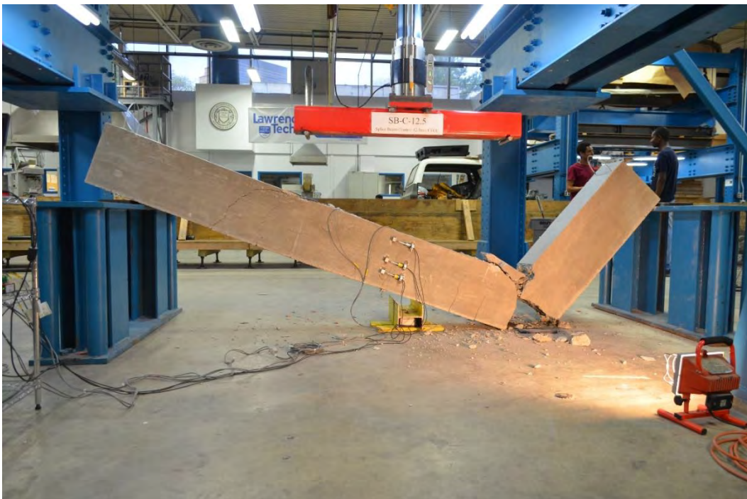
Figure 7.3-10 Failure of BC-0.5
