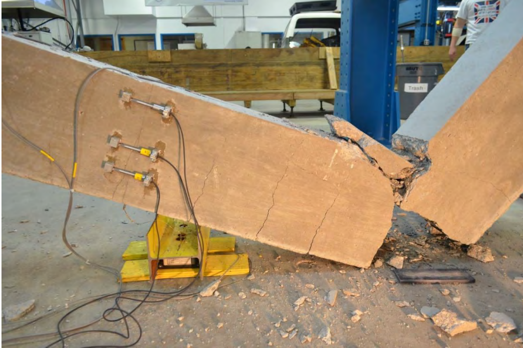
Figure 7.3-11 Close-up view of BC-0.5 showing the rupture of steel strands
