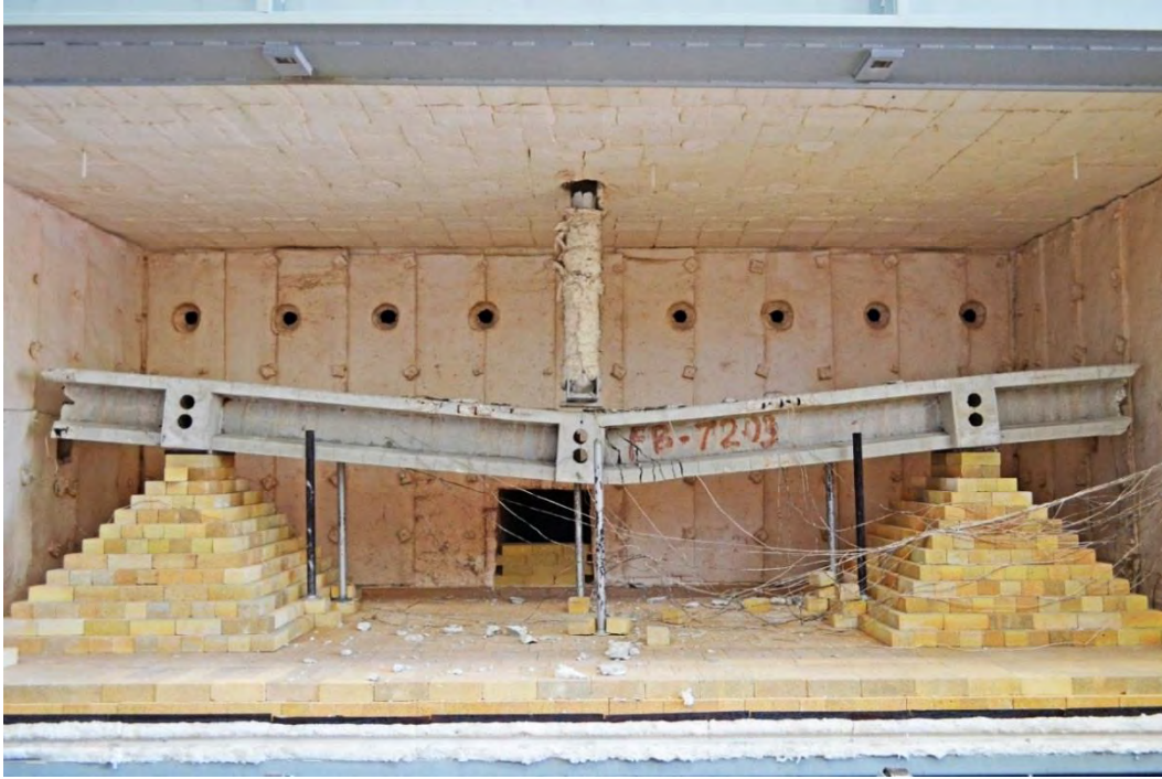
Figure 6.3-19 Beam C72-14-1 after fire
