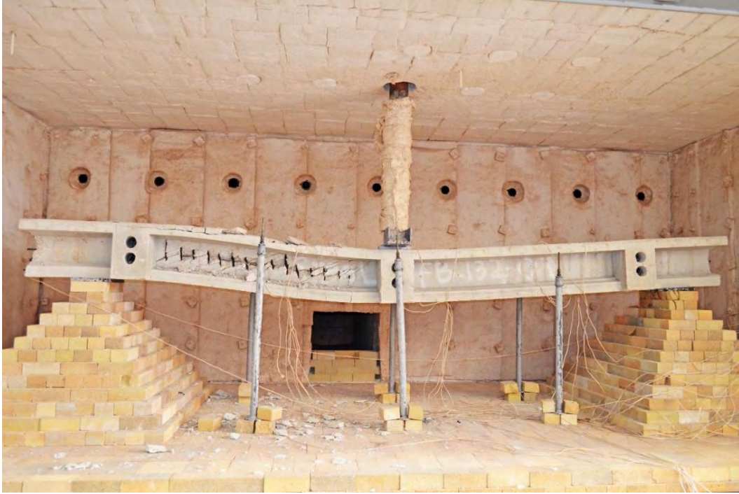
Figure 6.3-11 Beam S132-25-1 after fire
