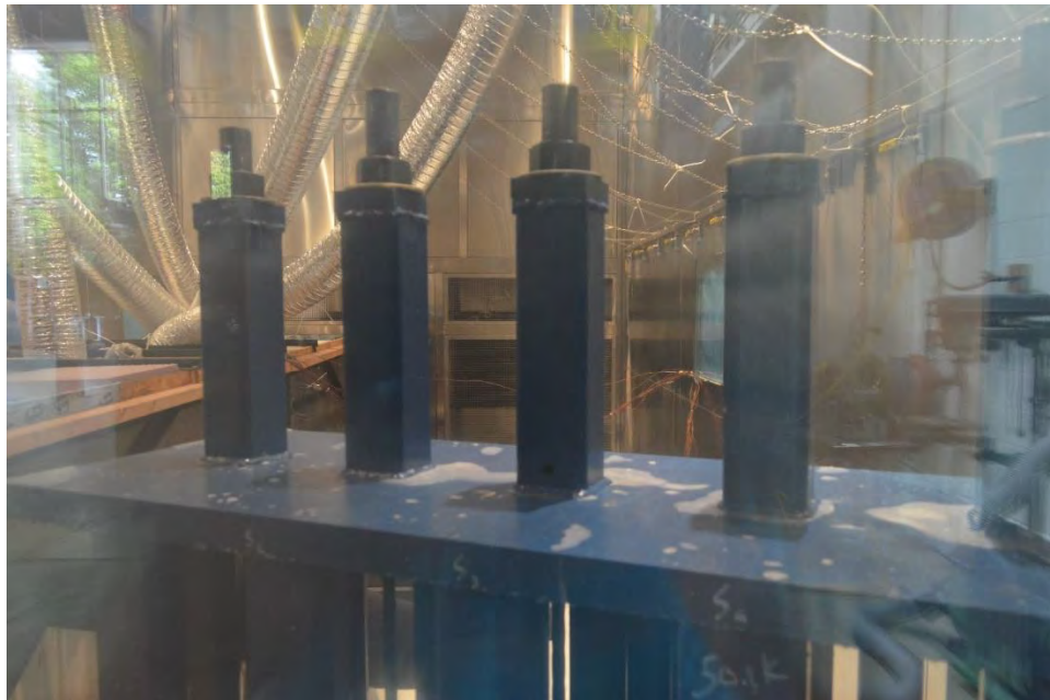
Figure 5.3-4 CFCC specimens during freeze-thaw testing
