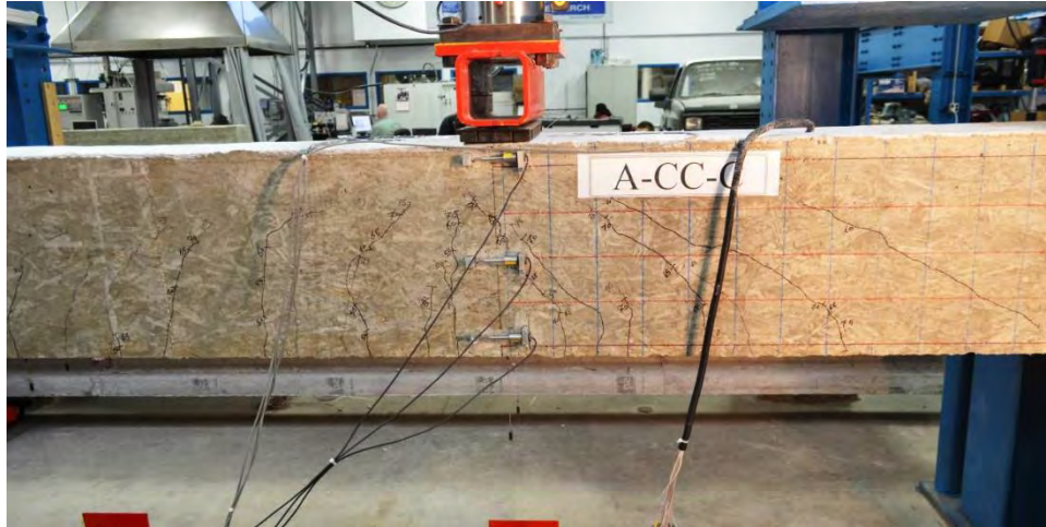
Figure 7.4-18 Crack pattern in beam C-C
