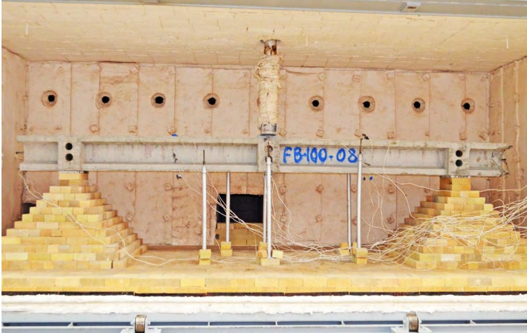
Figure 6.3-48 Beam C100-20-5 before fire
