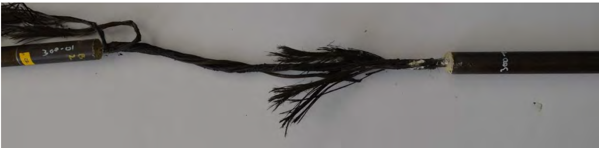
Figure 6.2-9 Failure of CFCC specimen at 572 °F (300 °C)
