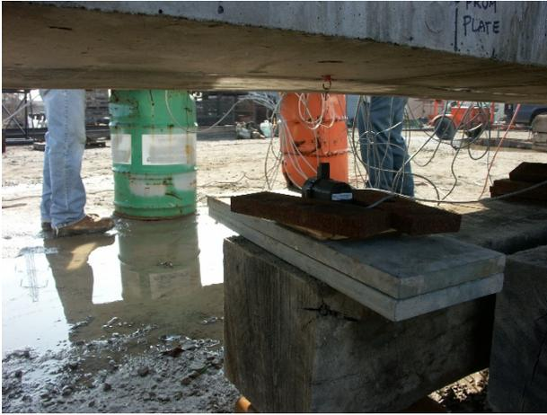
(a) CAPS setup for beam deflection measurement
