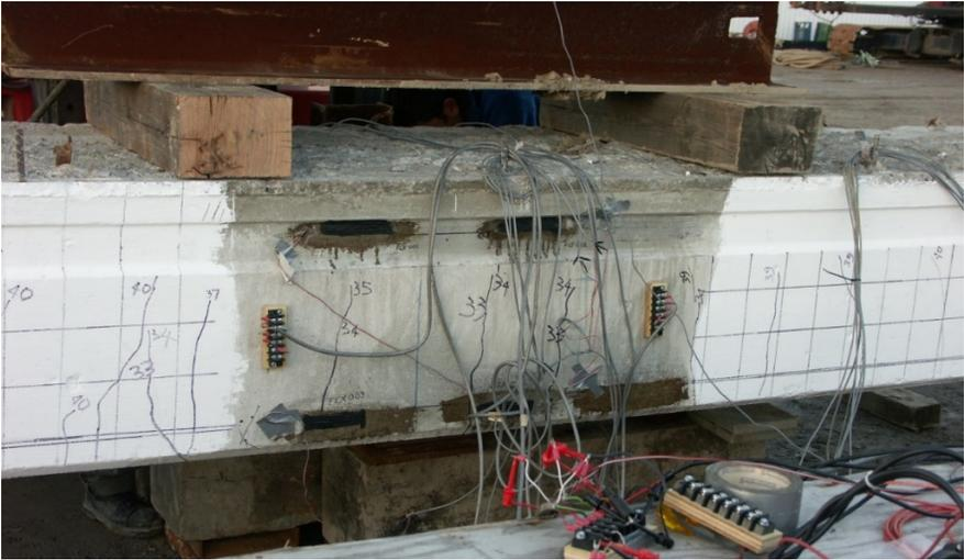
**Figure 2-26. Flexural crack propagation during load testing**
