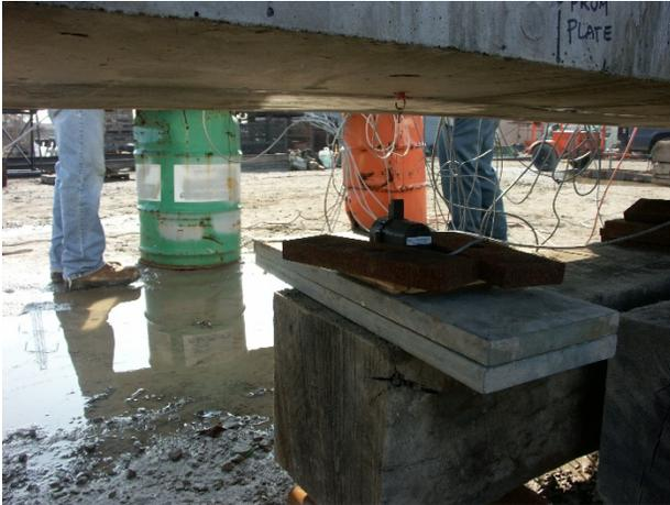
(a) CAPS setup for beam deflection measurement
