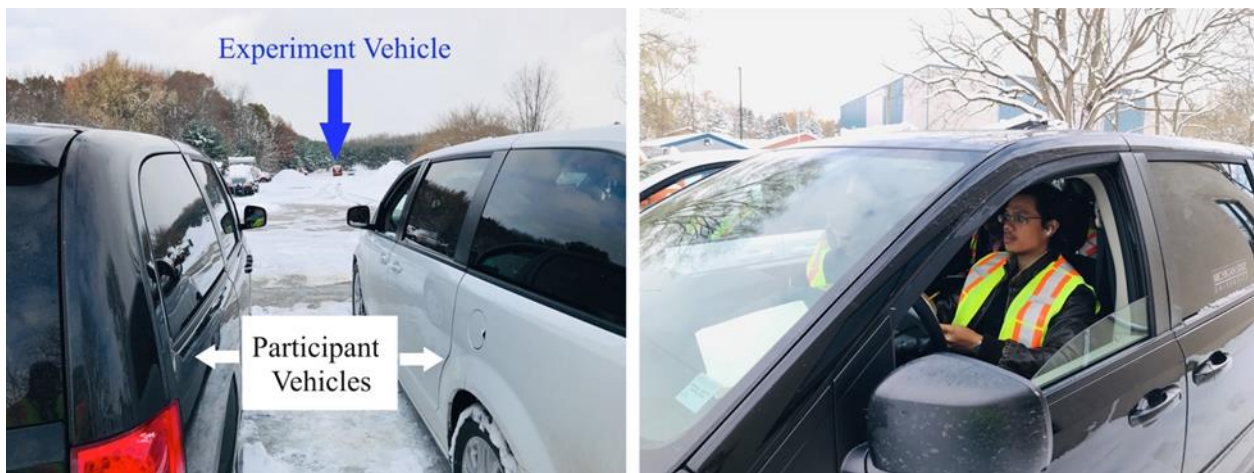
Figure 4-2 Conspicuity test configuration (participants are in stationary vehicles during the test)
