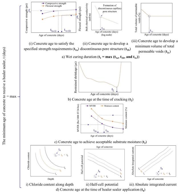
Figure 4-1. The procedure for deciding the minimum concrete age to receive a healer sealer
