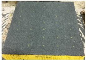
f) Specimen after two coats of epoxy application
