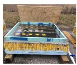
d) Slabs ponded with NaCl solution
