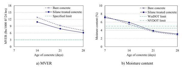
Figure 3-13. MVER and moisture concrete variation with the age of concrete
