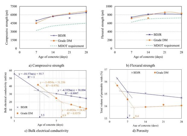
Figure 3-5. Experimental results to determine wet curing duration
