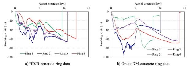
Figure 3-6. Steel ring strain variation with time
