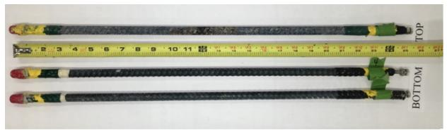
a) Reinforcing steel of a reference specimen
