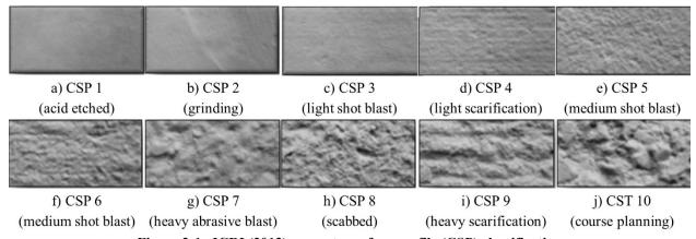
Figure 2-1. ICRI (2013) concrete surface profile (CSP) classification
