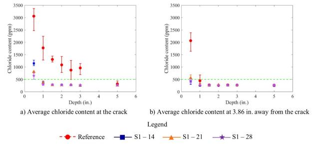
Figure 4-4. Chloride content along the depth of Grade DM concrete specimens Note: ppm = parts per million.
