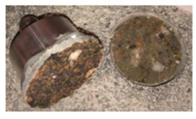
iii) Failure at an elevated temperature
