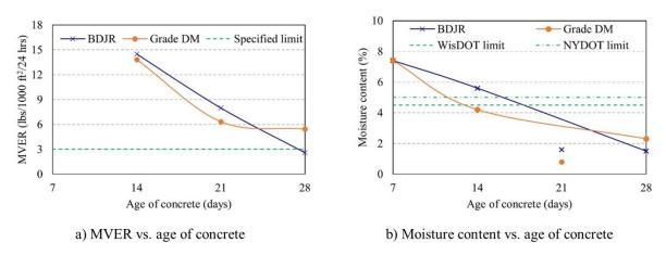
Figure 3-7. MVER and moisture content variation with the age of concrete
