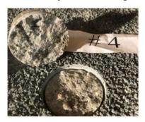
iv) Failure at room temperature following a heat cycle a) Failure modes under simulated laboratory exposure conditions
