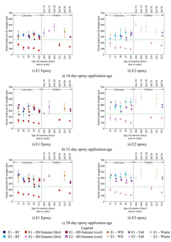
Figure 3-9. Thin epoxy overlay bond strength performance on Grade DM concrete slabs Note: RT = room temperature; HS= elevated temperature; WD = wet-dry cycle.
