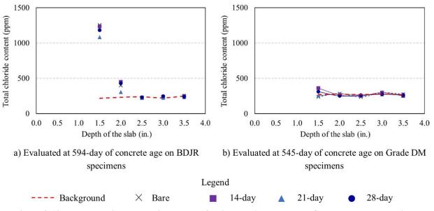
Figure 3-12. Total chloride content in the slabs fabricated with BDJR and Grade DM concrete mixes
