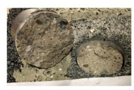
ii) Failure at room temperature following a wet cycle
