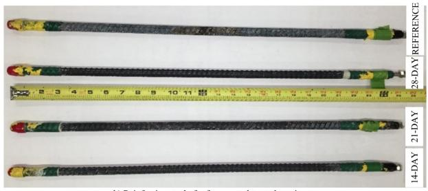
b) Reinforcing steel of reference and treated specimens
