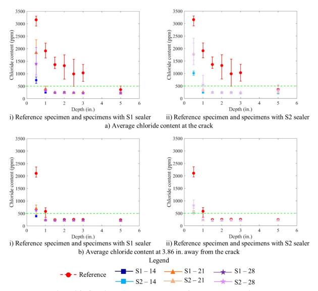
Figure 4-3. Chloride content along the depth of BDJR concrete specimens
