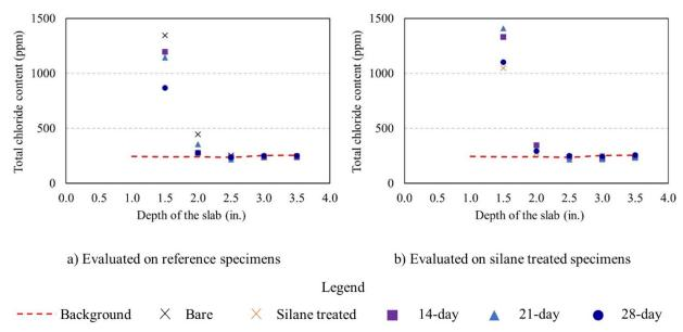
Figure 3-16. Total chloride content along the depth of the slab with and without silane pretreatment
