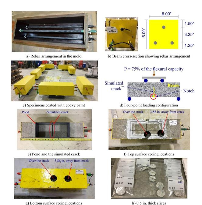
Figure 4-2. Healer sealer performance evaluation – specimen detail and coring locations
