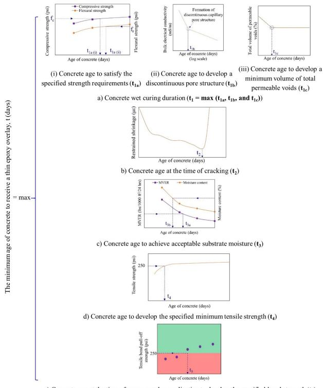
e) Concrete age at the time of epoxy overlay application to develop the specified bond strength  $(t_5)$
