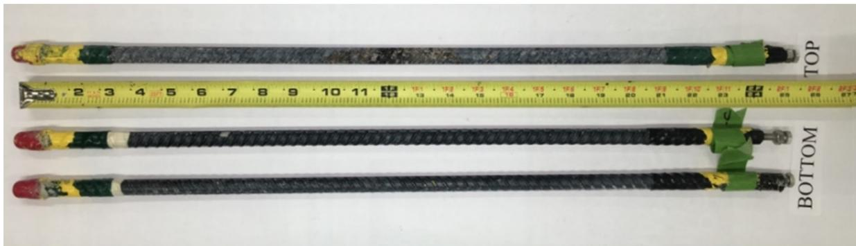
a) Reinforcing steel of a reference specimen
