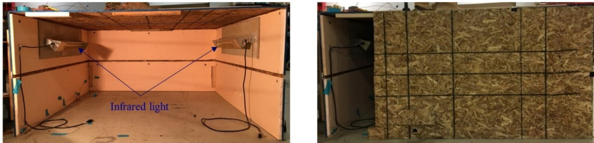
a) Insulated heating chamber with infrared lights
