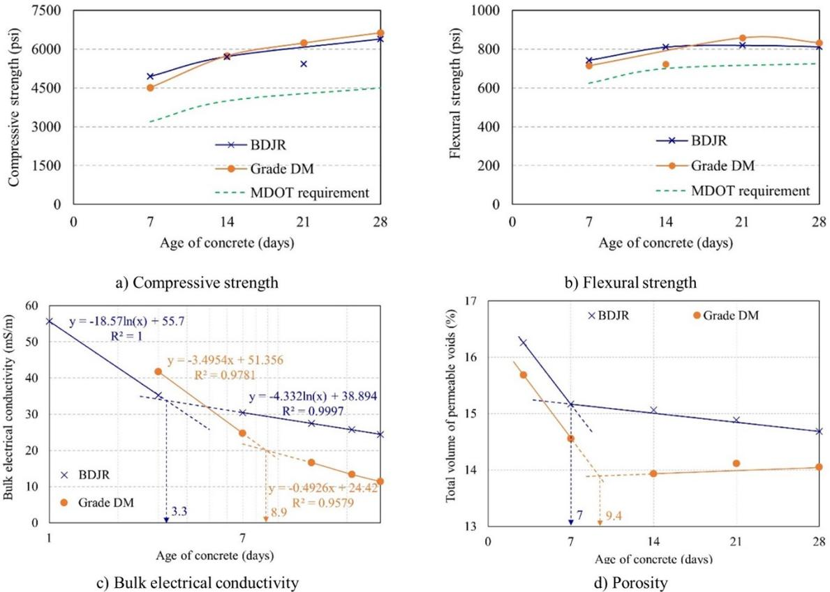
**Figure 3-5. Experimental results to determine wet curing duration**
