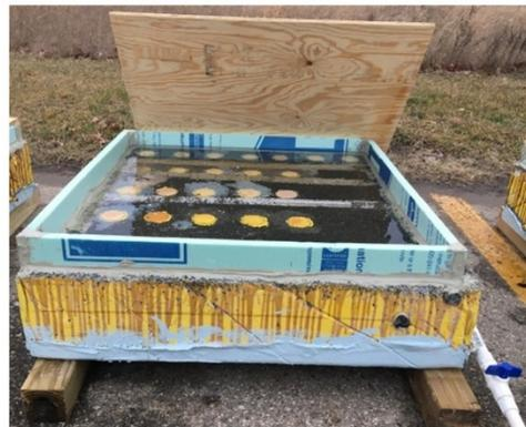
d) Slabs ponded with NaCl solution
