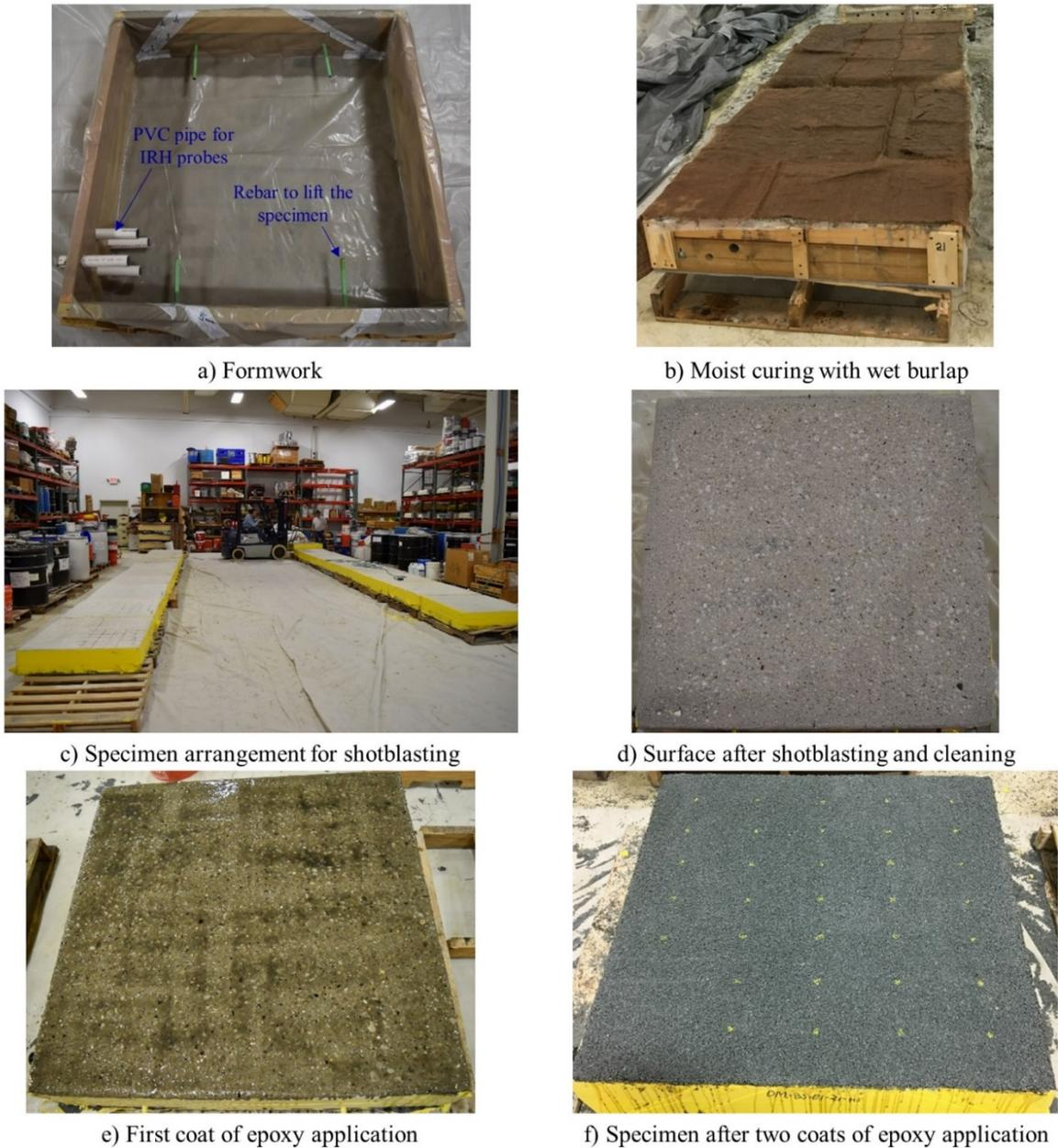
**Figure 3-2. Slab specimen fabrication and preparation procedures**
