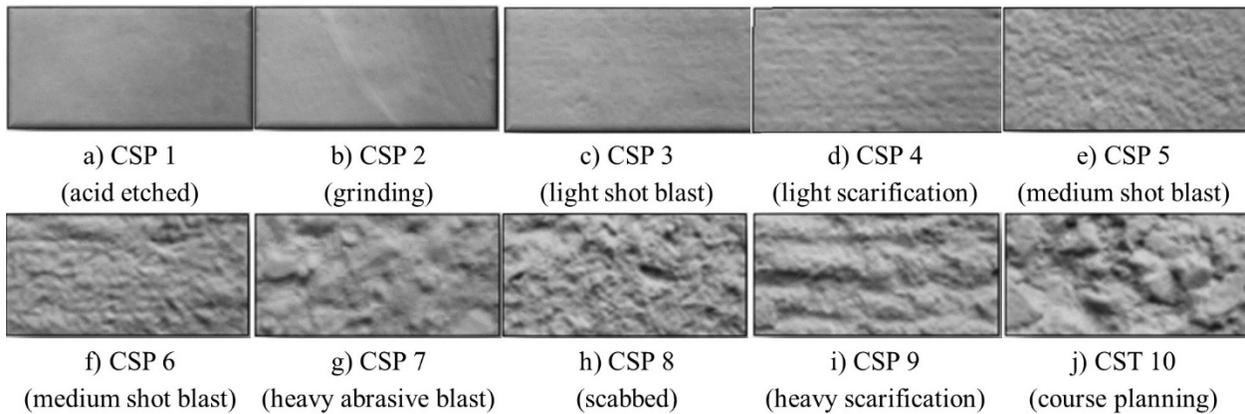
**Figure 2-1. ICRI (2013) concrete surface profile (CSP) classification**
