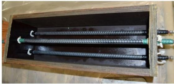
a) Rebar arrangement in the mold
