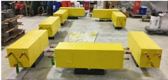
c) Specimens coated with epoxy paint
