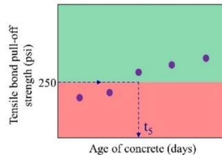
e) Concrete age at the time of epoxy overlay application to develop the specified bond strength ( $t_5$ )
