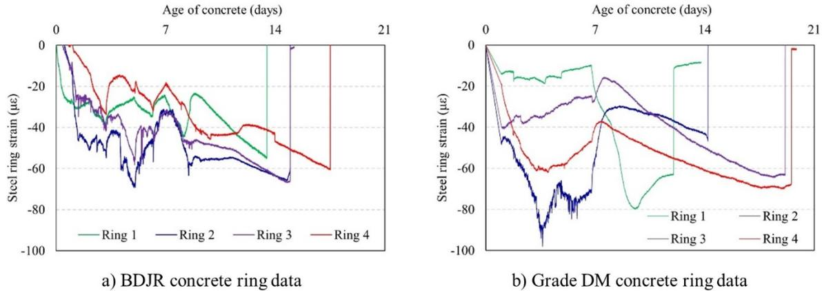
**Figure 3-6. Steel ring strain variation with time**
