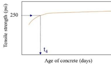
d) Concrete age to develop the specified minimum tensile strength ( $t_4$ )
