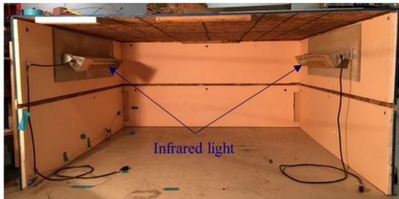
a) Insulated heating chamber with infrared lights
