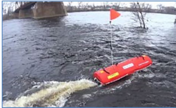
FIGURE 7. MDOT'S BRIDGE INSPECTION ROBOT USES SONAR TO DETECT UNDERWATER CHANNEL SCOUR AROUND BRIDGE PILINGS
