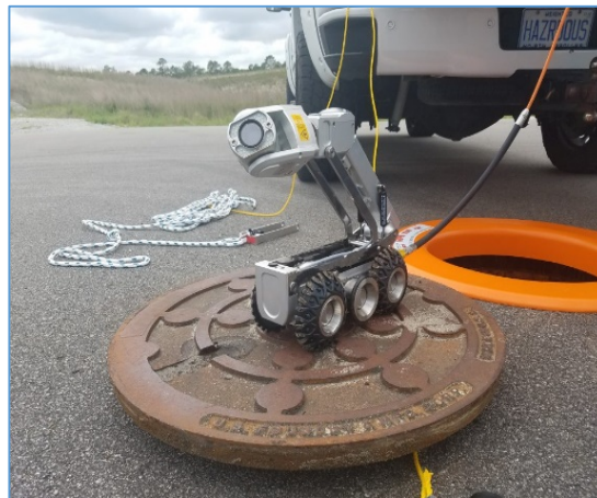
FIGURE 1. A TETHERED MOBILE ROBOT USED FOR INSPECTION OF DRAINAGE SYSTEMS
