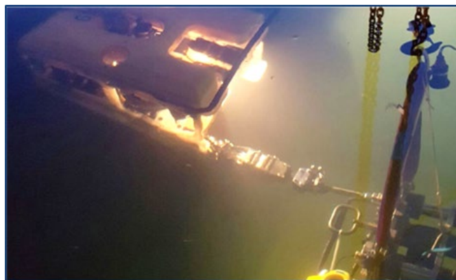
FIGURE 6. AN UNDERWATER ROV WITH CUSTOM-FITTED TOOLS CAN PERFORM SOME CONSTRUCTION TASKS
