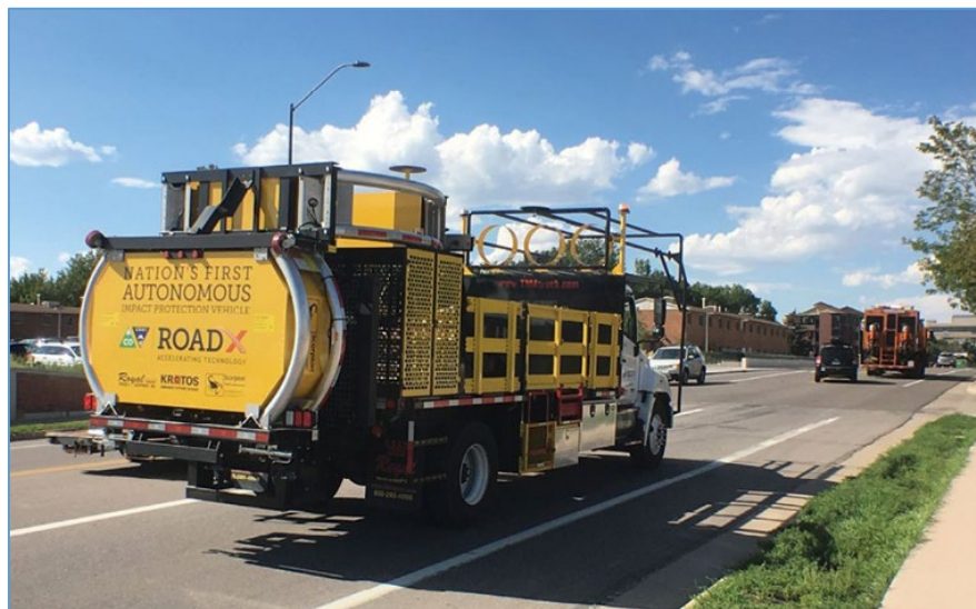
FIGURE 2. AUTONOMOUS ATTENUATOR TRUCKS CAN REDUCE RISKS TO ROAD CREWS
