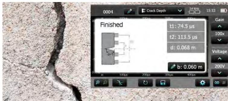
**Figure 2-49. Crack depth calculation using Proceq Pundit PL-200 data (Proceq 2014)**
