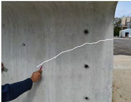
(c) Diagonal cracking – From girder top to girder bottom
